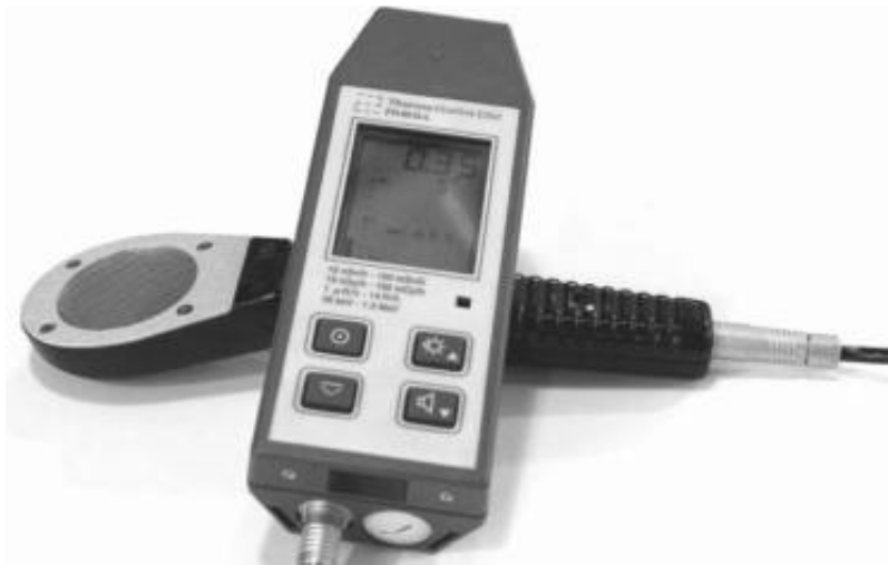
Figure 3.35 Thermo Eberline ESM FH 40 G-L radiation monitor detects alpha, beta, and gamma radiation.
