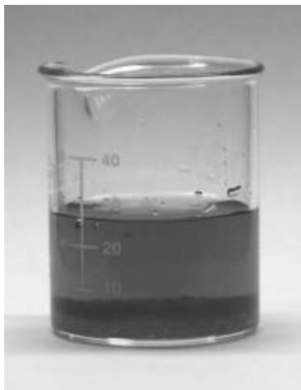
Figure 1.5 Saturated solution of copper sulfate. Copper sulfate crystals dissolve the solid into the liquid while stirring. When the liquid becomes saturated, it can accept no more copper sulfate. Adding more solid only causes the excess crystals to settle to the bottom of the container. The addition of more water would allow the excess crystals to dissolve and become mobile.
