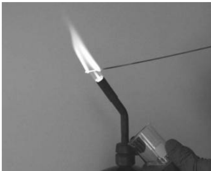
Figure 3.10 Chlorinated solvents are detected with a copper wire in the flame when vapors are drawn into the torch air intake. Low vapor pressure liquids may need to be heated slightly to increase vapor production.
