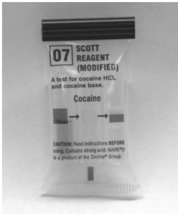
Figure 3.11 An example of a field cocaine test kit. This test uses cobalt thiocyanate to detect cocaine in acidic and basic environment.
