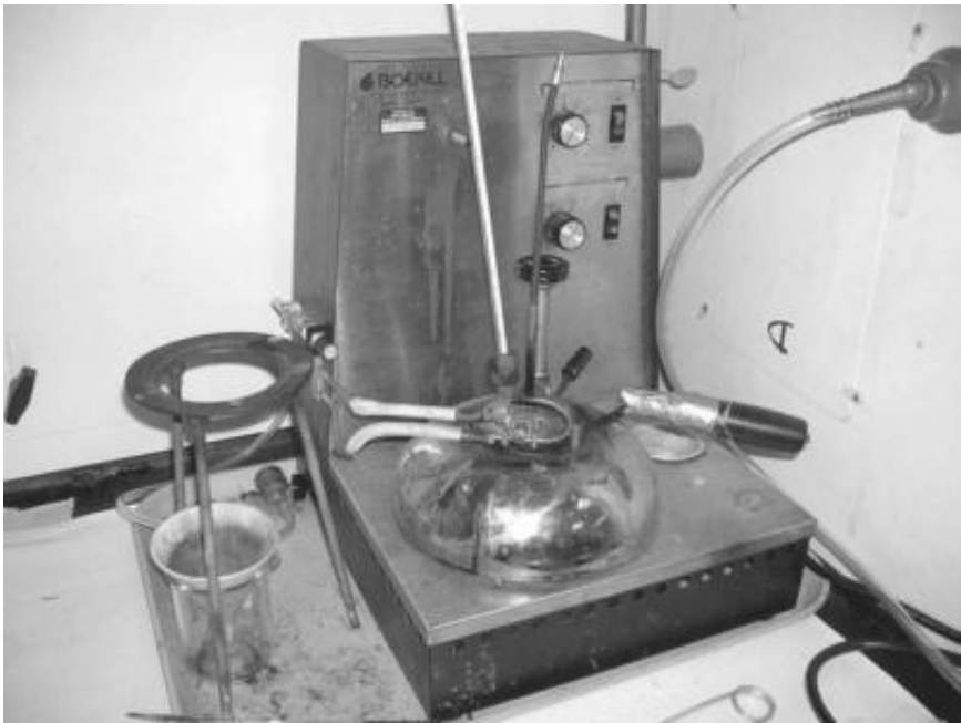
Figure 1.14 This device is used for determination of flash point using the Pensky-Martens closed-cup method.
