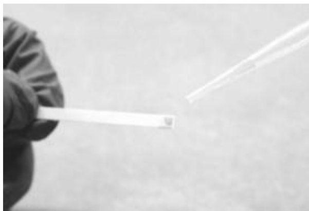
Figure 3.6 Positive result on peroxide test paper from exposure to 3% hydrogen peroxide.
