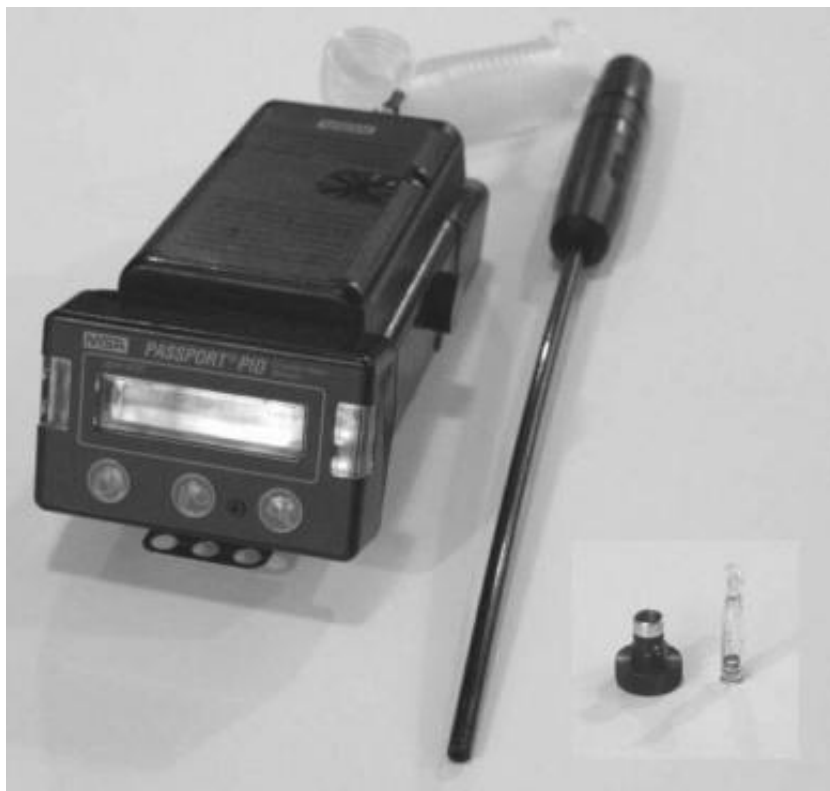
Figure 3.26 The Passport® PID Organic Vapor Monitor photoionization detector from MSA. This unit is shown with the sampling probe attached. The photoionization lamp and cap are pictured on the right.
