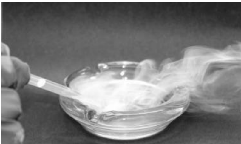
Figure 2.3 Thionyl-chloride-forming acidic fume in moist air.
