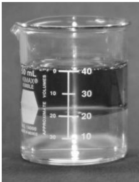
Figure 1.4 Insoluble oil floating on water. Insoluble materials separate after agitation and cannot be diluted.
