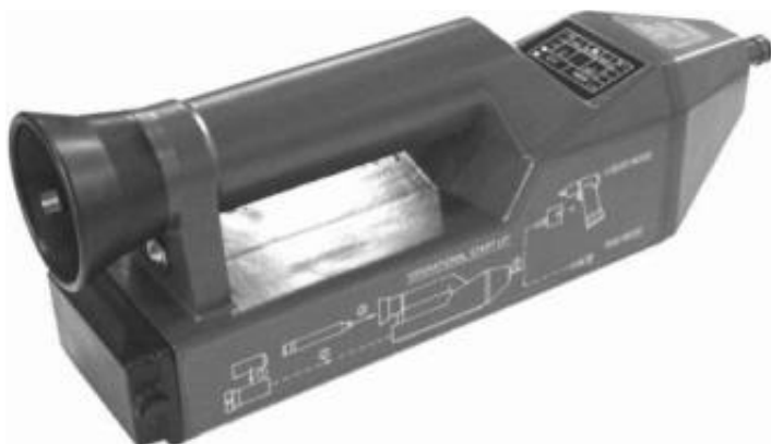
Figure 3.29 AP2C flame photometry air monitor by Proengin SA. The instrument is alarming for G-nerve agent after exposure to a training surrogate.
