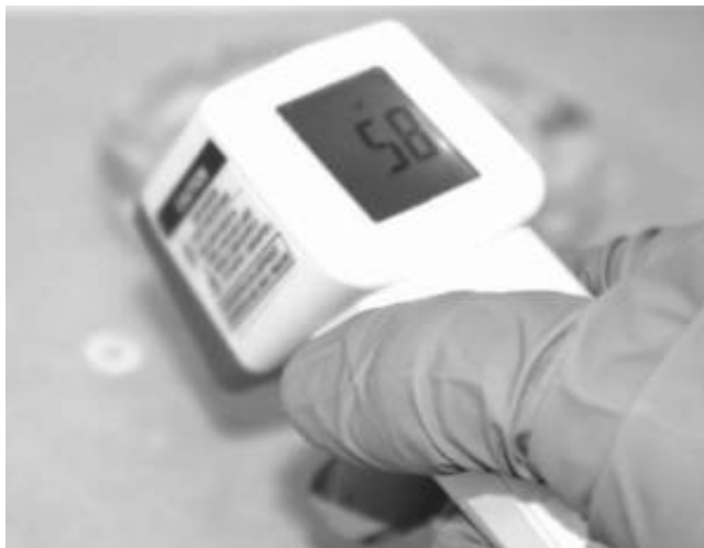
Figure 4.8 Use an infrared thermometer to measure changes in temperature relative to ambient conditions.
