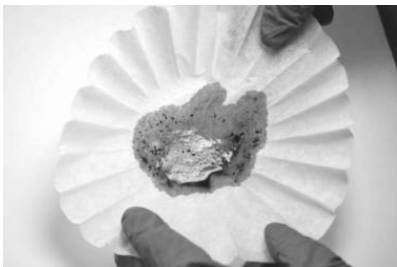
Figure 3.40 Filtering may be useful to concentrate a powder for testing. Here a dilute povidone solution is poured or sprayed over flour on the filter.
