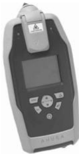
Figure 3.34 The FirstDefender from Ahura Corporation uses Raman spectroscopy to identify unknown substances. (Image: Ahura Corporation, Wilmington, MA. With permission.)
