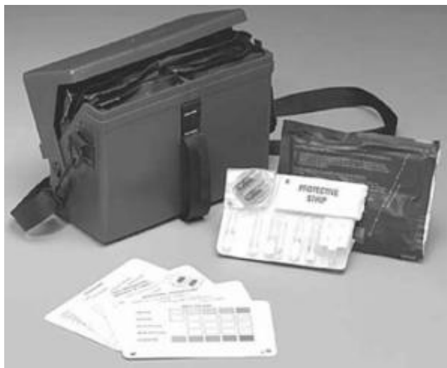
Figure 3.12 The M256A1 Kit includes instructions, M8 paper, and several vapor samplers to detect and identify chemical warfare agents as vapors in air.
