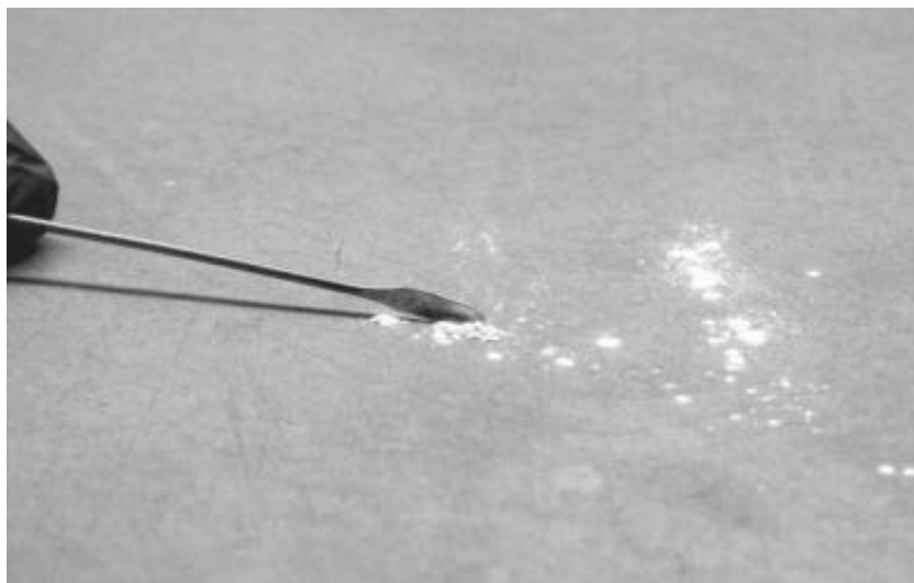
Figure 3.37 Split the sample so that the entire volume is not consumed in testing. Preserve some of the material for future testing and some as possible evidence. If testing cannot be performed on a very small amount, you should re-evaluate your characterization strategy.
