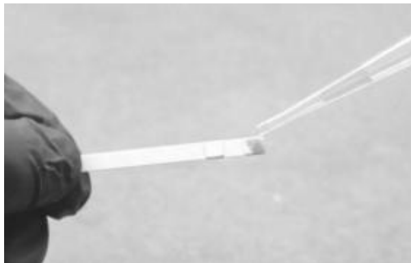
Figure 3.7 Detection of nitrate in an aqueous solution by a nitrate/nitrite test strip.
