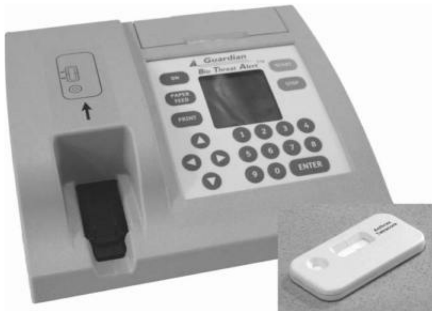
Figure 3.49 The Guardian Bio Threat Alert, a handheld immunochromatography test with optical reader.
