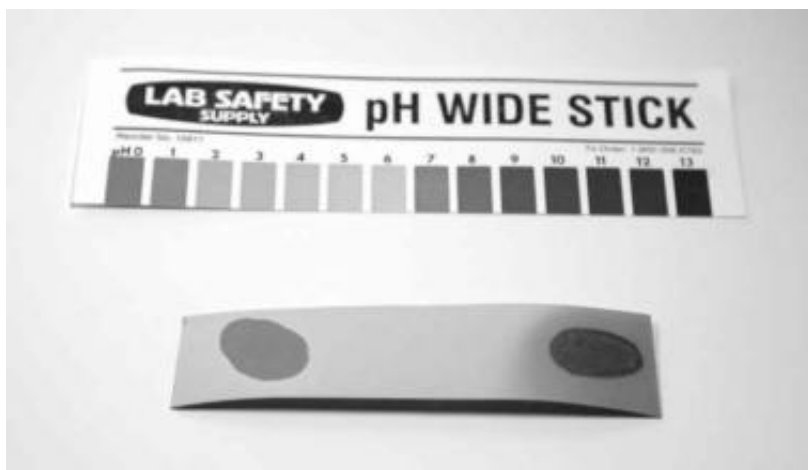
Figure 3.3 A universal pH indicator on a test strip indicating a strongly acidic pH on the left and a strongly basic pH on the right. pH indicators may be used to detect corrosive or caustic vapors as indicated by the “fog” of activated indicator surrounding the liquid ammonium hydroxide on the right.
