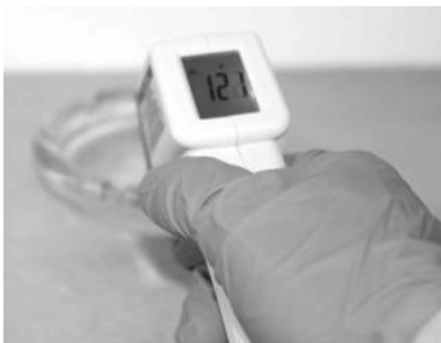
Figure 2.4 Infrared thermometer measuring increase in temperature caused by addition of sodium hydroxide to water.
