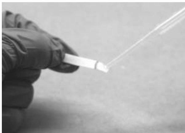
Figure 3.5 Black color bleached immediately to white on a potassium iodide starch test strip. Note the thin line of black formed at the leading edge of solution moving along the test strip.
