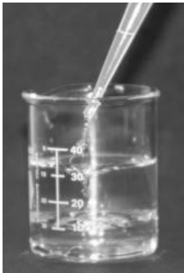
Figure 1.9 Trichloroethylene (TCE) under water. TCE is insoluble in water and even after agitation will separate and fall below the water to form a distinct layer.
