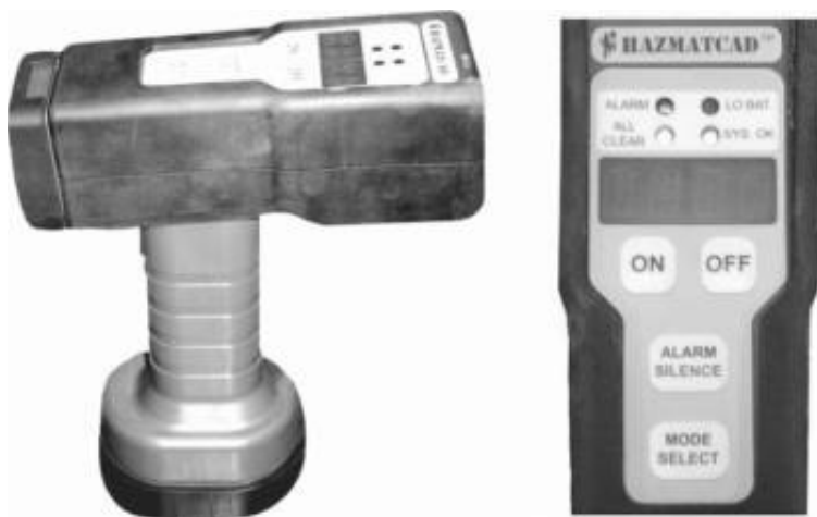
Figure 3.27 HAZMATCAD surface acoustic wave detector by MSA. HAZMATCAD incorporates electrochemical cells to expand its capability.
