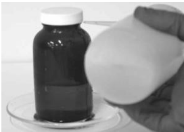
Figure 4.4 Peroxide material dried between the cap and container can shear and explode when the lid is removed. A small volume of acetone and water gently applied under the container lid will dissolve exposed solid material. The rinse solution can then be tested for peroxide.
