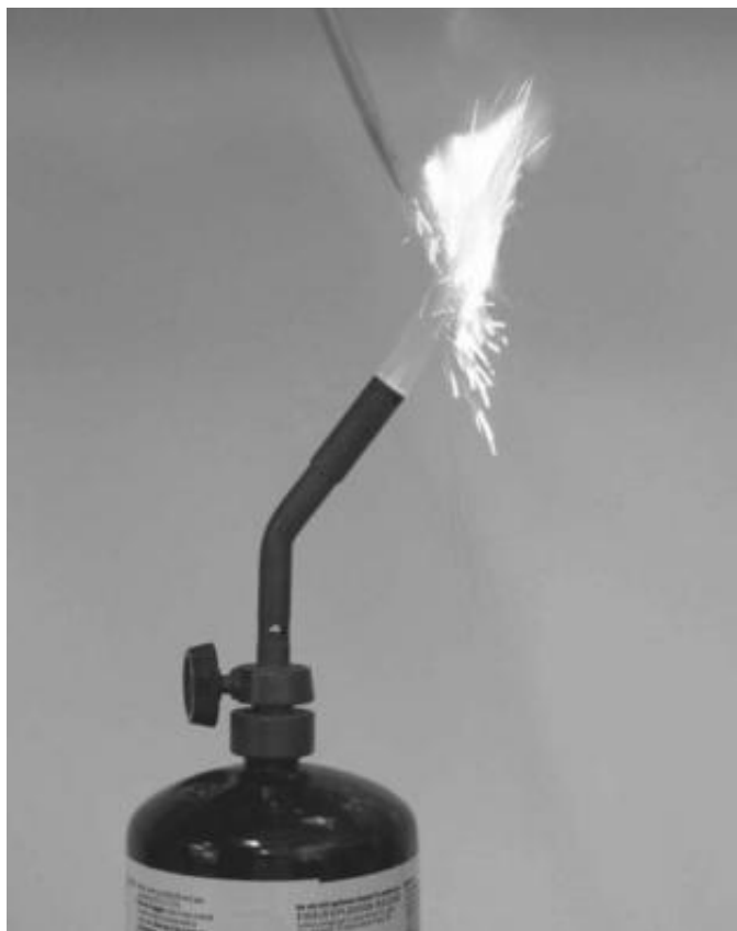
Figure 4.10 Metal dust forming sparks in a propane torch flame.
