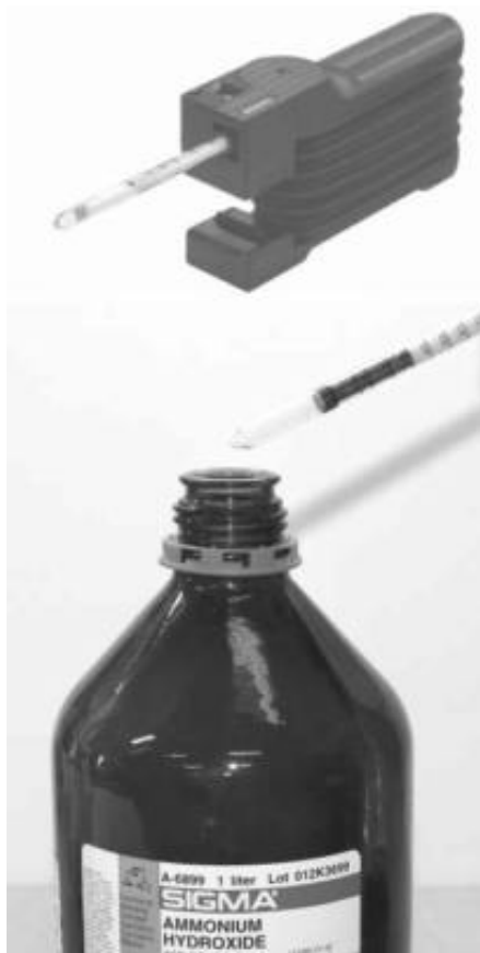
Figure 3.14 Colorimetric tube in the hand-held Drager Accuro® pump (top). Drager ammonia tube detecting ammonium hydroxide vapor (bottom). Colorimetric tubes may be used qualitatively with a bulb syringe or other inexpensive pump.
