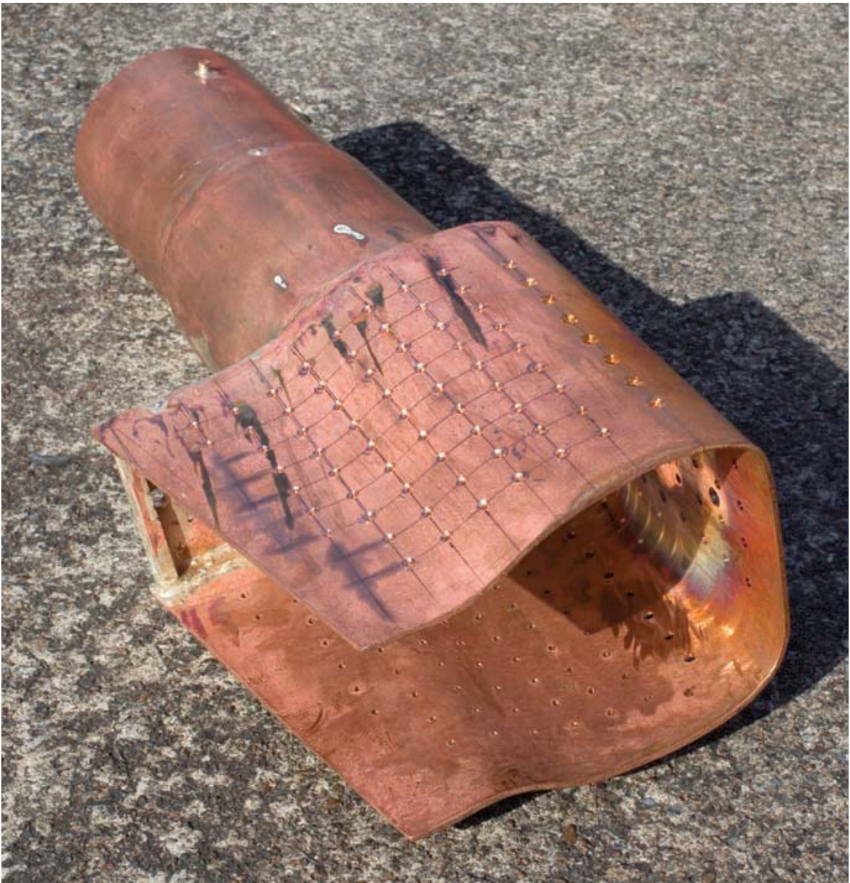
Photo 55 Model locomotive boiler, firebox, copper fabrication.
