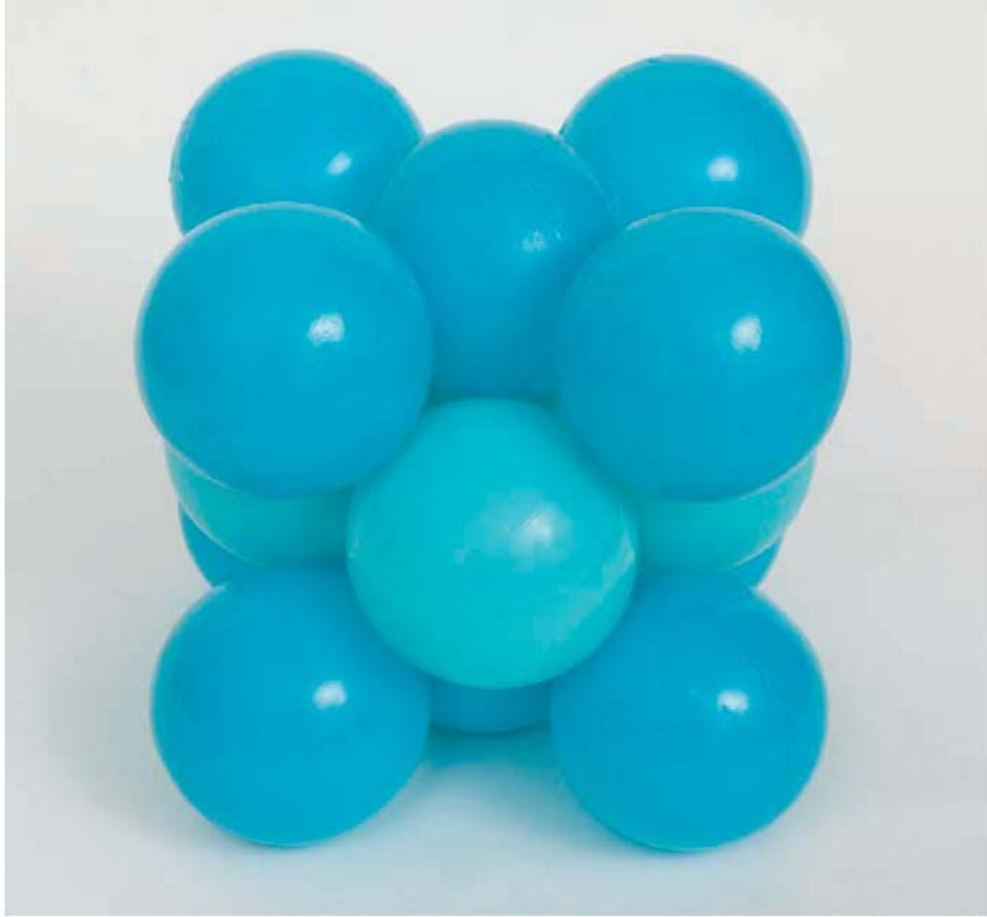
Photo 97 Model of fcc (face centred cubic) atomic structure.
