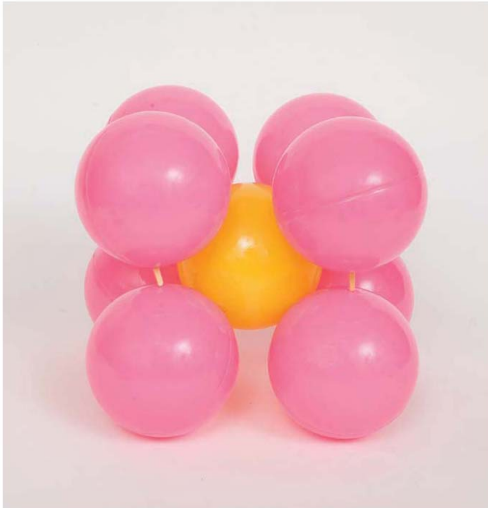
Photo 96 Model of bcc (body centred cubic) atomic structure.
