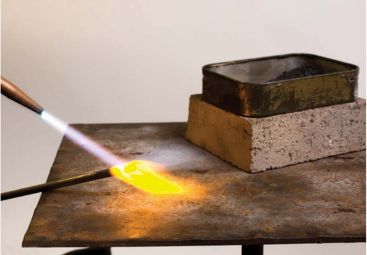
Photo 133 Re-heating test bar after dipping in case hardening compound.
