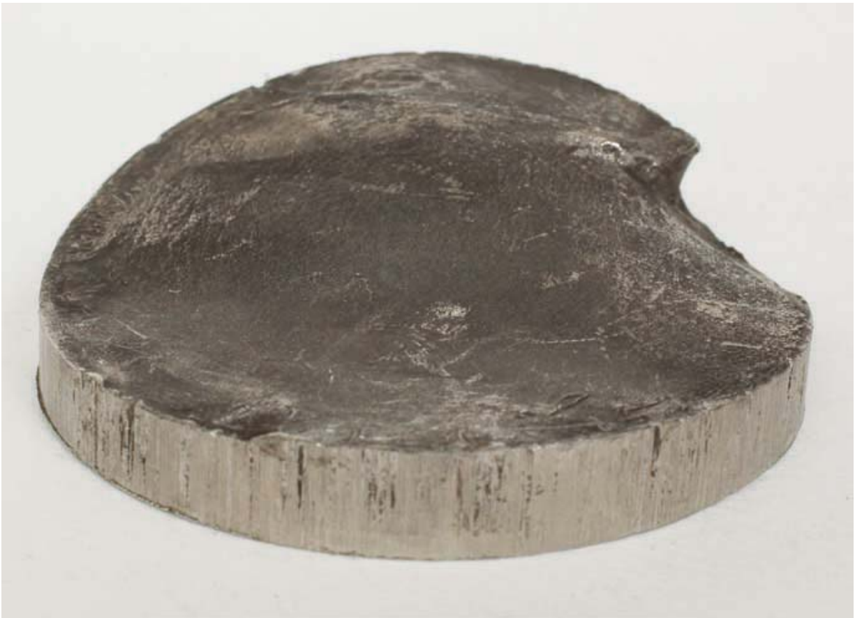
Photo 76 Pump shaft, 85mm dia. rotating bending fatigue failure.
