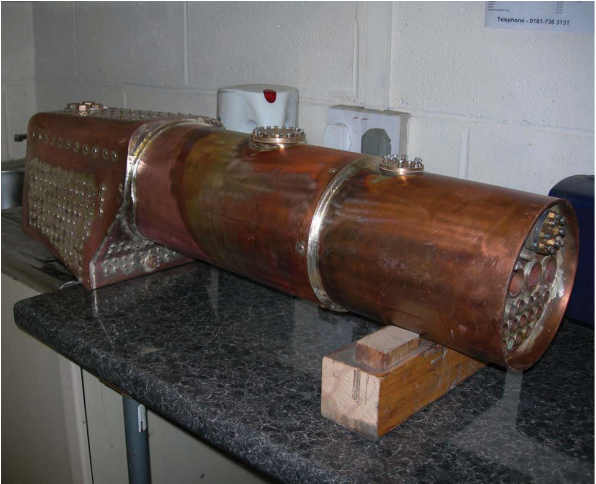
Photo 16 LMS Duchess, showing varieties of silver soldered joints.
