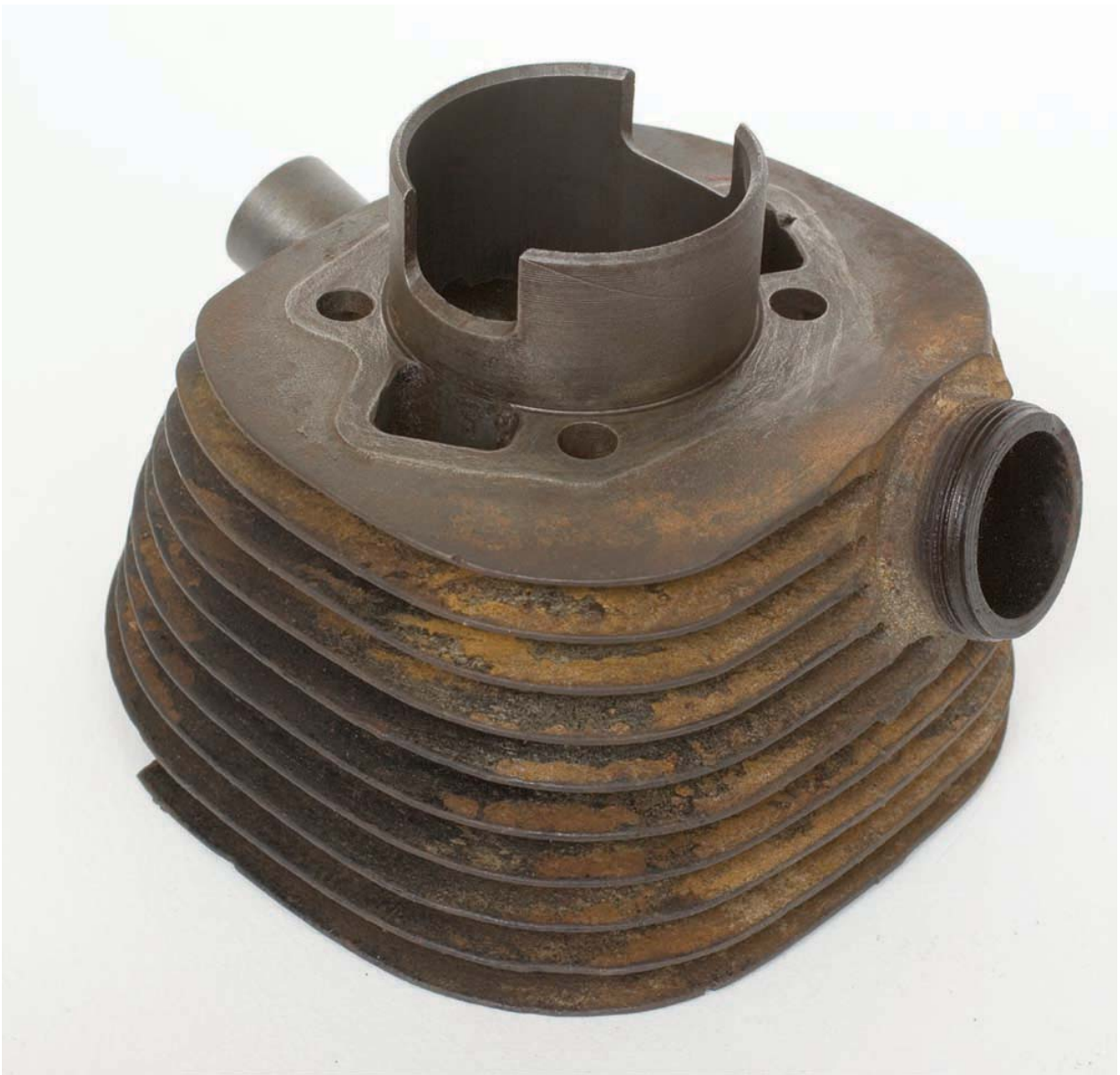
Photo 36 Cylinder, showing large transfer and exhaust ports, produced by coring and requiring only minimal fettling.
