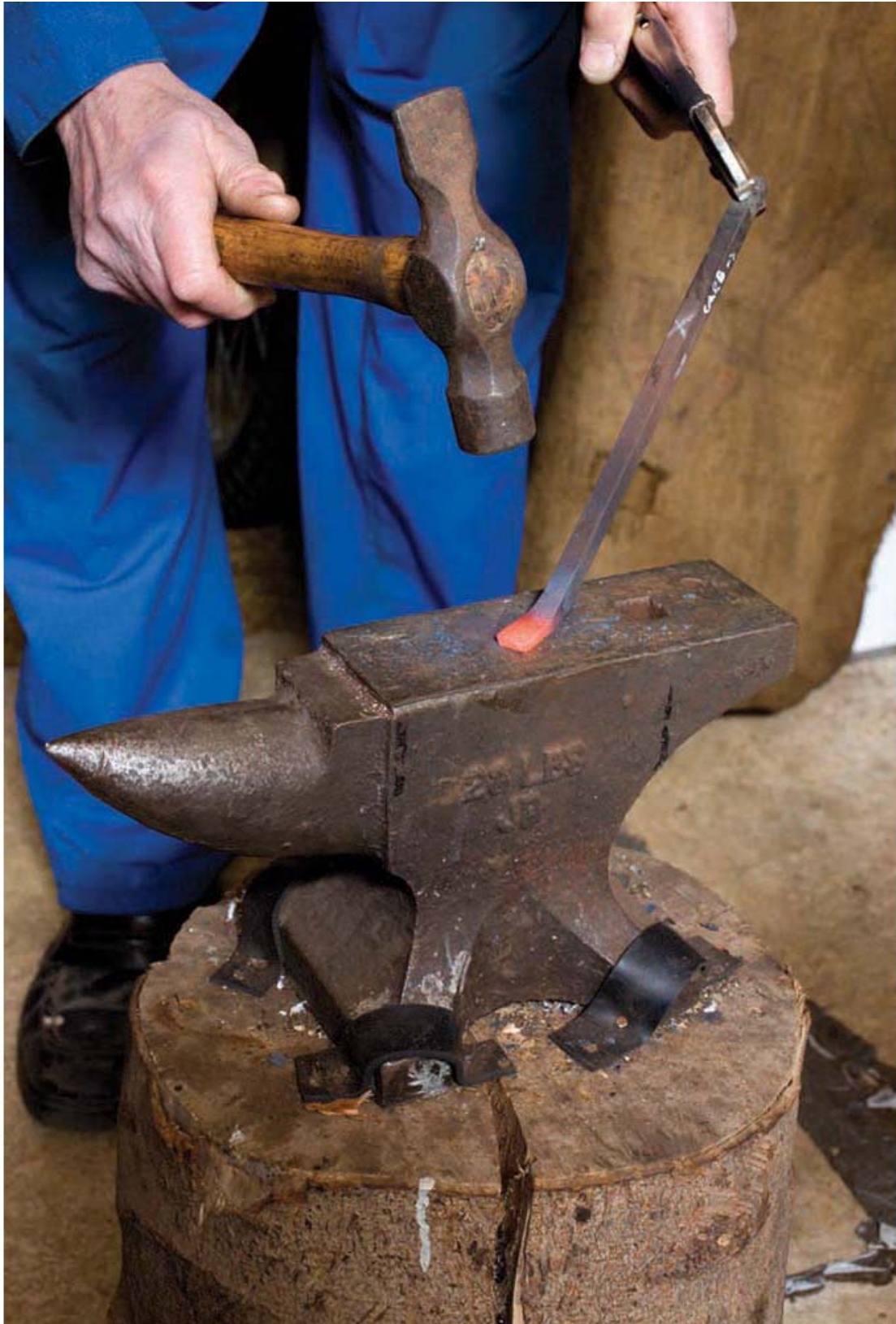
Photo 46 Hot working steel, aka blacksmithing.
