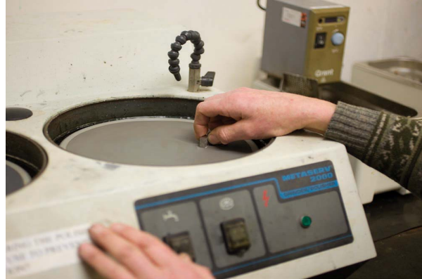
Photo 90 Water lubricated abrasive grinding disc for initial specimen preparation.
