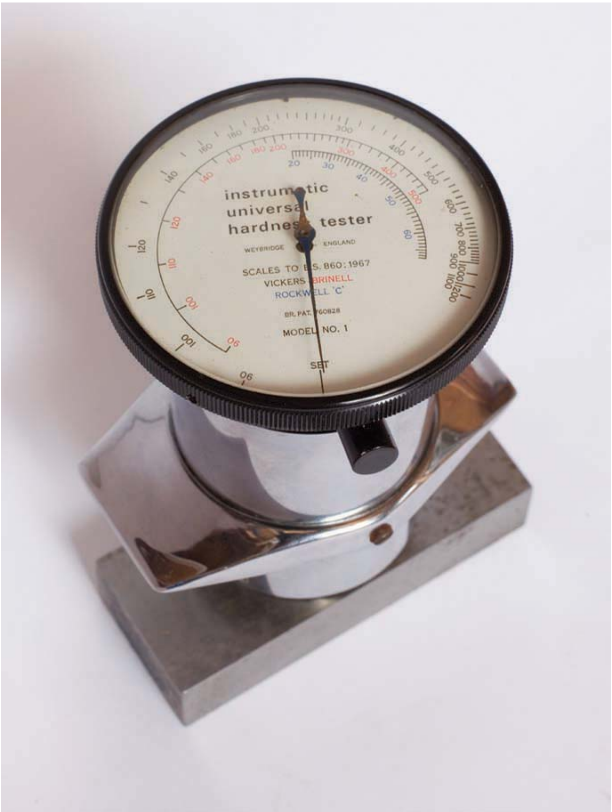
Photo 141 Hand-held mechanical hardness tester with multi-scale reading, for approximate hardness measurement.
