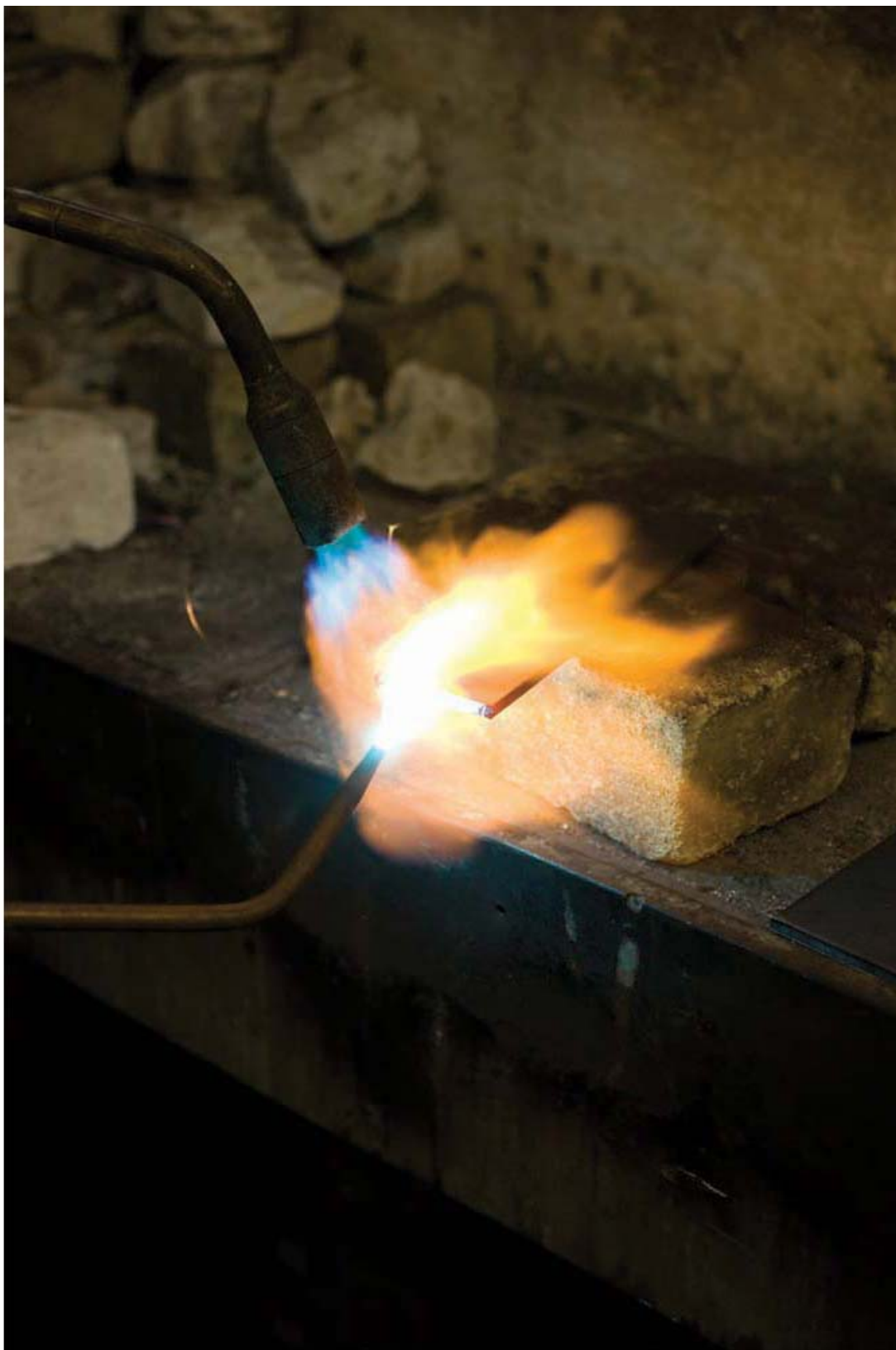
Photo 119 Direct heating by gas torch on firebricks.
