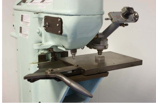
Photo 94 Detail of Vickers hardness tester, traversing table moved to measurement position.
