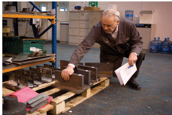
Photo 91 Commercial test house specimens for weld procedure testing.
