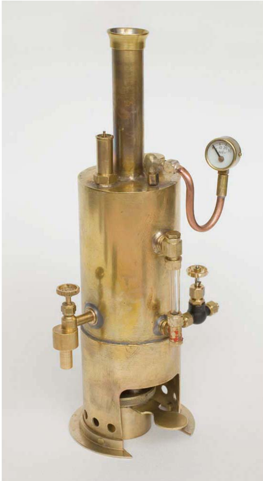
Photo 2 Vertical boiler, delivering 30psi, to power a Viper Vee twin, oscillator steam engine.
