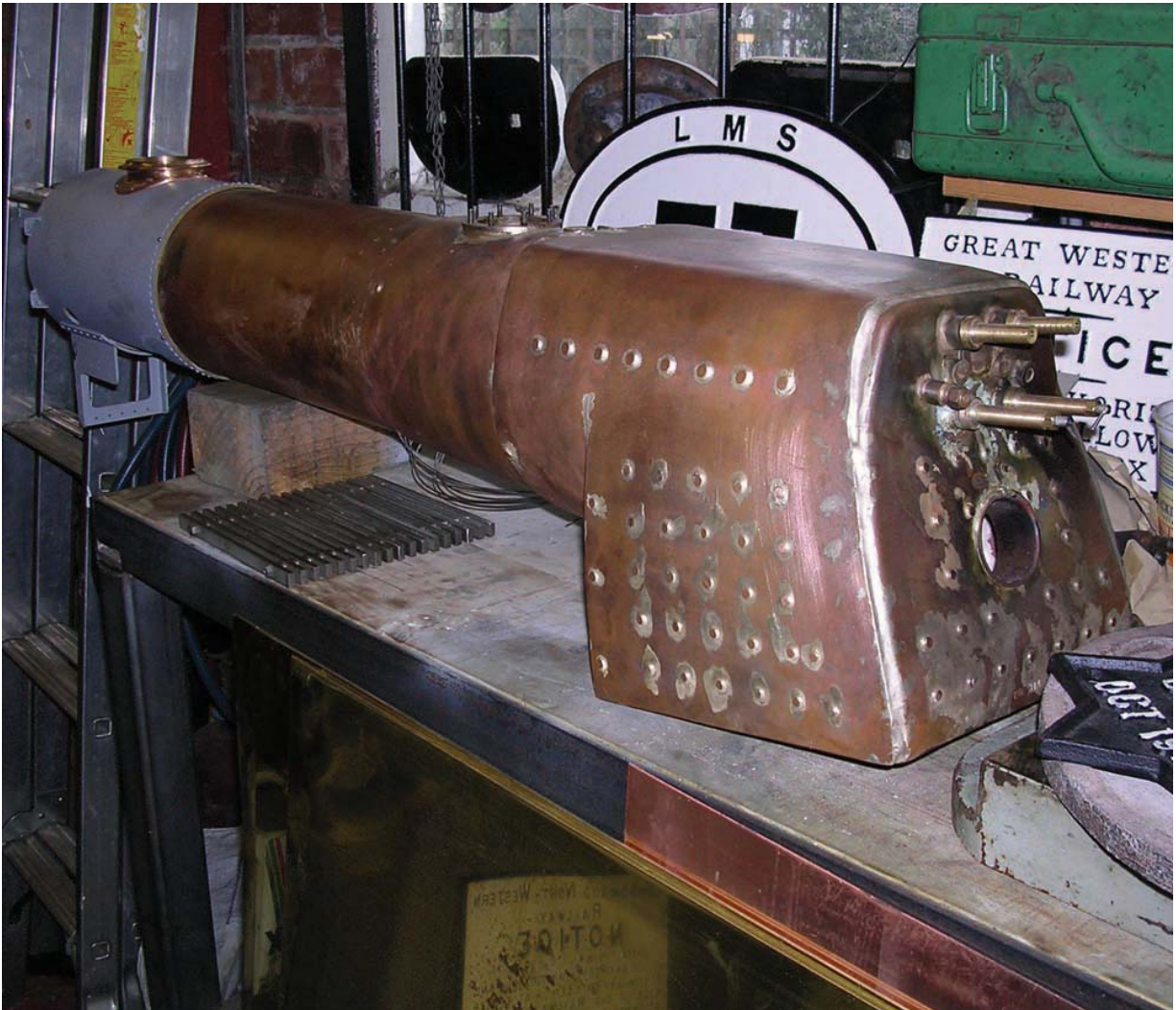
Photo 15 Firebox view of Photo 14, showing reinforcement universally employed.
