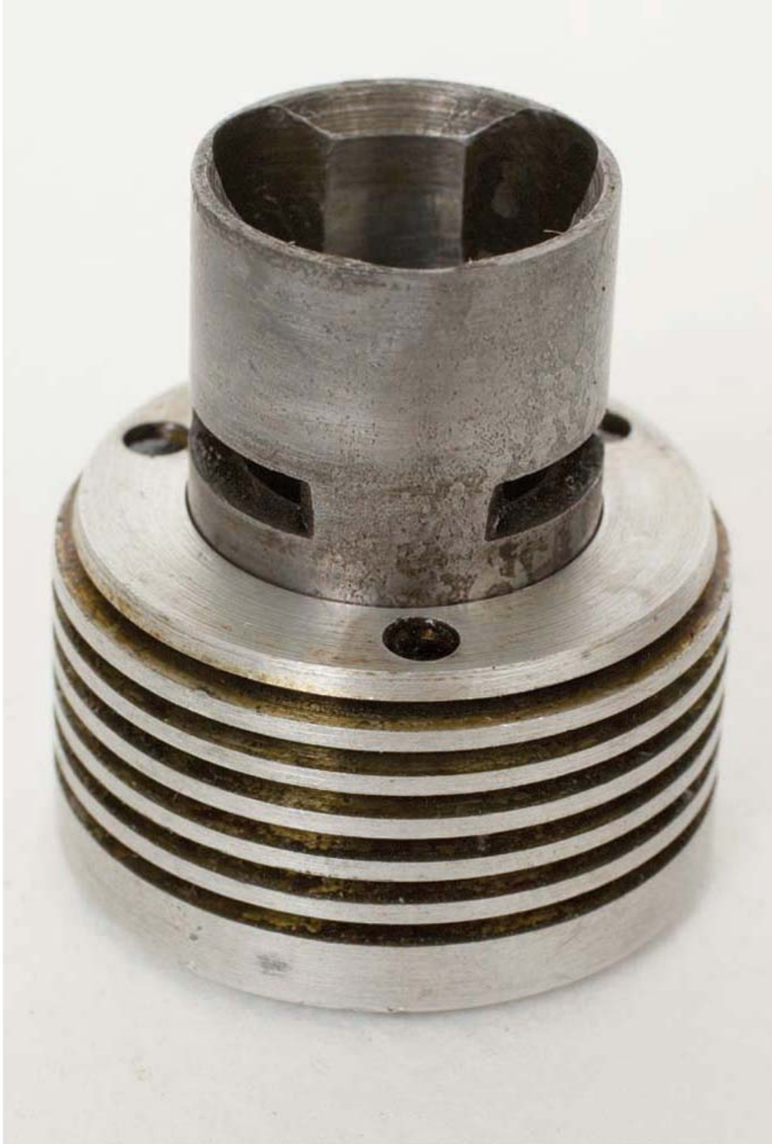
Photo 27 Steel cylinder liner and finned aluminium alloy jacket, transfer ports as grooves in liner, exhaust ports clearly seen.
