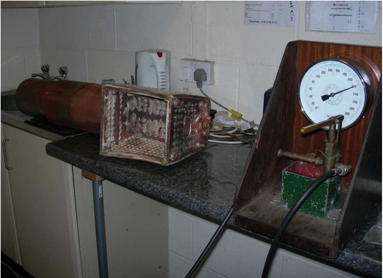
Photo 23 LMS Duchess on boiler proof testing, before build. -
