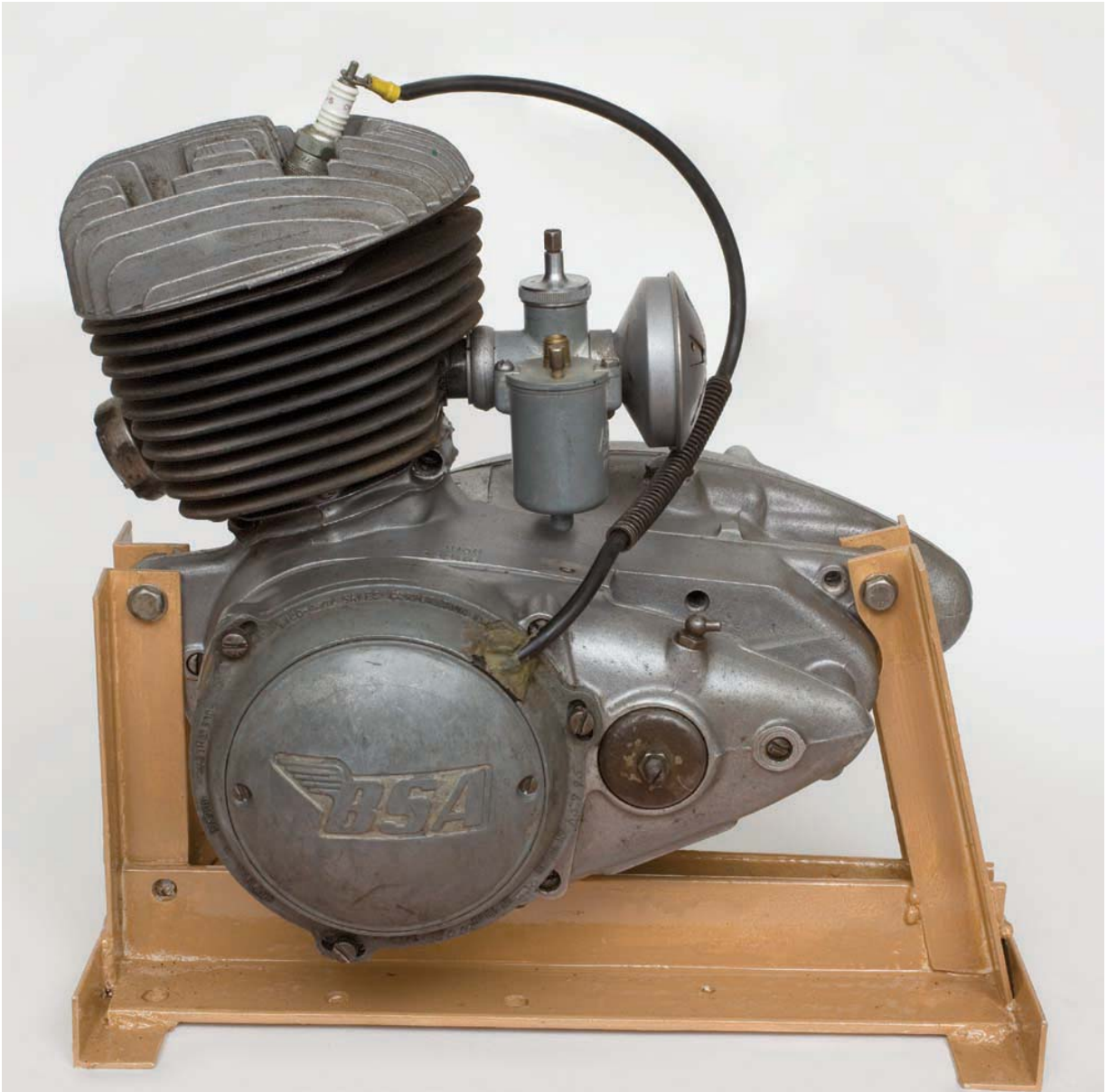
Photo 32 148cc two stroke BSA classic motorcycle engine, on handling stand.
