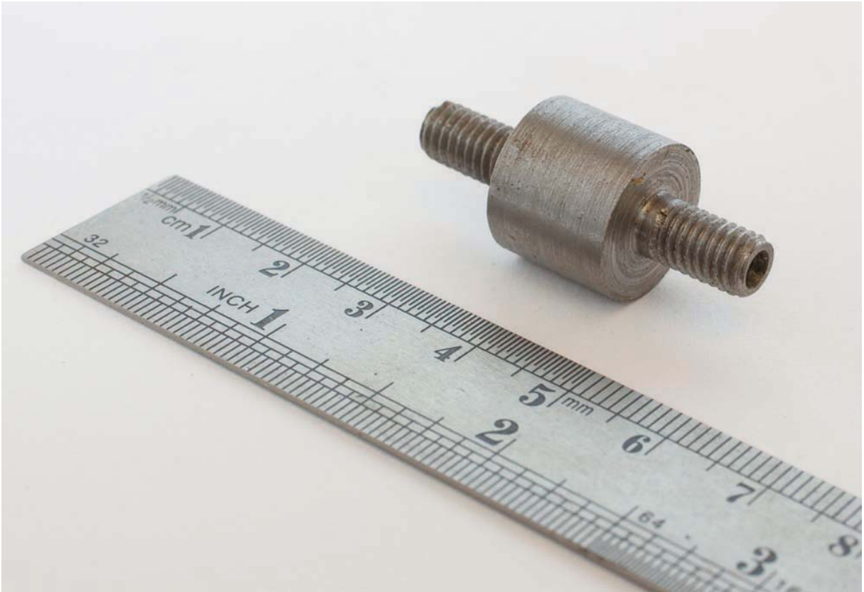
Photo 137 Case hardening completed by quenching and clean-up. Plain surface hard, threads as received.
