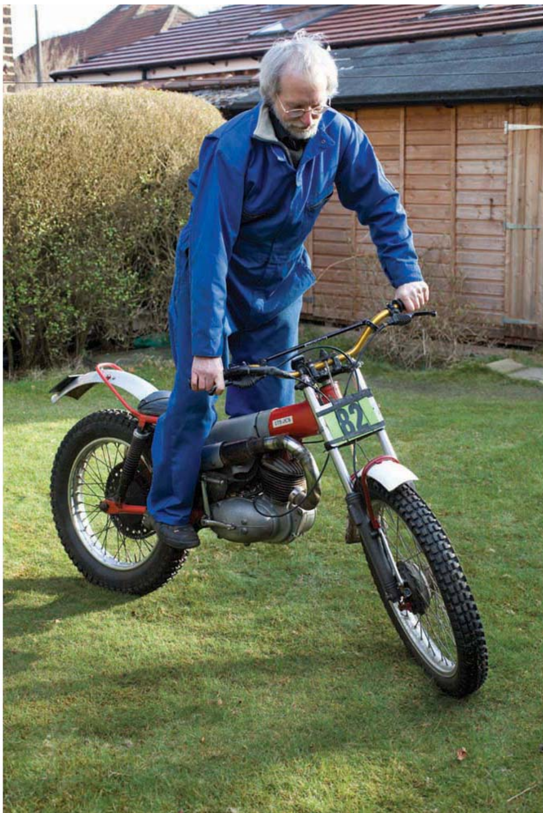
Photo 53 JCS, pre-65 trials special, based on 4" (100mm) dia. mild steel tubing for frame and fuel tank.
