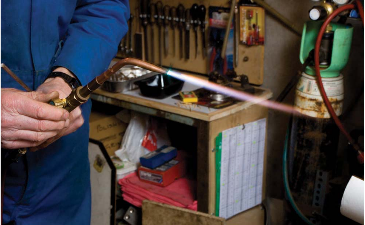
Photo 47 Oxyacetylene, versatile general heat source for hot working, welding and brazing/bronze welding.
