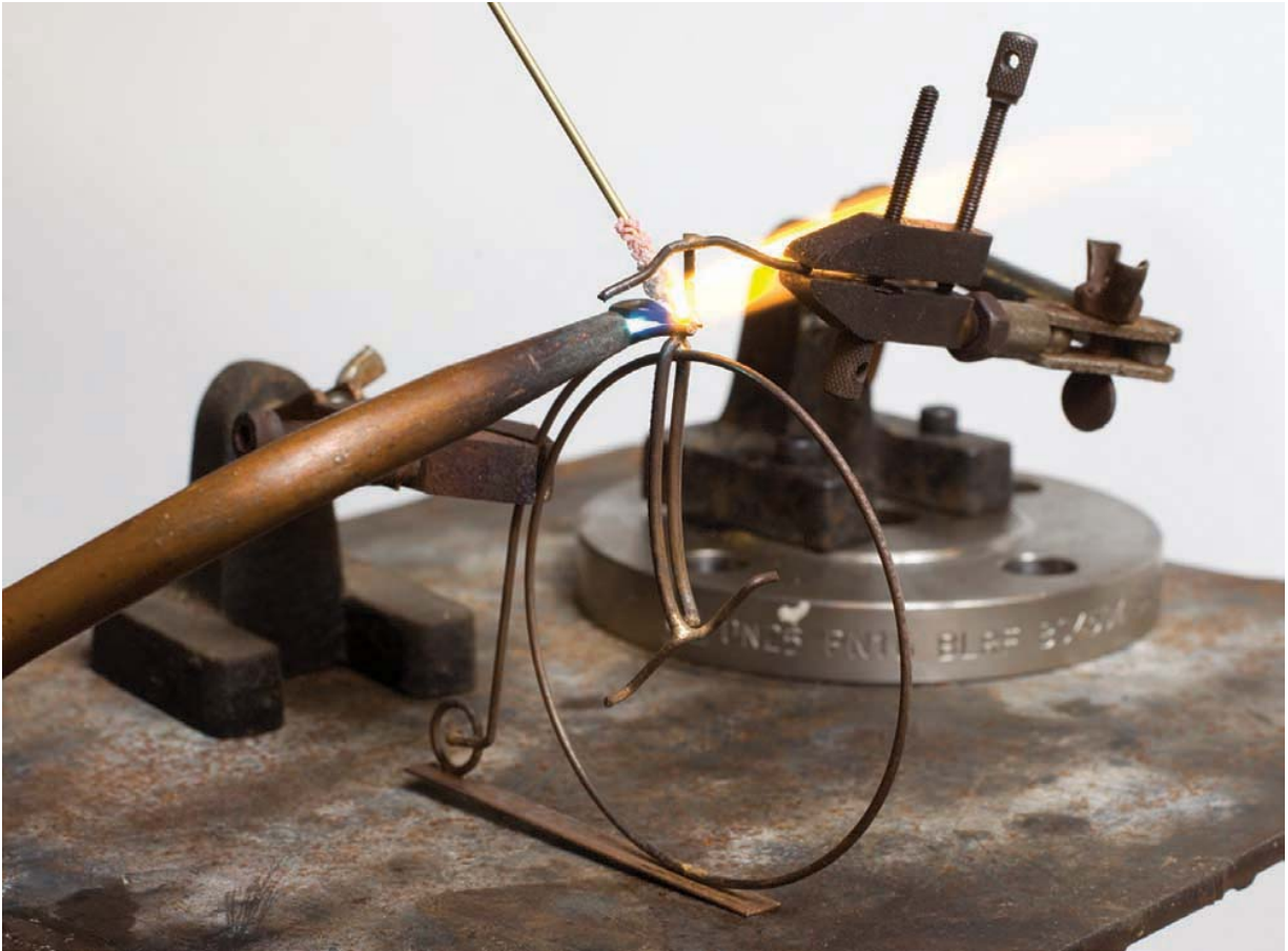
Photo 49 Further bronze welding as Photo 50, small jigs and clamps required to hold components.
