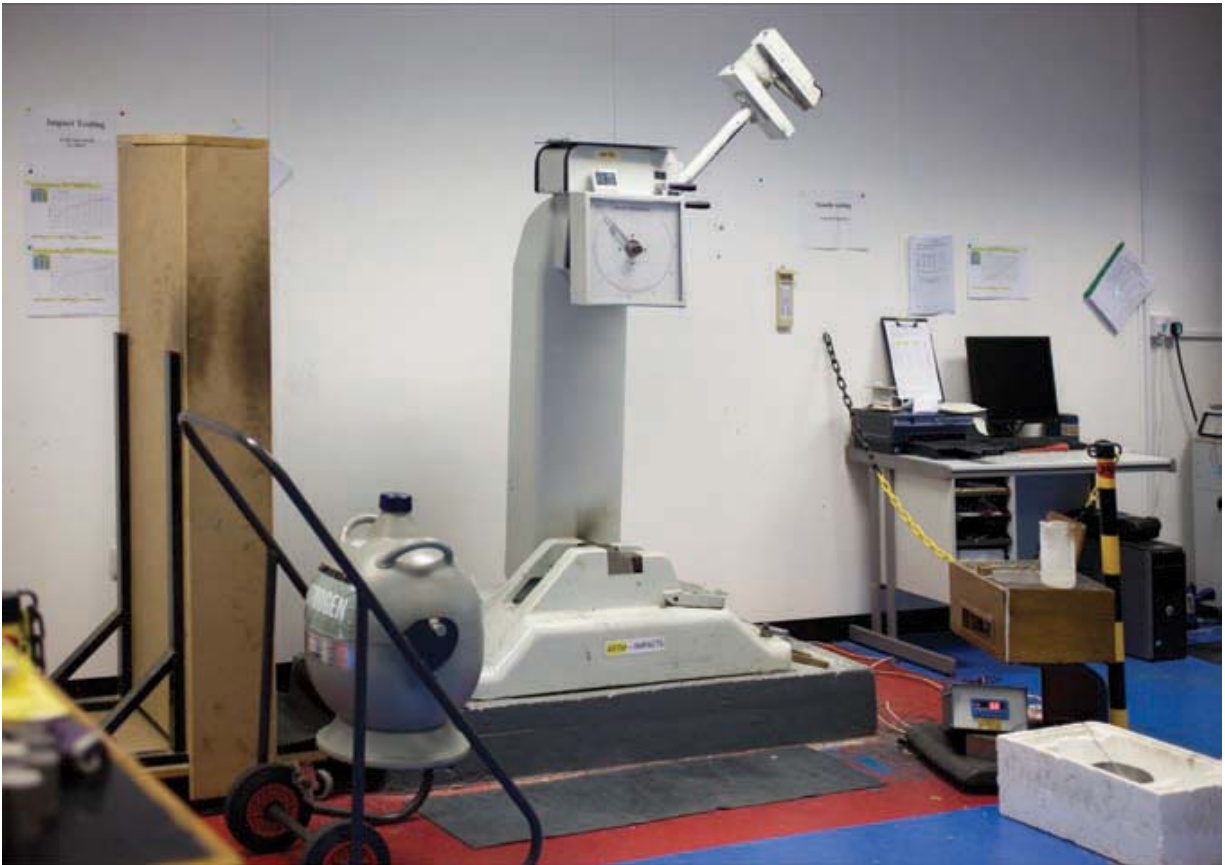
Photo 69 Charpy impact test apparatus, ready for testing.
