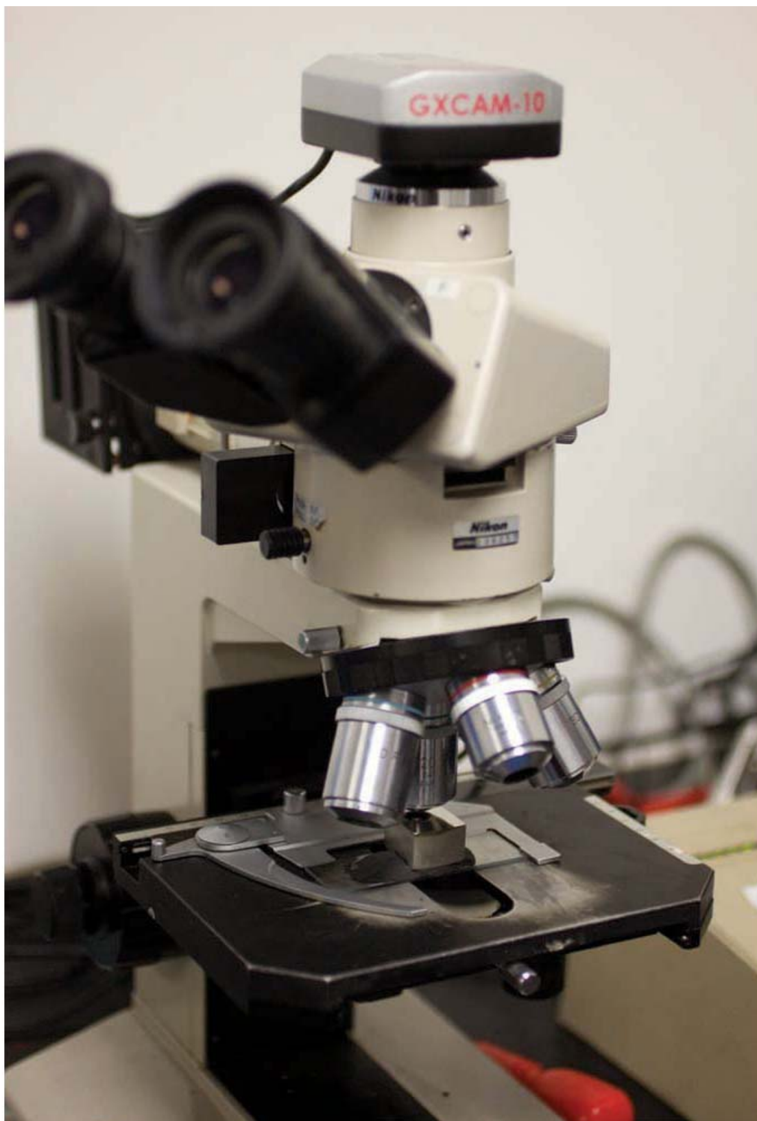
Photo 89 Optical microscope for metallographic micro testpiece examination.
