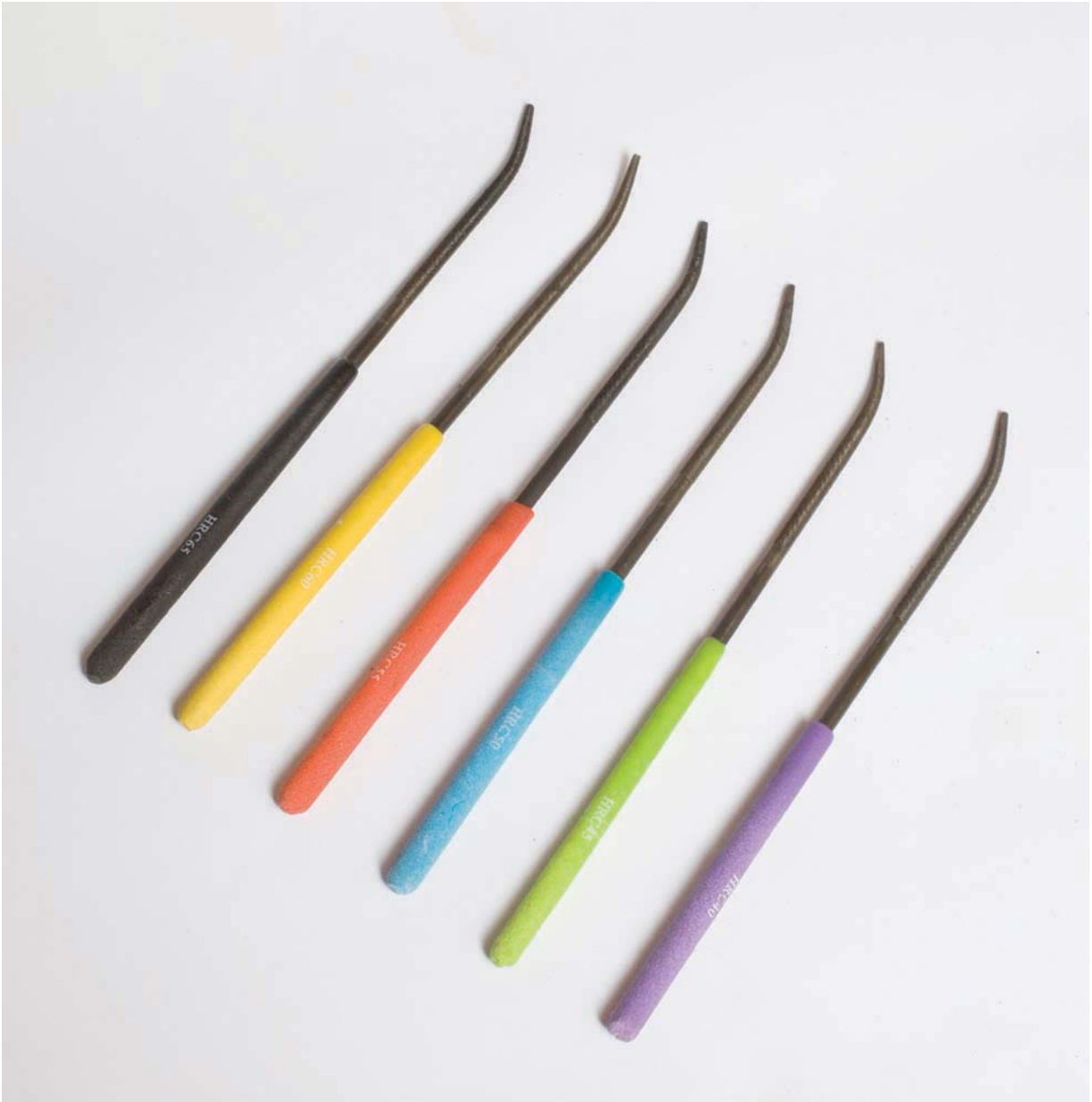
Photo 144 Comparative hardness testing, for hard steels, with graded files from 40 to 65 HRC (Rockwell hardness, C scale).
