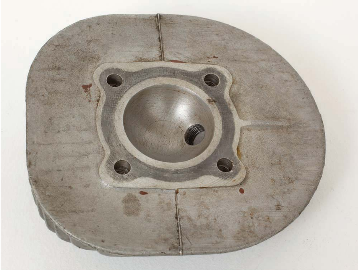
Photo 34 Cylinder head, showing combustion chamber and casting mould separation line.
