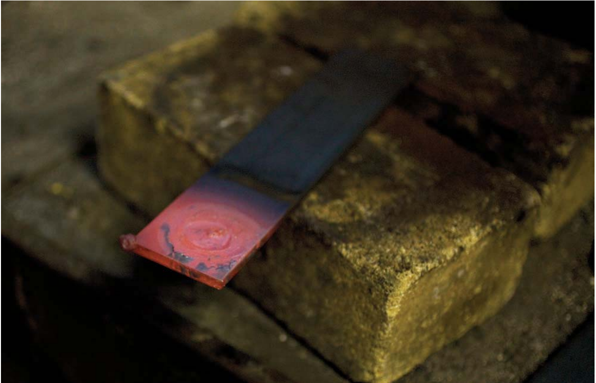
Photo 120 Material at lower bound for hot forming (previously overheated).
