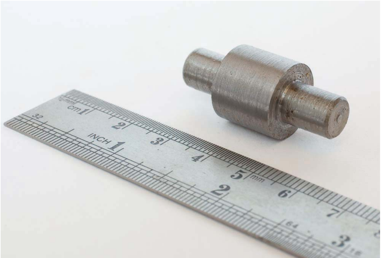
Photo 135 Case hardening sample, stage I, machined oversize, mild steel in as-received condition.
