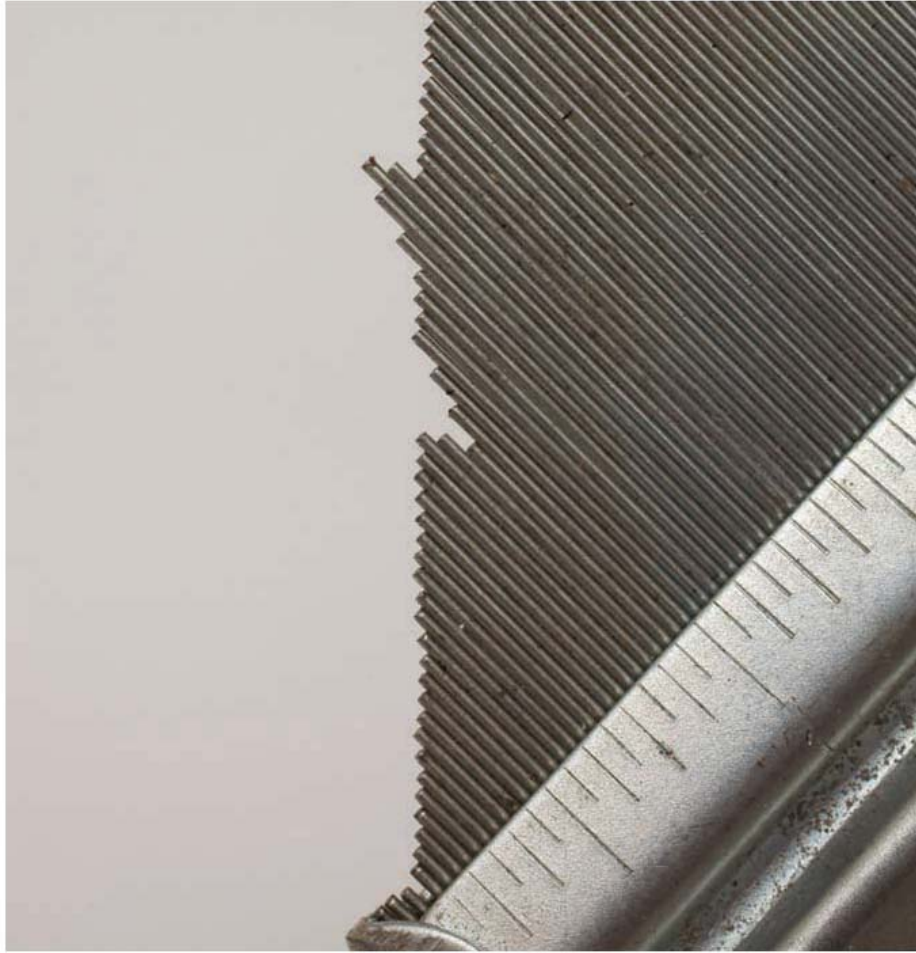
Photo 79 Model of intrusion and extrusion from Persistent Slip Bands, for Stage I fatigue crack initiation (using profile tool).
