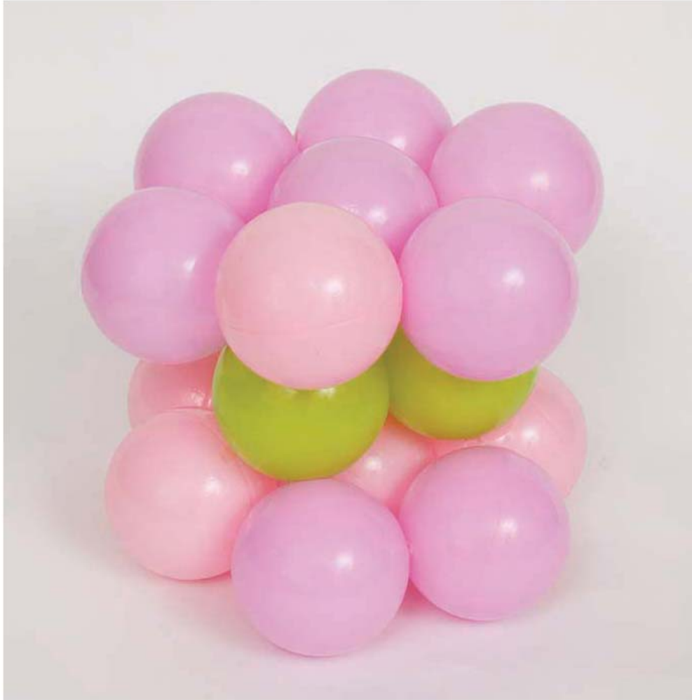
Photo 98 Model of hcp (hexagonal close packed) atomic structure.
