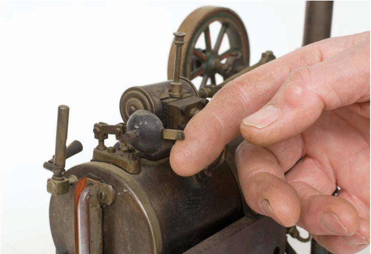
Photo 12 Further detail of photo 10, injector pump and its exhaust.
