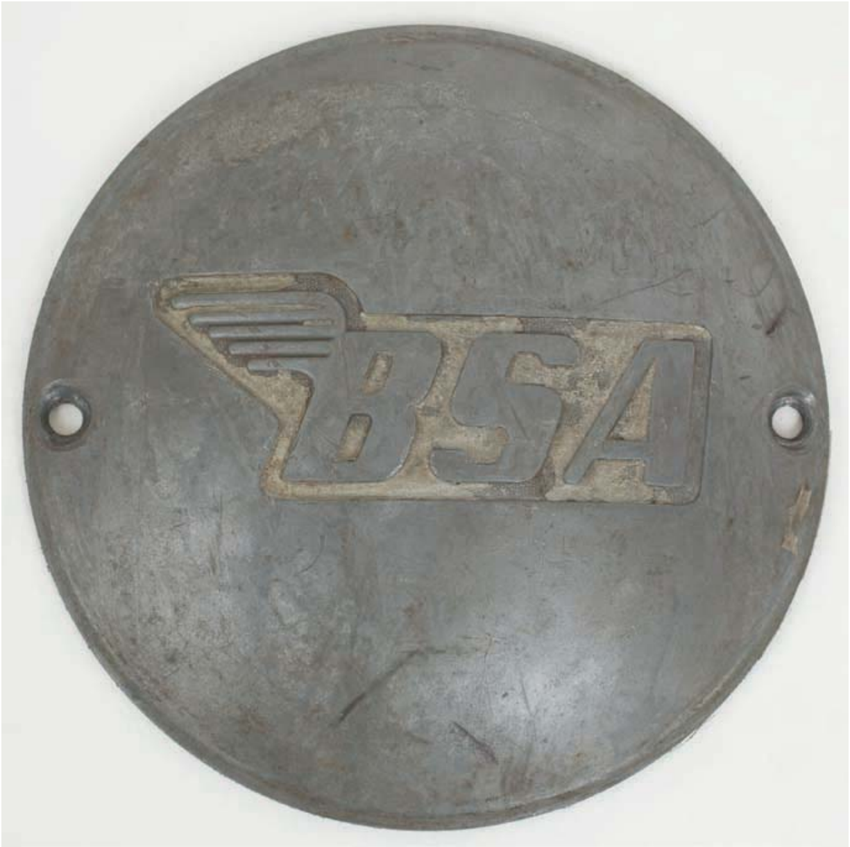
Photo 44 Zinc based alloy, fine die cast for non-structural magneto cover.
