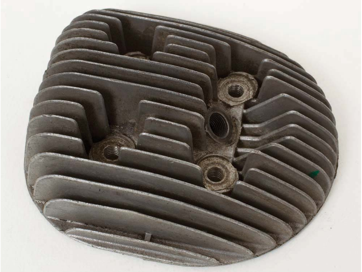
Photo 33 Cylinder head casting, showing deep finning possible for economic manufacture by sand casting.
