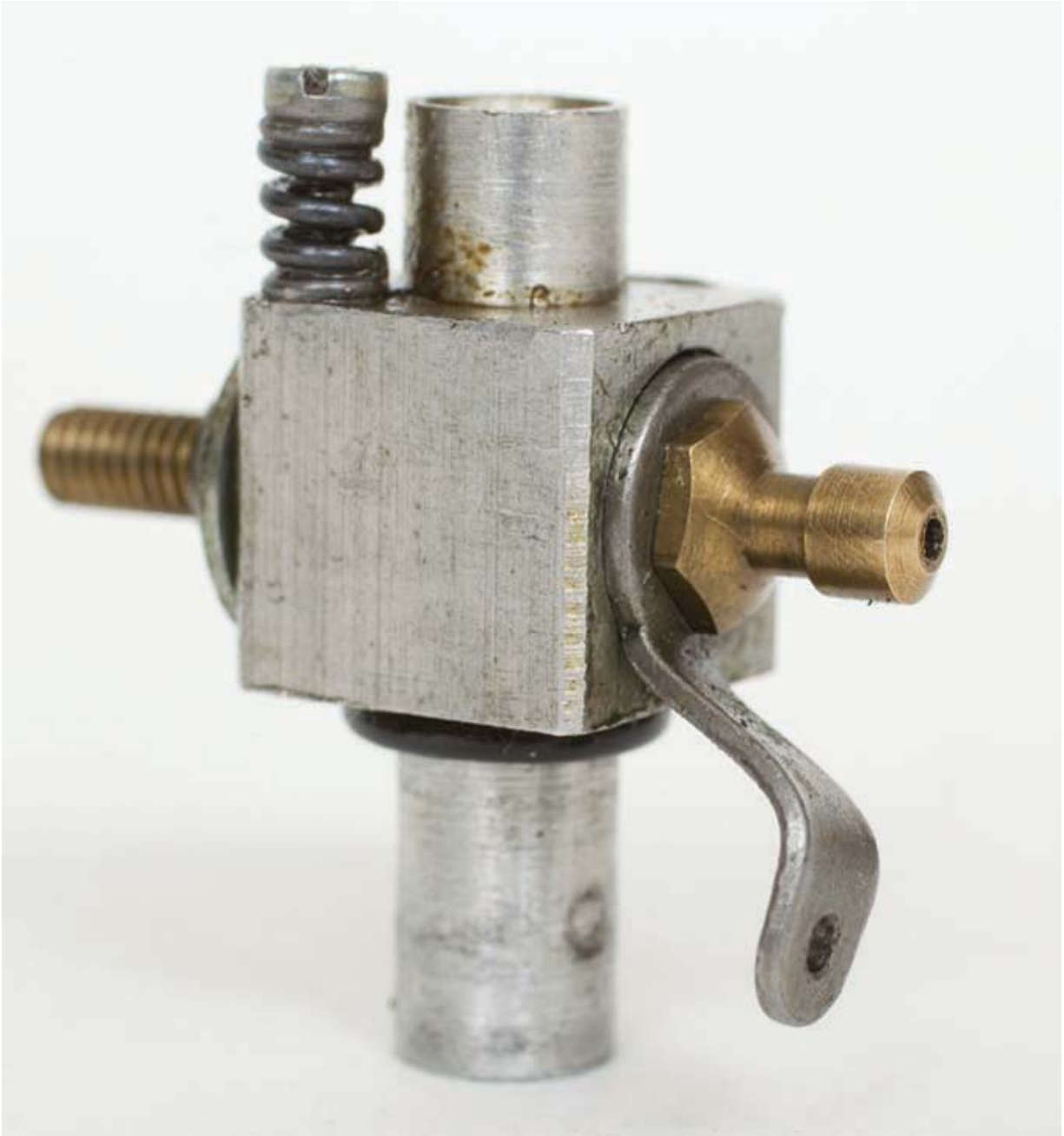
Photo 30 Spray unit, analogous to a carburettor, for fuel supply to inlet port, with controls for speed variation and cut-off.
