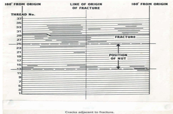
Photo 86 Markham colliery; diagram of cracks found by NDE on brake rod thread.
