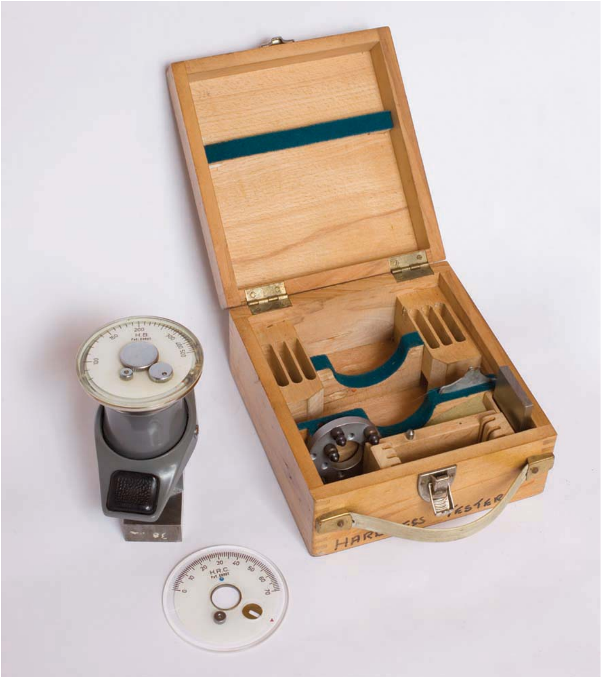
Photo 142 Portable hardness tester for variety of steel testing.
