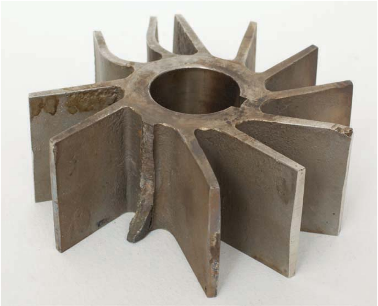
Photo 77 Impeller, 115mm across blade tips, bending fatigue failure.
