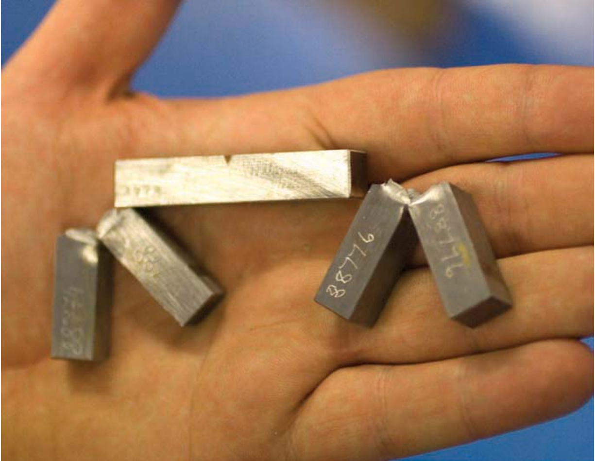
Photo 68 Charpy impact test specimens, surface deformation (shear lips) indicates high ductility and impact values.
