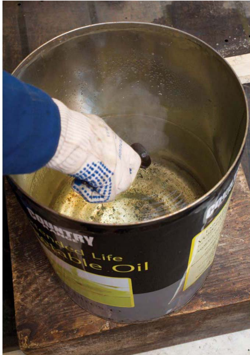
Photo 130 Immersion of testpiece for rapid quench into water.
