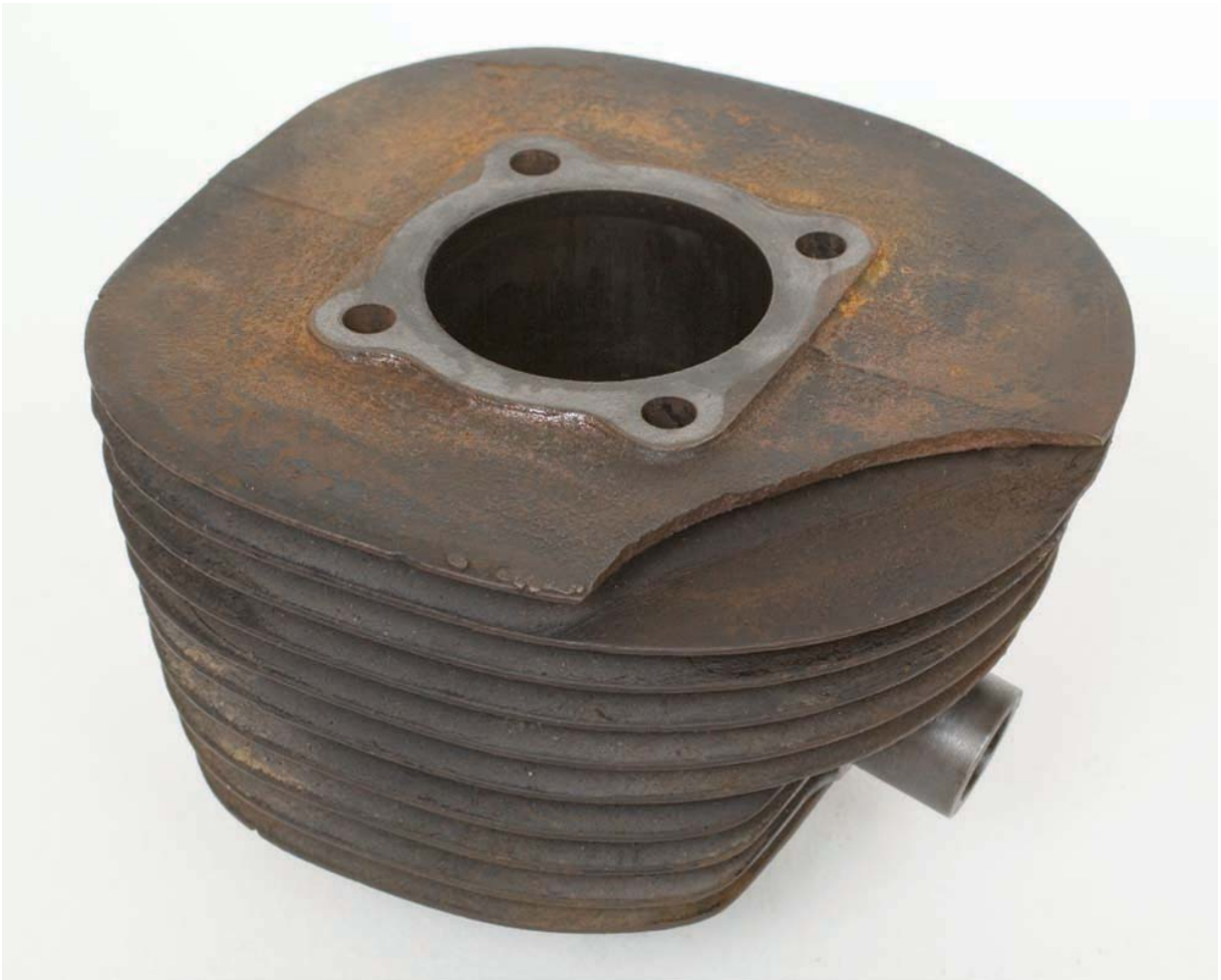
Photo 35 Cast iron cylinder, deep finning and fin fracture with no local plastic deformation.
