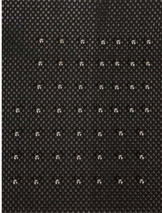
Photo 105 The 'line dislocation' continues through the structure.
