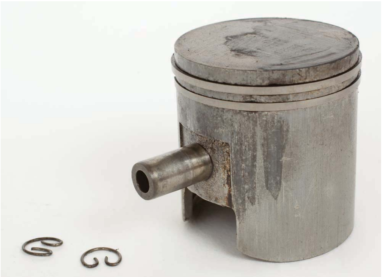
Photo 43 Piston with gudgeon pin and compression rings. Scoring shows prior minor seizure.
