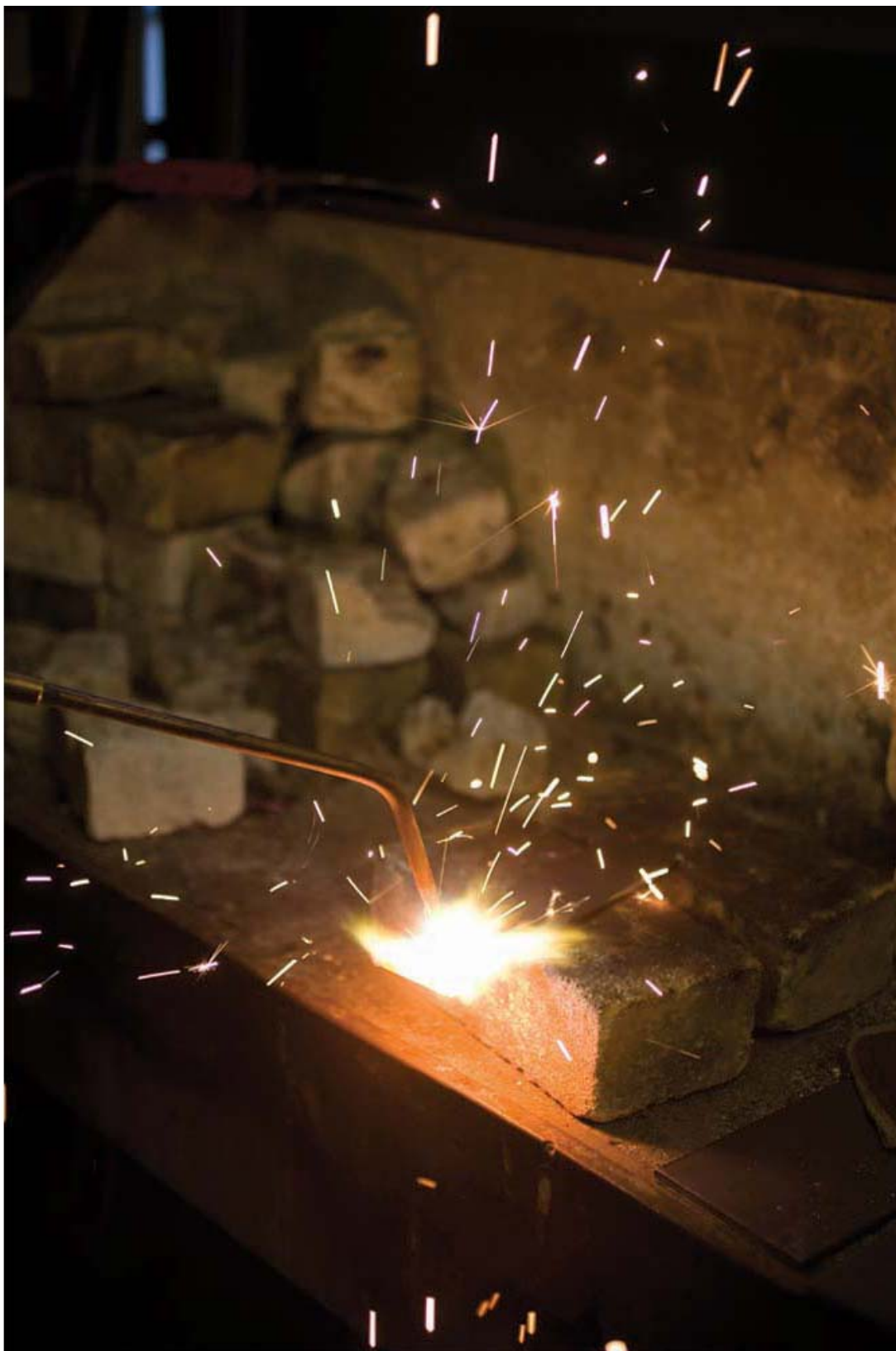
Photo 122 Gross overheating of material, with rapid surface emissions and metallurgical damage.
