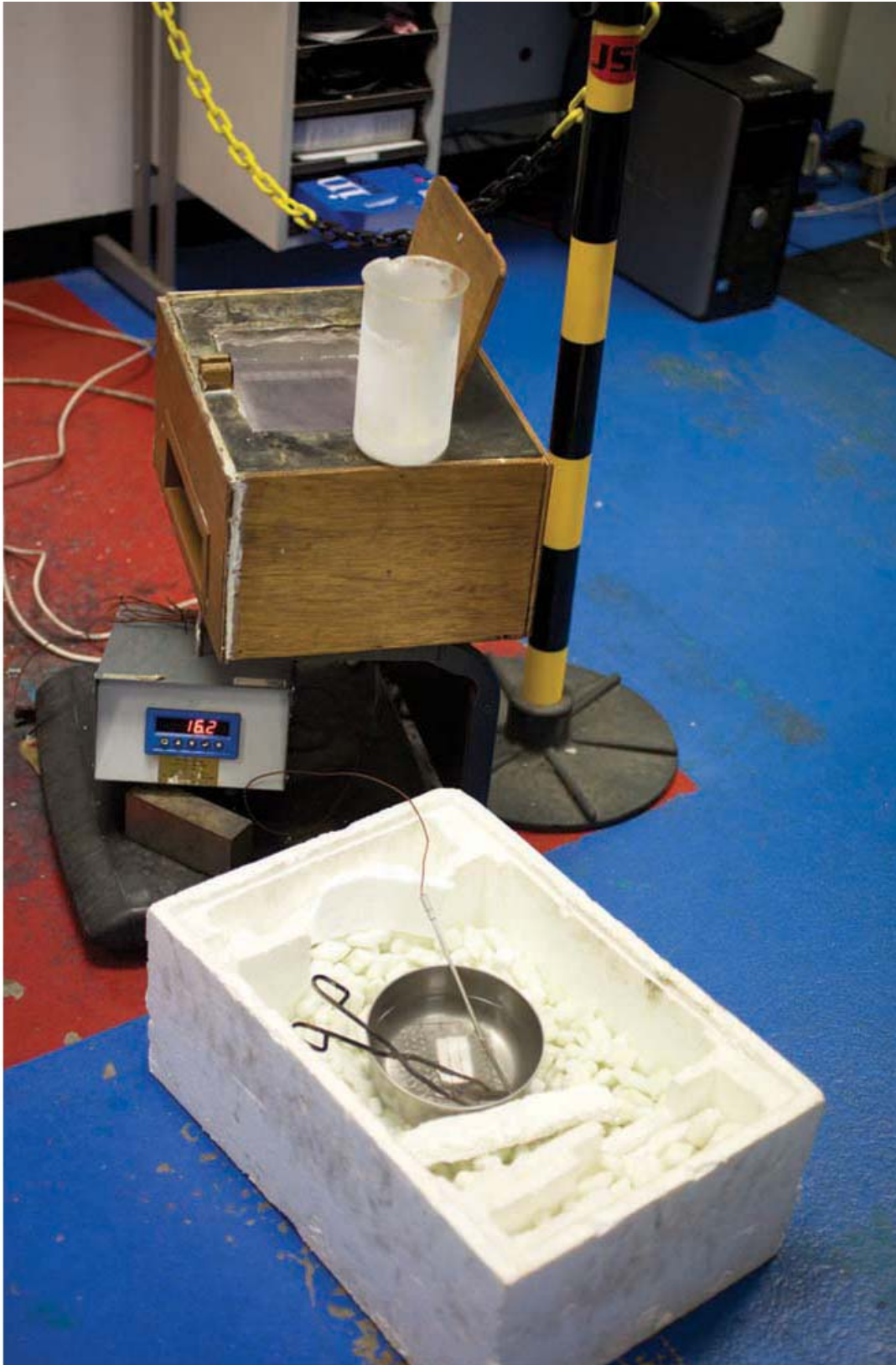
Photo 70 Sub-zero coolant bath for Charpy impact test pieces.
