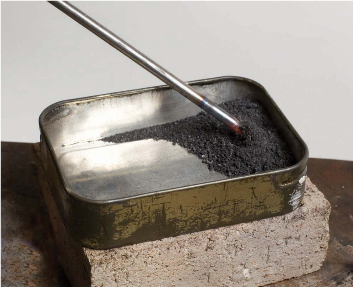
Photo 132 Direct hardening of steel bar into carburizing (case hardening) compound.
