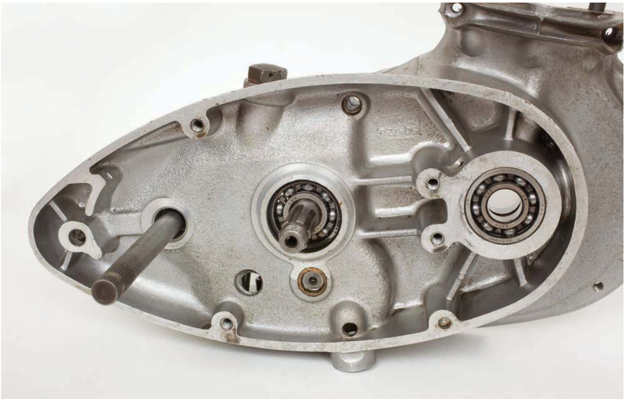
Photo 38 Aluminium crankcase half, with interference fit ball bearings.
