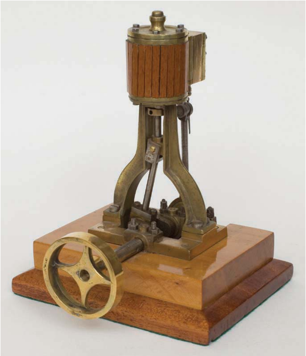
Photo 6 General purpose proprietary vertical engine, popular in factory mills and workshops, seen in the film The African Queen.
