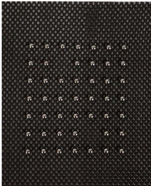
Photo 100 Ball bearing model of a 'vacancy' (missing) in a metal grain.
