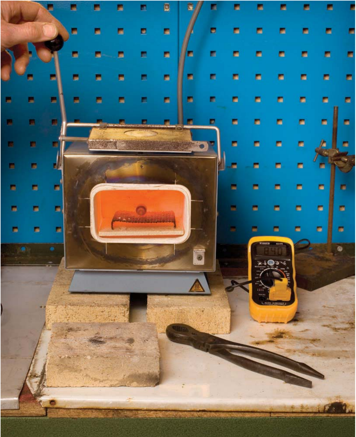
Photo 134 Heat treatment sample, ready for removal from furnace after soaking at temperature.
