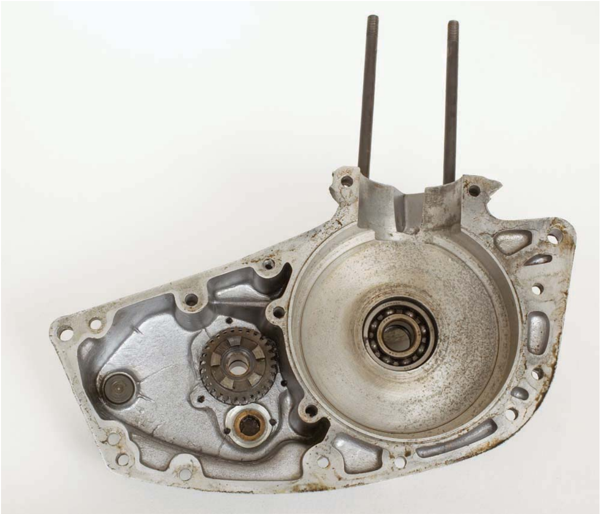
Photo 39 Crankcase internal view, showing casting detail.
