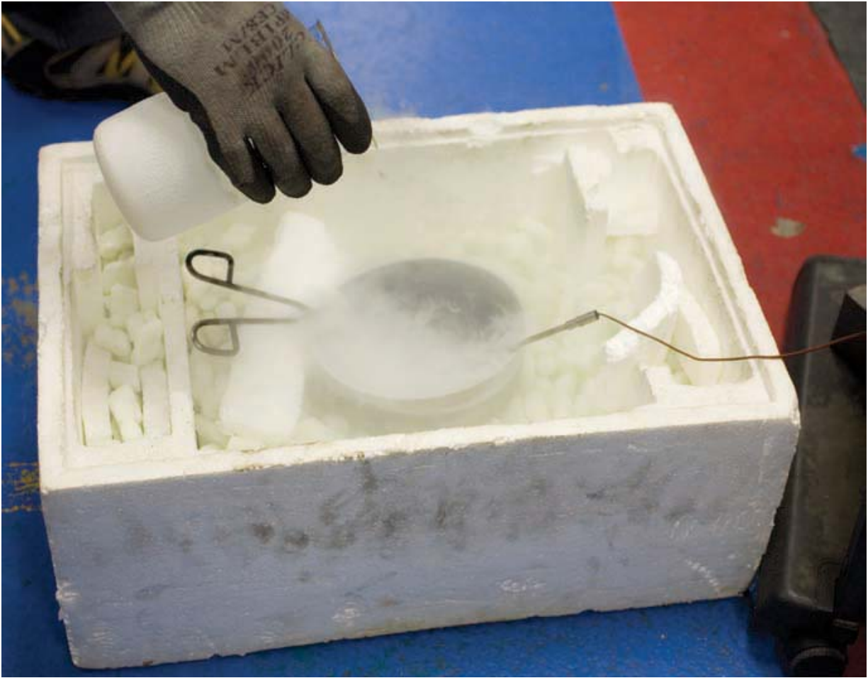
Photo 71 Testpieces in coolant bath for testing at -20^{\circ}\text{C} .
