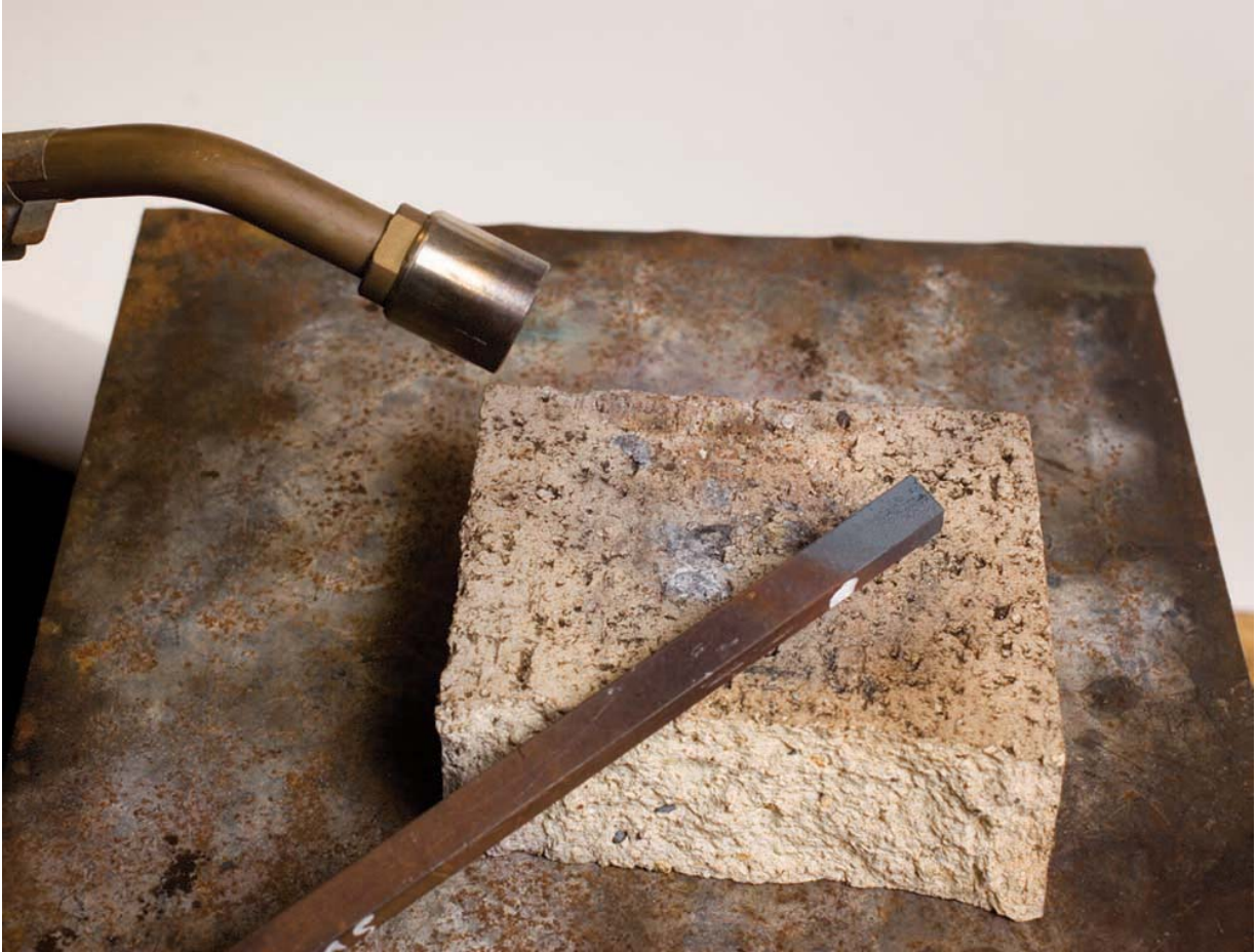
Photo 115 Butane gas heating torch, lower heat output but can be more manageable than oxy-acetylene for soldering.
