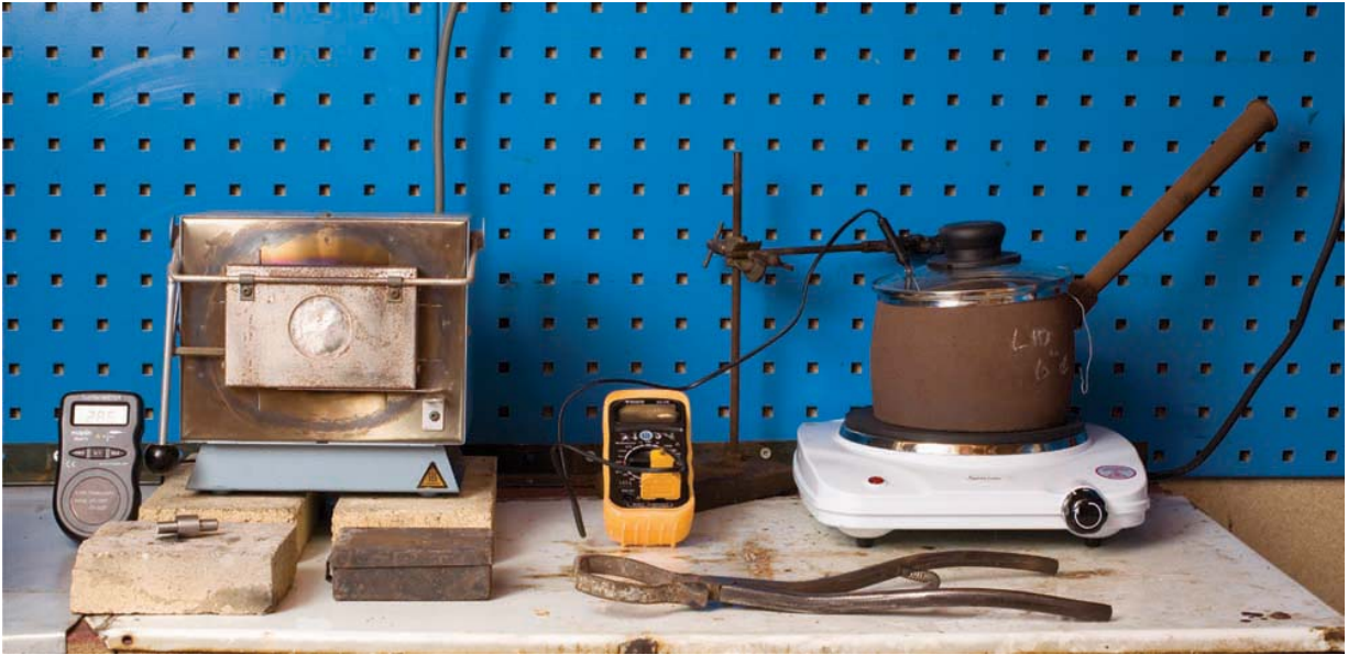
Photo 131 Basic heat treatment facility for small samples, heat treatment furnace, and salt-pot heating with digital temperature monitoring. (Thermal insulation removed for clarity.)
