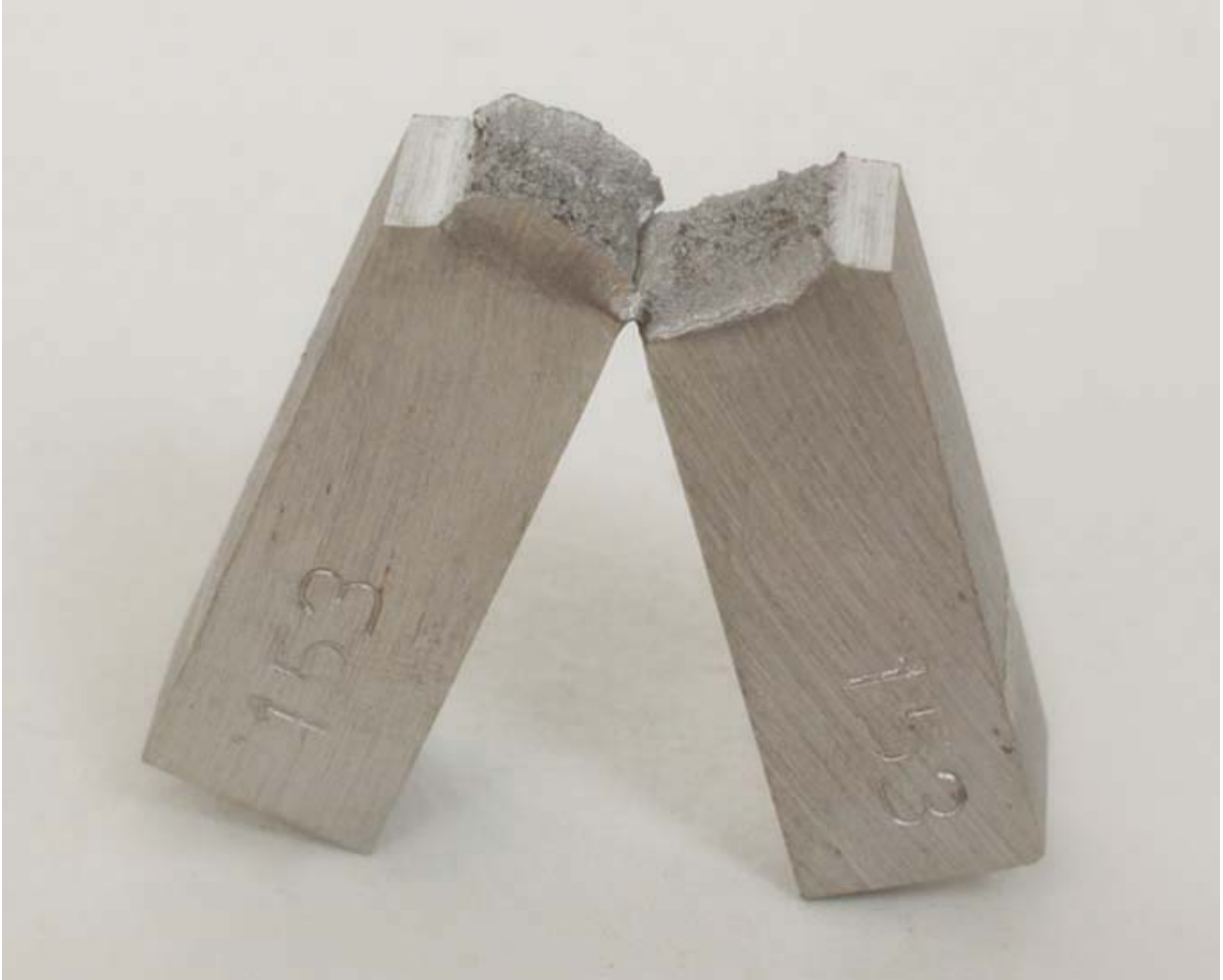
Photo 72 Impact test pieces, brittle fracture, low ductility and impact values, compare Photo 71 .
