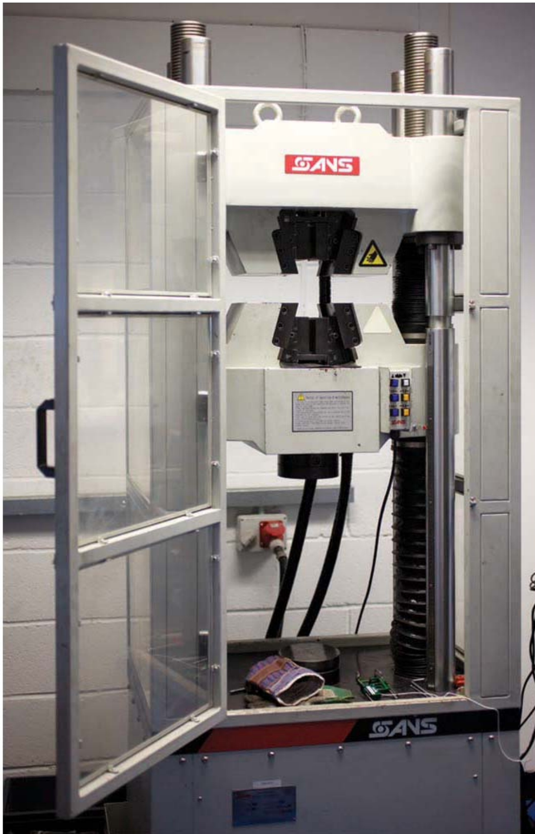
Photo 61 Tensile test machine, also possible to employ for uni-axial fatigue testing.
