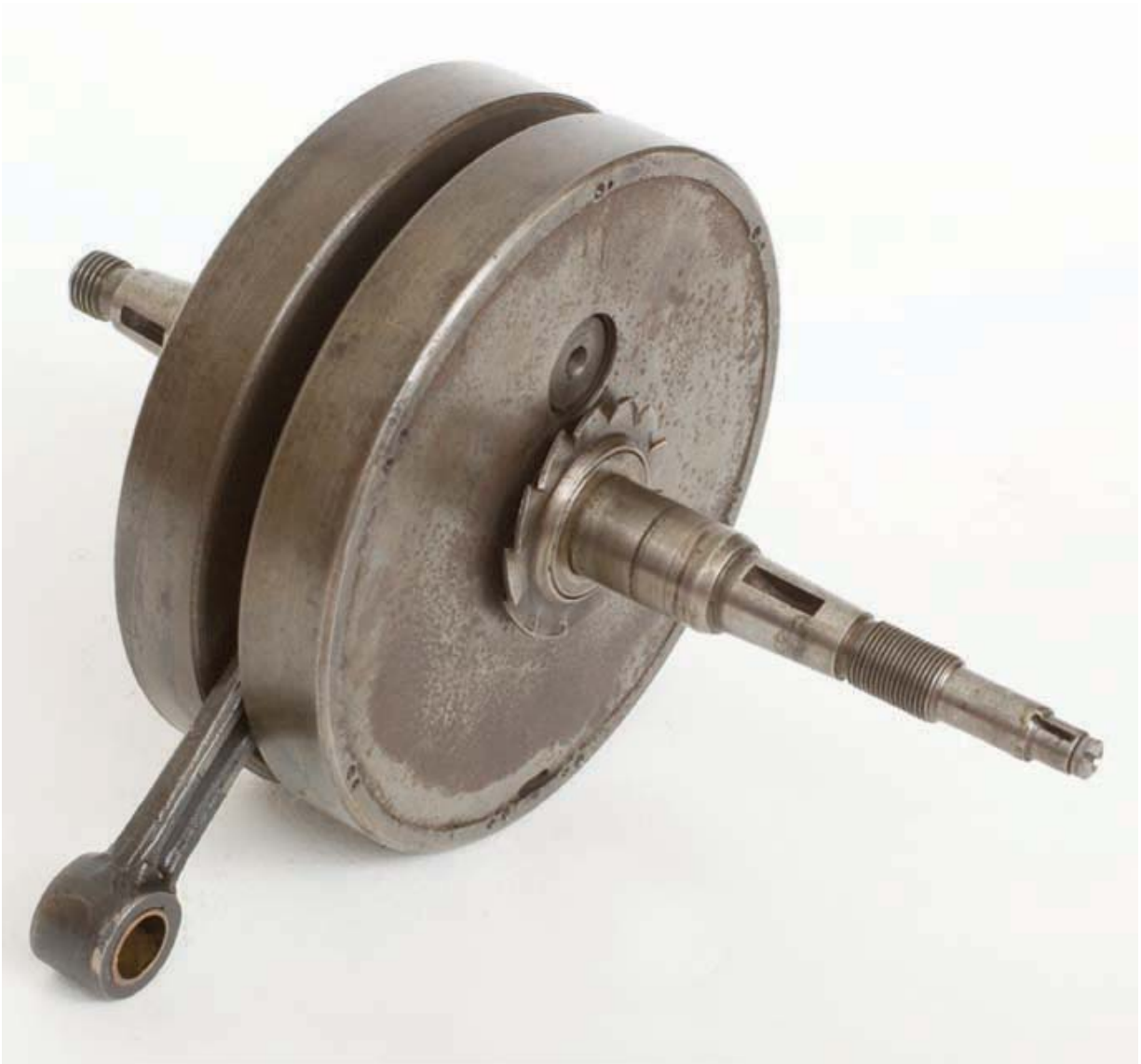
Photo 37 Flywheel/crankshaft/connecting rod assembly, showing standard mild steel flywheel discs to assist performance.
