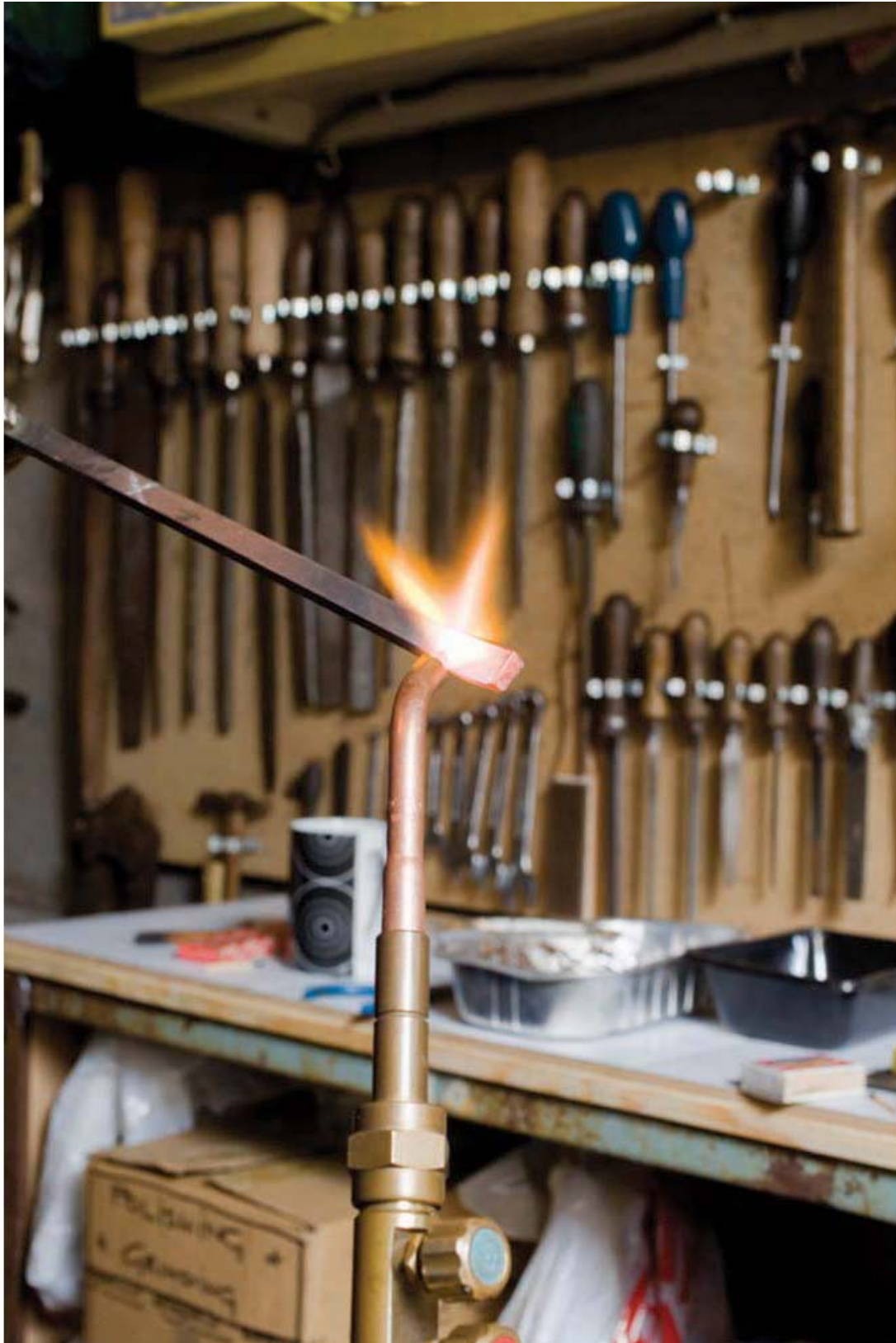
Photo 117 Oxy-acetylene torch held ready for hot working of bar material.
