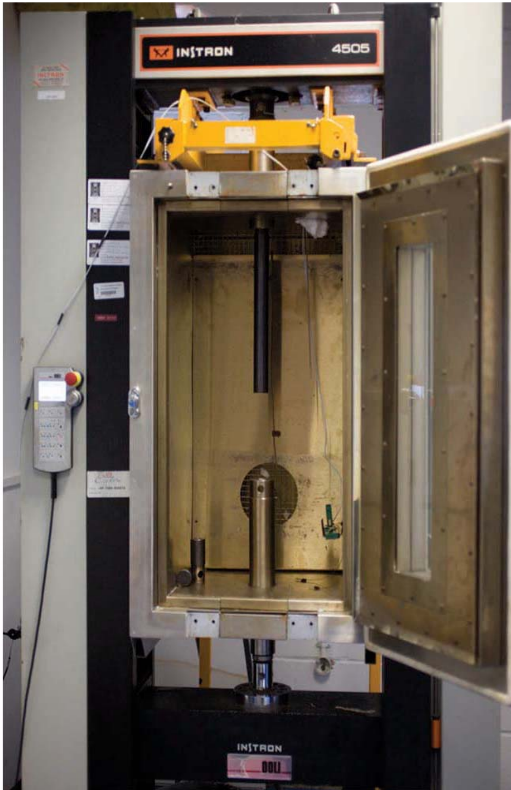
Photo 62 Tensile and creep testing machine, with elevated temperature facility.
