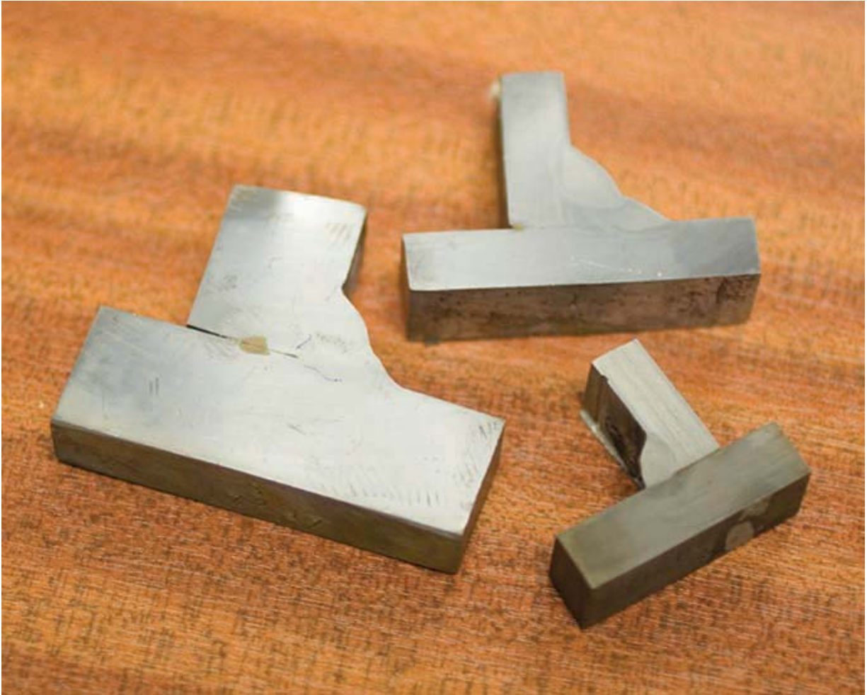
Photo 67 Selection of single-sided fillet weld sections, macro preparation.
