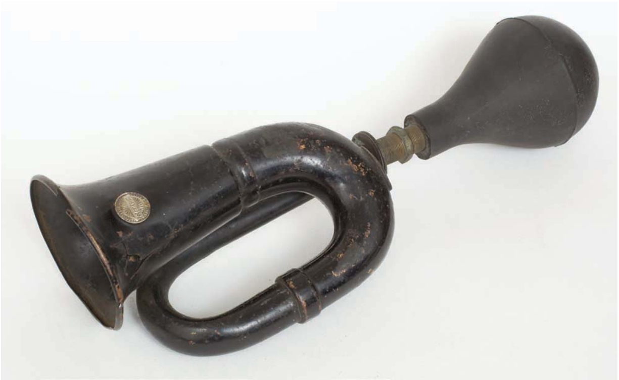
Photo 57 Early vehicle bulb horn, c. 1920, for vintage motorcycle.
