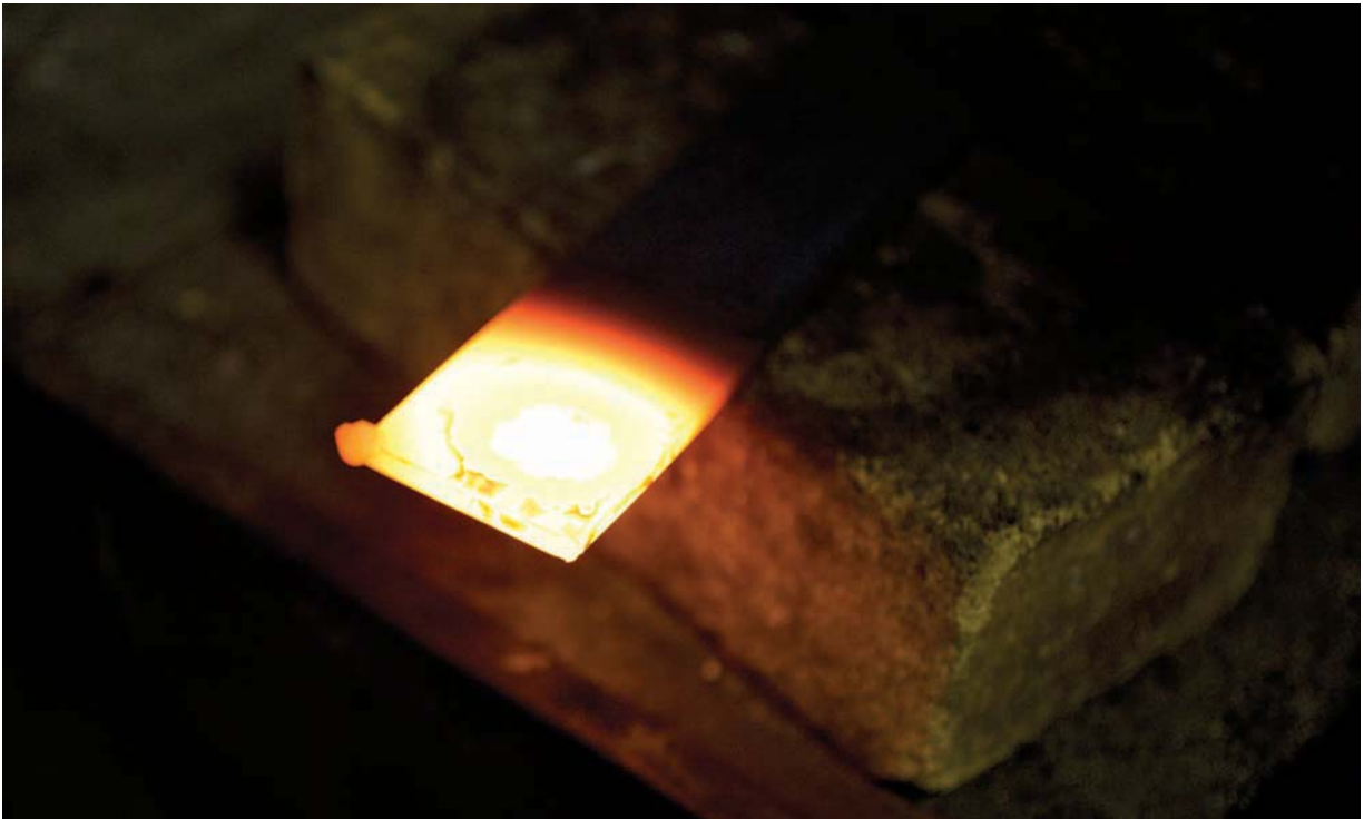
Photo 121 Material at higher bound for hot working, can lead to excessive grain growth if overdone.
