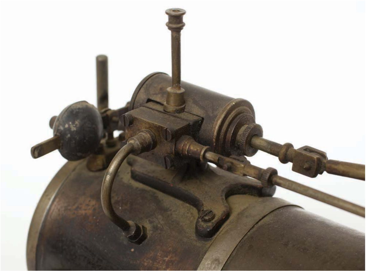
Photo 11 Detail of photo 10, gravity operated pressure relief valve, simple and effective!
