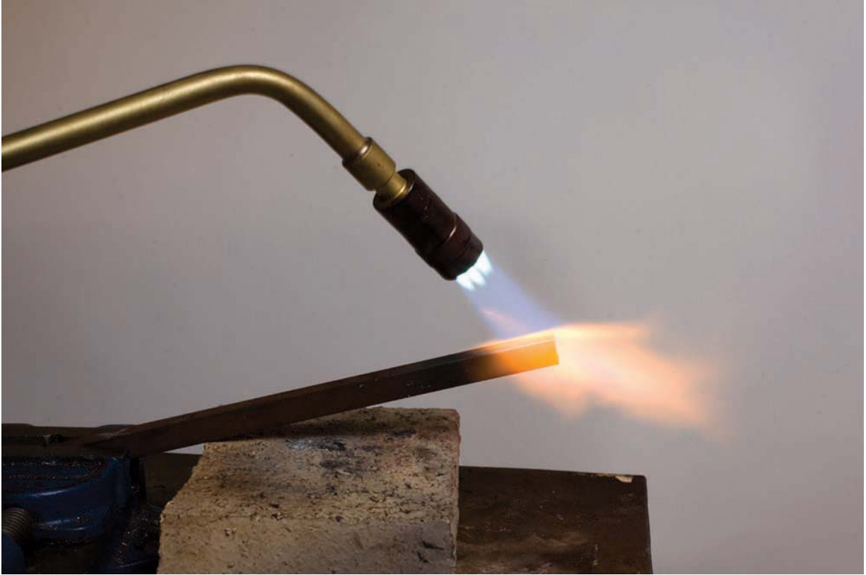
Photo 116 Oxy-acetylene torch with 'pepperpot' (multi jet) nozzle for more general heating than with a welding jet.
