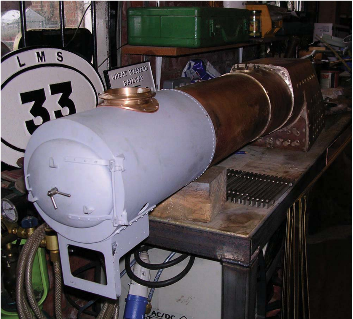
Photo 14 Boiler build nearing completion in Ron Perry's workshop.
