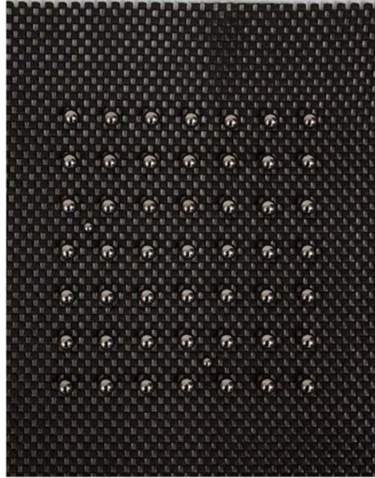
Photo 101 Ball bearing model of crystal array, containing two 'interstitials', (superimposed, smaller, atoms).
