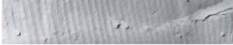
Photo 78 Fatigue fracture face details, striations clearly visible: (a) direct testpiece SEM at 1 micron spacing; (b) SEM replica, 4000x magnification; (c) SEM replica, 10000x magnification.
