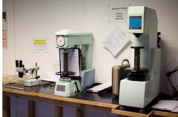
Photo 92 Macro viewer, Brinell and Rockwell laboratory hardness testing machines.
