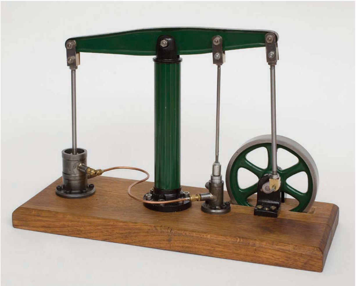
Photo 7 Simple beam engine as used in the early nineteenth century Industrial Revolution for general power source.
