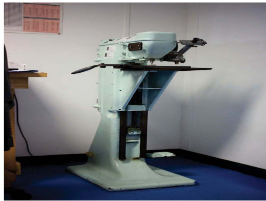
Photo 93 Traditional floor-standing manual Vickers hardness tester.
