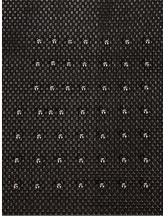
Photo 103 Model of an introduced 'dislocation' (crystal imperfection), as an extra plane of atoms.
