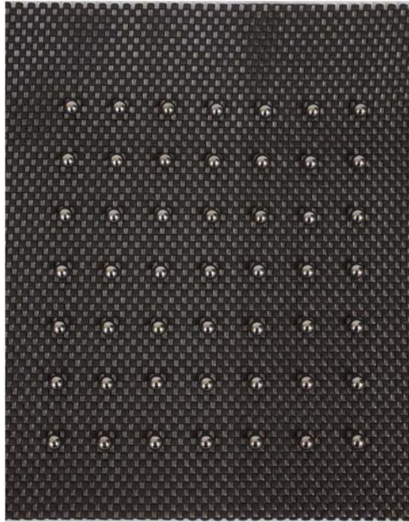
Photo 102 Model of perfect crystal array, with no defects.
