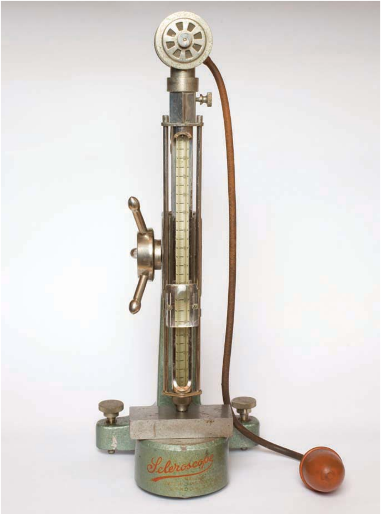
Photo 143 Shore Schleroscope hardness tester, particularly accurate for larger pieces.
