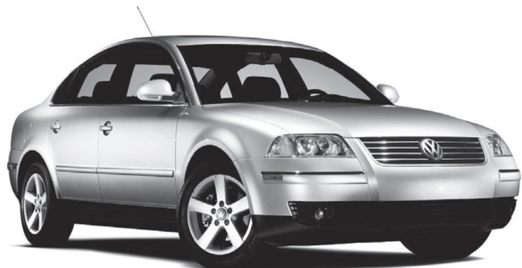
FIGURE 33.2 The Volkswagen Passat—a typical modern pressed-steel body with no separate chassis. For a given material this “monocoque” construction gives a minimum weight-to-strength ratio. (Courtesy of Volkswagen—photo credit to Brian Garland 2004)
