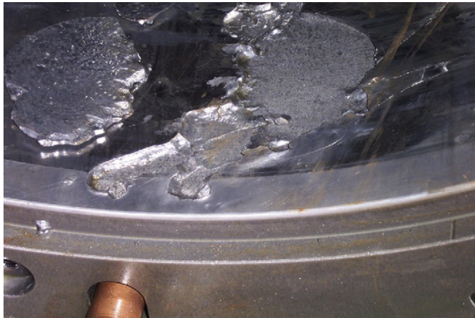
Propeller shaft white metal bearing
