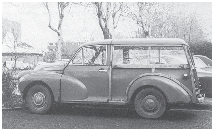
FIGURE 33.3 The Morris Traveller—a classic of the 1950s—used wood as an integral part of the body shell.
