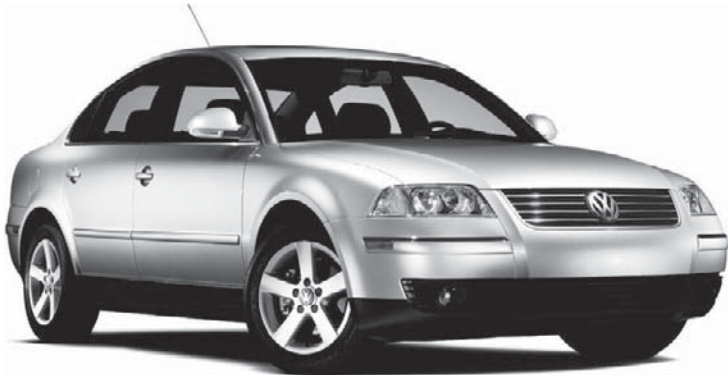
FIGURE 30.2 The Volkswagen Passat—a typical modern pressed-steel body with no separate chassis. For a given material this “monocoque” construction gives a minimum weight-to-strength ratio. (Courtesy of Volkswagen—photo credit to Brian Garland © 2004)
