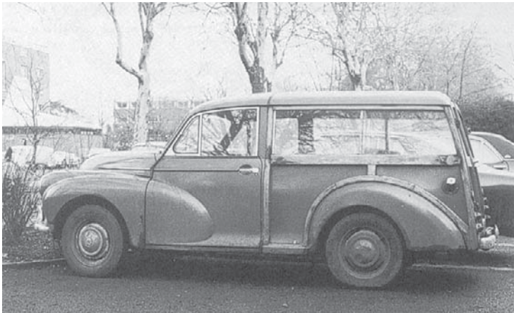
FIGURE 30.3 The Morris Traveller—a classic of the 1950s—used wood as an integral part of the body shell.
