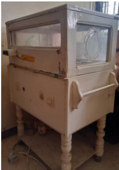
Fig. 3. Temperature and humidity-regulated enclosure
