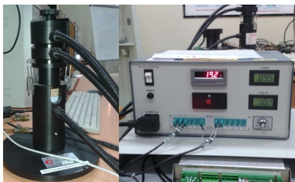
Fig. 4. H111 Heat Transfer Service Unit and Data Logger
