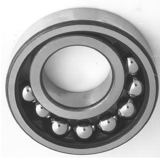
FIGURE 1.14 Photograph showing Conrad-type ball bearing components just before snapping the inner ring to the position concentric with the outer ring.
