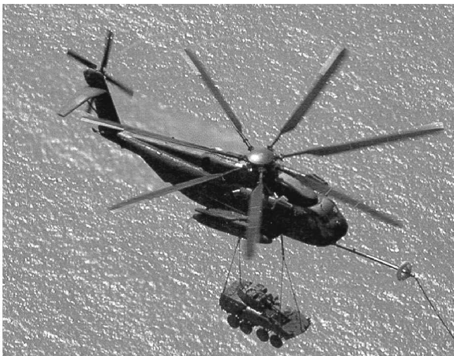
FIGURE 1.9 CH-53E Sikorsky Super Stallion heavy-lift helicopters employ ball, cylindrical roller, and spherical roller bearings in transmissions that power the main and tail rotors. (Courtesy of Sikorsky Aircraft, United Technologies Corp.)
