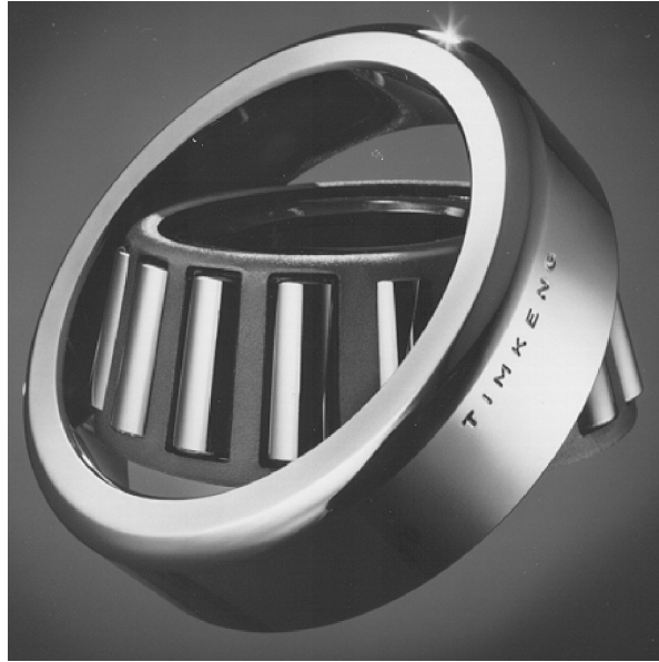
FIGURE 1.43 Single-row tapered roller bearing showing separable cup and nonseparable cone, cage, and roller assembly. (Courtesy of the Timken Company.)
