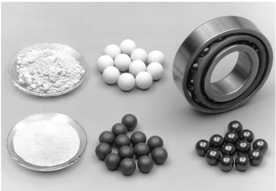
FIGURE 13.16 Bearing quality silicon nitride begins life as a powder before a series of processes transforms it into a highly engineered bearing component. (Photograph courtesy of SKF.)
