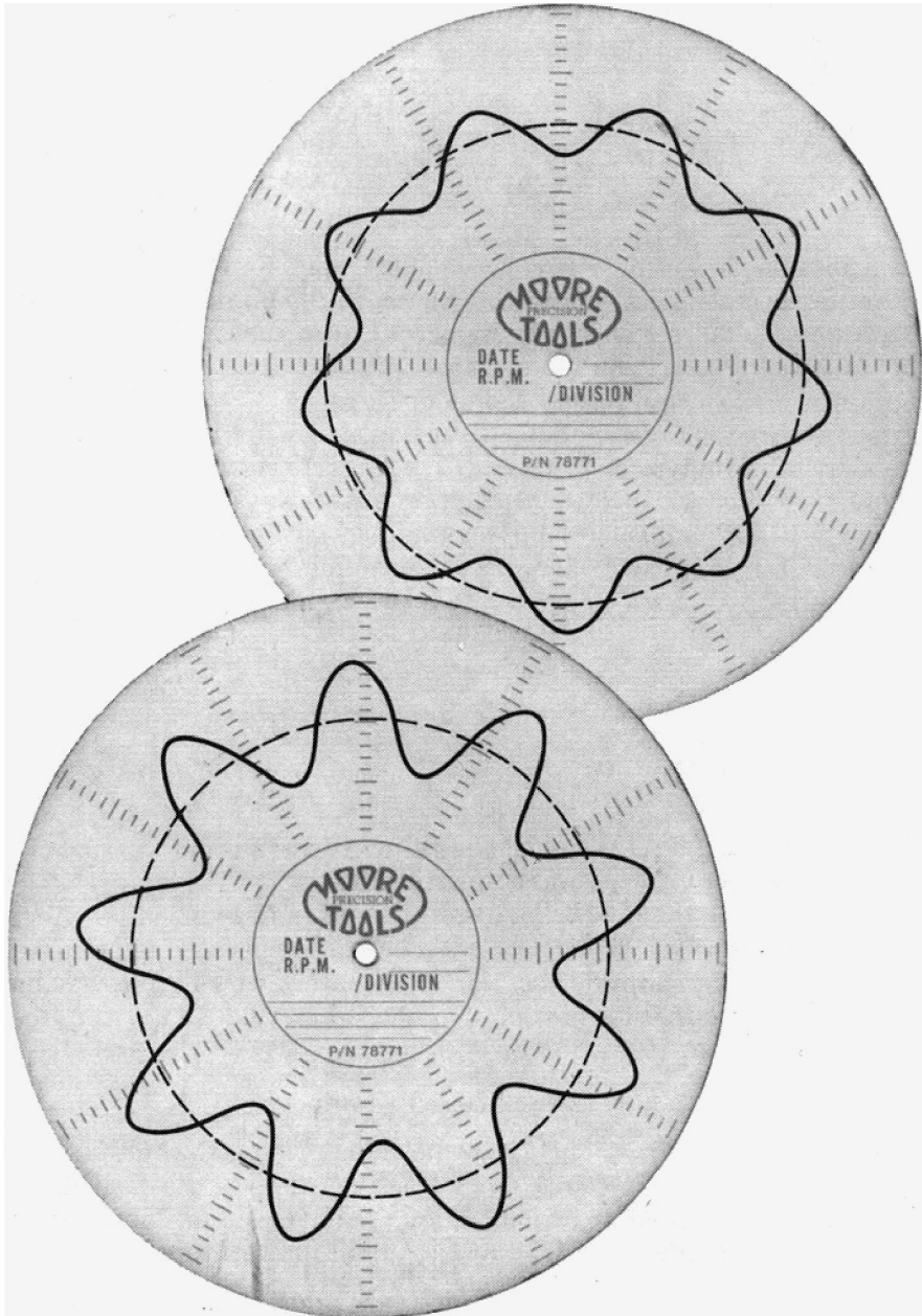
FIGURE 14.8 Spherical roller bearing inner-ring waviness, machine setup error. Each radial division equals 1 \mu\text{m} .
