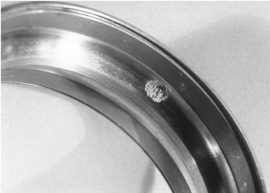
FIGURE 11.6 Fatigue spall in ball bearing raceway surface.
