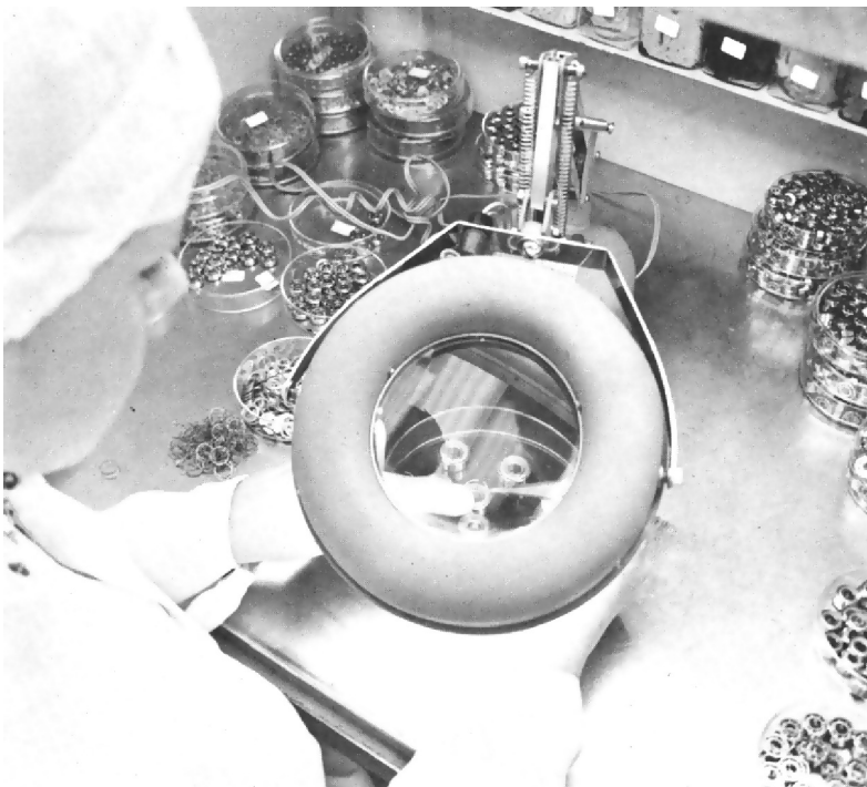
FIGURE 1.22 A delicate final assembly operation on an instrument ball bearing assembly is performed under magnification in a “white room.”
