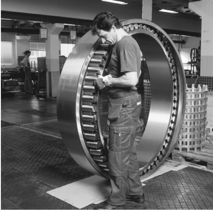
FIGURE 1.4 A large spherical roller bearing for a ball mill (mining) application. (Courtesy of SKF.)
