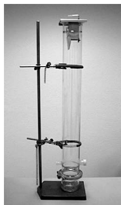
Figure 2.13: Apparatus for determining dusting behaviour of pigments
