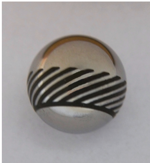
Figure 5.3 Spherical grooved bearing 8 mm diameter
