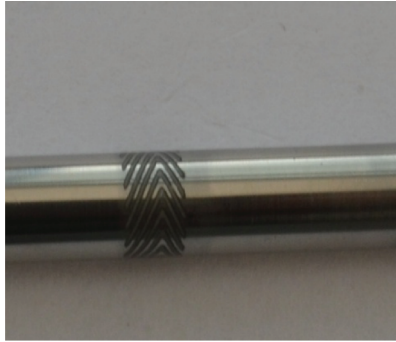
Figure 5.2 Herringbone grooved bearing on 4 mm diameter shaft
