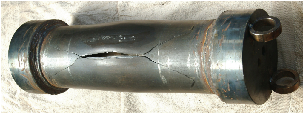
Fig. 36. Specimen after burst test
