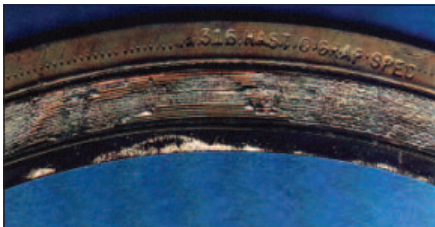
Oxidised spiral wound gasket
