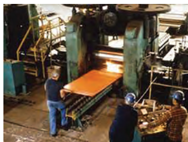
Fig. 9.9 Two-high rolling mill. This type of mill lends itself to rolling titanium sheet and plate. Courtesy of Timet
