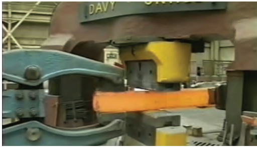
Fig. 9.1 Titanium ingot at the start of press forging. Ingot breakdown is done in a press with open flat dies so that the deformation rate can be controlled more closely and the as-cast ingot structure can be worked with less danger of cracking.
