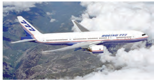
Fig. 15.10 Titanium use on the Boeing 777 accounts for approximately 15% of its gross empty weight.
