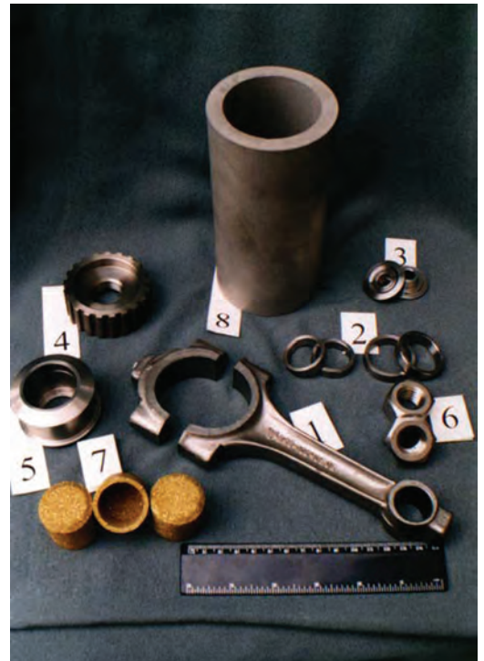
Fig. 8.33 Ti-6Al-4V parts produced using a pressed-and-sintered approach and titanium hydride. 1) Connecting rod with big end cap. 2) Saddles of inlet and exhaust valves. 3) Plate of valve spring. 4) Driving pulley of distributing shaft. 5) Roller of strap tension gear. 6) Screw nut. 7) Embedding filter, fuel pump. 8) Embedding filter. Courtesy of Ukrainian Academy of Sciences
