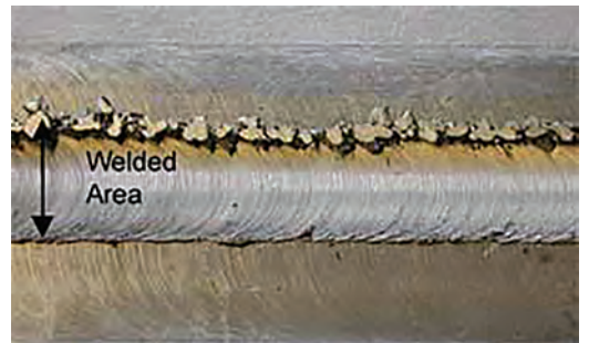
Fig. 12.14 Surface appearance of a good-quality friction stir weld in 6.35 mm (0.25 in.) thick Ti-6Al-4V. Source: Ref 12.18
