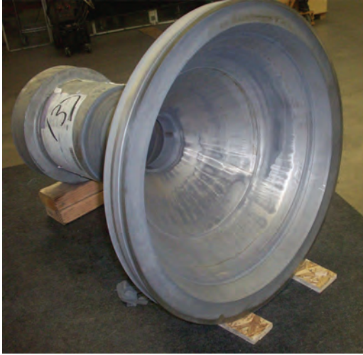
Fig. 8.43 Near-net shape Ti-6Al-4V engine casing fabricated using the prealloyed metal can method. Courtesy of Synertech PM Inc./P&W Rocketdyne
