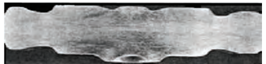
Fig. 10.14 The grain flow shown in this macrostructure of a closed-die radial section of a compressor wheel forging differs from that of the rolled ring in Fig. 10.13.
