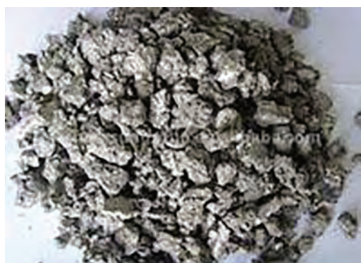
Fig. 1.25 Hydrogenated titanium sponge produced by the ADMA Products non-Kroll process. Courtesy of V. Moxson, ADMA Products, Sept 2013.
