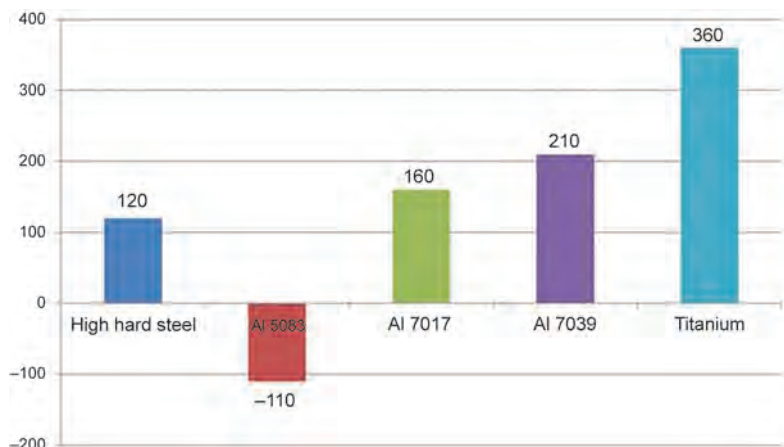
Fig. 15.28 Number of pounds reduced in weight compared to each 455 kg (1000 lb) of rolled homogeneous alloy steel at 14.5 mm (0.57 in.) armor-piercing protection. Data courtesy of Adam Gardels, ATI Wah Chang
