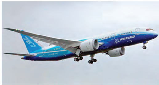
Fig. 15.13 Titanium alloys compose up to 20% of the gross empty weight of the Boeing 787.
