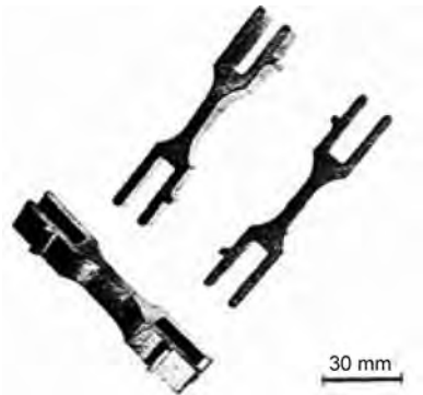
Fig. 8.27 Pressed-and-sintered blended-elemental Ti-6Al-4V connector link arm for the Pratt & Whitney F100 engine. Courtesy of Imperial Clevite Inc.
