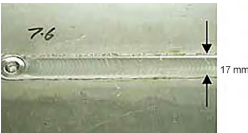
Fig. 12.17 Surface appearance of a friction stir weld in 6.7 mm (0.25 in.) thick Ti-15V-3Al-3Cr-3Sn. Source: Ref 12.18
