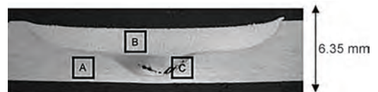
Fig. 12.18 Cross section of an early friction stir welding trial in 6.35 mm (0.25 in.) thick Ti-6Al-4V shows three different weld zones: parent metal (A), deformed surface region (B), and partially transformed weld-root zone containing voids (C). Source: Ref 12.18
