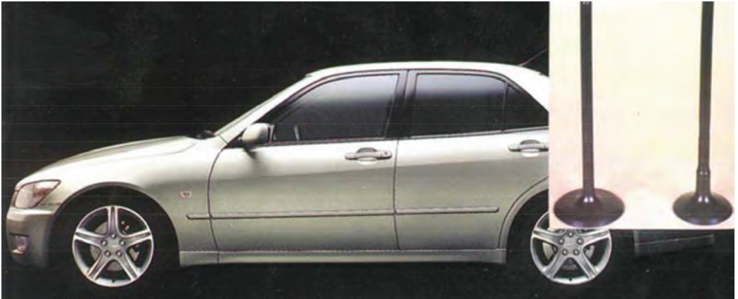
Fig. 8.36 The Toyota Altezza, 1998 Japanese car of the year, was the first family automobile in the world to feature titanium valves. Inset: Ti-6Al-4V intake valve (left) and TiB/Ti-Al-Zr-Sn-Nb-Mo-Si exhaust valve (right). Courtesy of Toyota Central R&D Labs, Inc.
