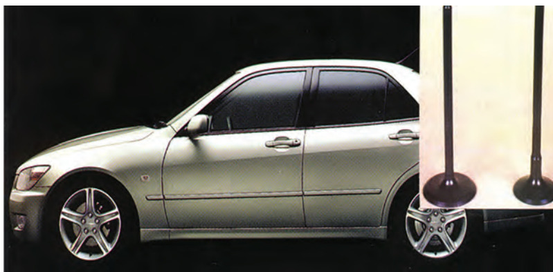
Fig. 15.33 The Toyota Altezza, 1998 Japanese car of the year, was the first family automobile in the world to feature titanium valves. Inset: Ti-6Al-4V intake valve (left) and TiB/Ti-Al-Zr-Sn-Nb-Mo-Si exhaust valve (right). Courtesy of Toyota Central R&D Labs, Inc.
