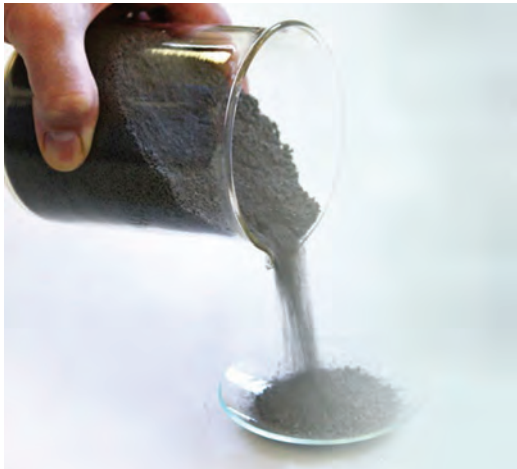
Fig. 1.20 Titanium metal powder suitable for use in near-net shape manufacturing, which produces components that are close to the finished size and shape. Courtesy of J. Barnes, CSIRO, Oct 2013
