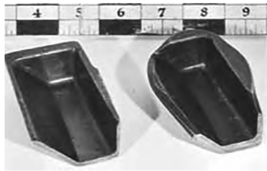
Fig. 10.21 Hammer forging. Left: workpiece forged from the beta field at a temperature of 1150 °C (2100 °F). Right: workpiece forged from the alpha-beta field at 955 °C (1750 °F). The piece on the left is filled. Dies were designed originally for forging aluminum.
