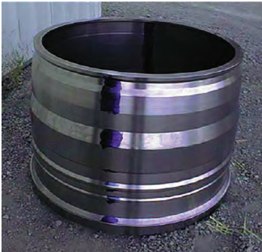
Fig. 8.55 Fan case produced by adding features with additive manufacturing to a forged preform
