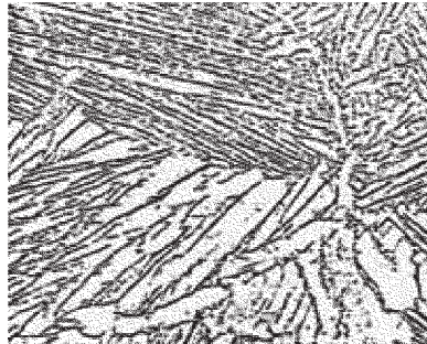
Fig. 7.16 Ti-5Al-2.5Sn billet. Coarse, platelike alpha in billet annealed in the beta field at 1040 °C (1900 °F) for 1 h and furnace cooled. Etchant: 10%HF-5%HNO 3 . Original magnification: 100×
