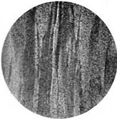
Fig. 10.24 Structure of properly forged material showing distorted beta grain. Etchant: 10%HF-10%HNO 3 -80%H 2 O. Original magnification: 8x
