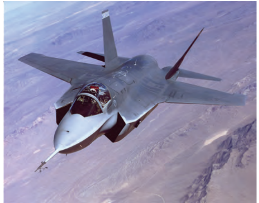
Fig. 15.15 F-35 Joint Strike Fighter with greater than 40% of its structural weight made of titanium
