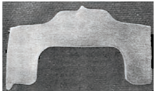
Fig. 10.13 Macrostructure of rolled Ti-6Al-4V ring illustrating the predominantly tangential grain flow
