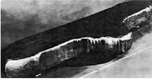
Fig. 10.7 Example of titanium forged in open or flat dies as in blacksmithing (hand forging)
