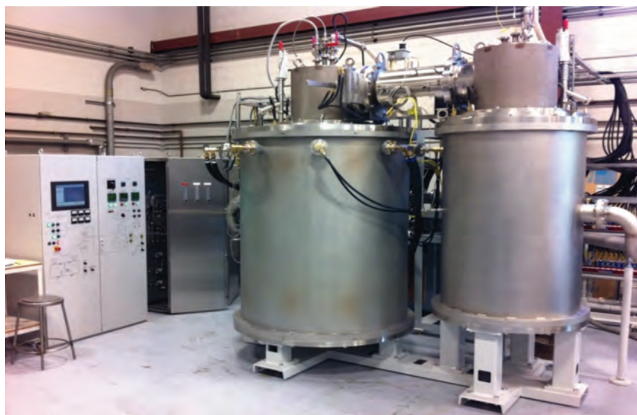
Fig. 8.35 Pilot-scale unit at ADMA Products for manufacturing hydrogenated titanium powder. Annual capacity is 113,400 kg (250,000 lb). Courtesy of ADMA Products Inc.
