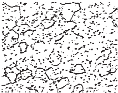
Fig. 7.6 Pure titanium sheet. Equiaxed alpha and beta spheruloids resulted from heating specimen from Fig. 7.4 at 705 °C (1300 °F) for 1 h and air cooling. Etchant: 10%HF-5%HNO 3 . Original magnification: 500×
