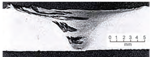
Fig. 12.13 Cross section of a friction stir weld in commercially pure (grade 2) titanium produced at The Welding Institute in 1995. Source: Ref 12.18
