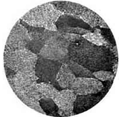
Fig. 10.25 Structure of improperly forged material showing equiaxed beta grain. Equiaxed grains indicate insufficient working after heating in the beta field. Etchant: 10%HF-10%HNO 3 -80%H 2 O. Original magnification: 8x
