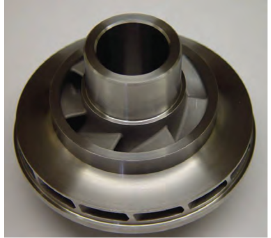
Fig. 8.44 Selectively net shape extralow interstitial Ti-6Al-4V impeller for a rocket engine turbopump. Fabricated using the prealloyed metal can method. Courtesy of Synertech PM Inc./P&W Rocketdyne
