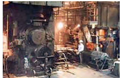
Fig. 9.10 Hot rolling converts slab material into a single longer piece that can be coiled at an intermediate-thickness hot band. Courtesy of Timet
