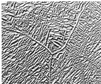
Fig. 10.27 Microstructure of properly processed Ti-13V-11Cr-3Al consisting of uniformly distributed alpha particles. This is a result of working the alloy in the low end of the forging range (<980 °C, or 1800 °F) and aging. This is the structure of the high-ductility material referred to in Table 10.7. Original magnification: 10,000x
