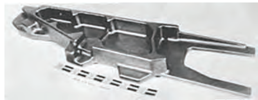
Fig. 10.22 Flat-track forging. Originally of aluminum design, this 18 kg (40 lb) Ti-6Al-4V structural part was forged from the beta field.
