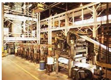
Fig. 9.11 Continuous vacuum annealing is used to process thin strip free from surface contamination. Courtesy of Timet
