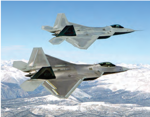
Fig. 15.14 The F-22 Raptor Advanced Tactical Fighter consists of up to 45% Ti alloy by weight.
