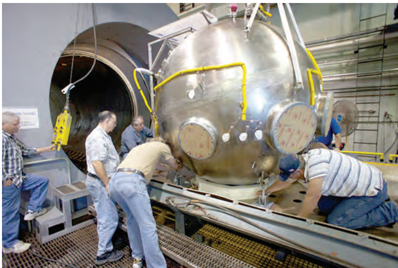
Fig. 15.20 Titanium personnel sphere for the human-occupied submersible Alvin is prepared for pressure testing. Courtesy of Woods Hole Oceanographic Institution
