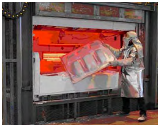
Fig. 11.12 A Ti-6Al-4V component is removed from a 900 °C (1650 °F) furnace after superplastic forming. Courtesy of Aeromet International PLC
