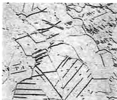
Fig. 5.4 Twinning in high-purity titanium. The twins are the needlelike bands in the grains. In some instances, the twins extend entirely across a grain. Etchant: 10%HF-5% \text{HNO}_3 . Original magnification: 250x
