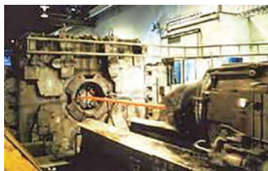
Fig. 9.8 German Fabrication Machines' radial precision forging machine. Courtesy of Timet
