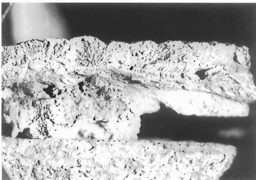
Fig. 19. Fracture surface of ground bar butt weld in sample 1 in single-sided region, close to outboard edge of ground bar. Note smoother fracture surface in weld root, from which some chevron patterns (arrowed) emerge. \times 4 .
