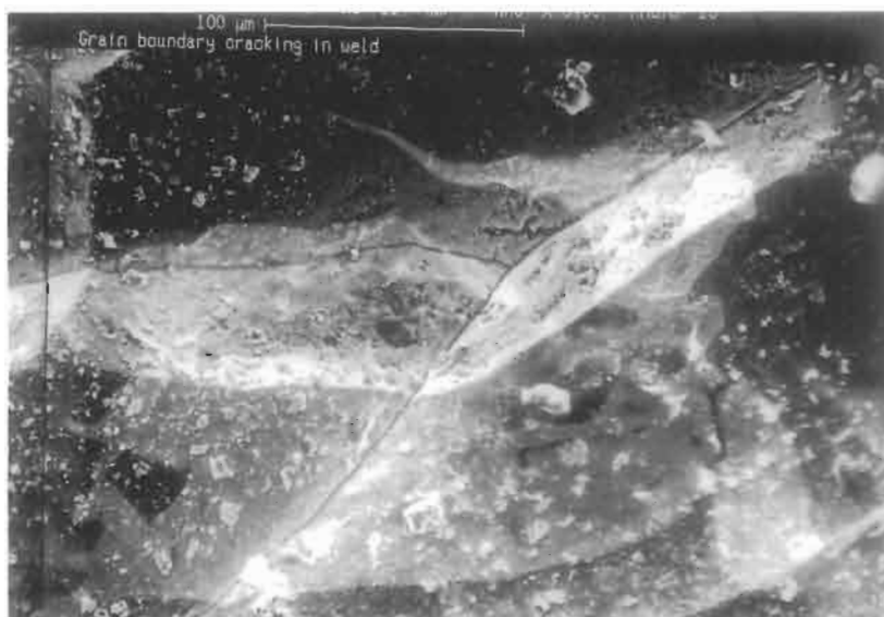
Fig. 7. SEM fractograph of the fracture surface as received. The intergranular nature of the fracture and secondary cracks can be seen.
