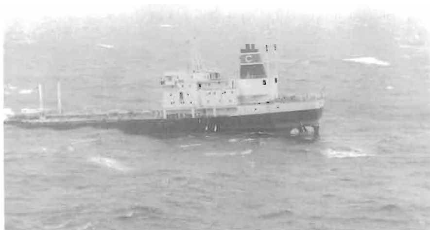
Fig. 4. Stern section of MV Kurdistan after breaking in two.
