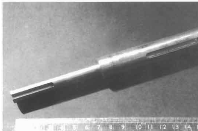
Fig. 5. Wheel shaft with reduced length keyway groove.
