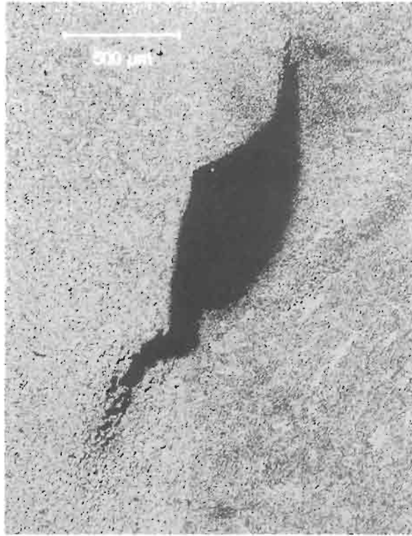
Fig. 9. This lack-of-fusion/slag flaw on the fusion line had extended about 500 \mu\text{m} by creep. Where it grew into the HAZ, it grew into fine-grained material, and there was a very high density of creep rupture voids. (The darker material on the right is weld metal.) (Nital etch, bright field.)
