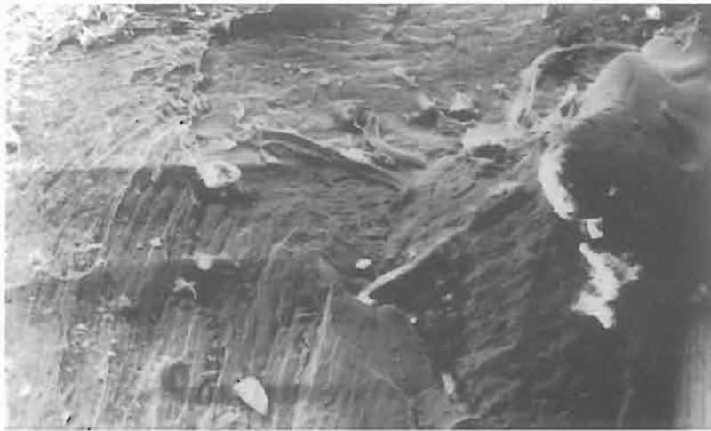
Fig. 6. Scanning electron micrograph taken from the shear part of the failure. Magnification: 153 times.
