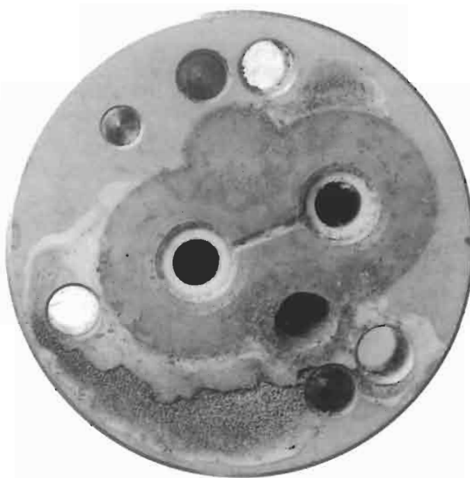
Fig. 2. Crevice corrosion suffered by the 316L stainless steel pump. Small crystals of sodium chloride can be seen on and around the corroded area.
