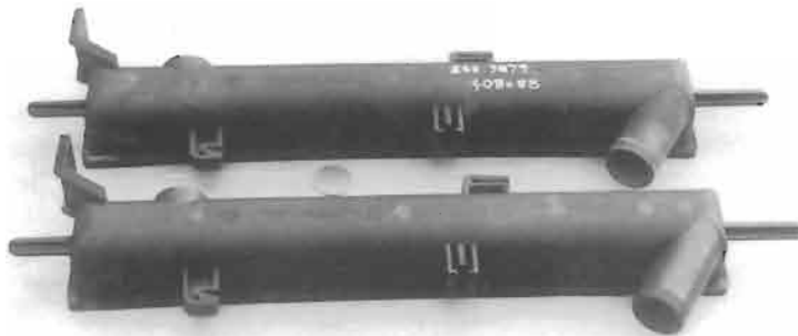
Fig. 1. Failed and new radiator boxes compared. The upper, failed sample cracked after 500 miles in service.
