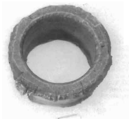
Fig. 4. Photograph of failed sight port flange.
