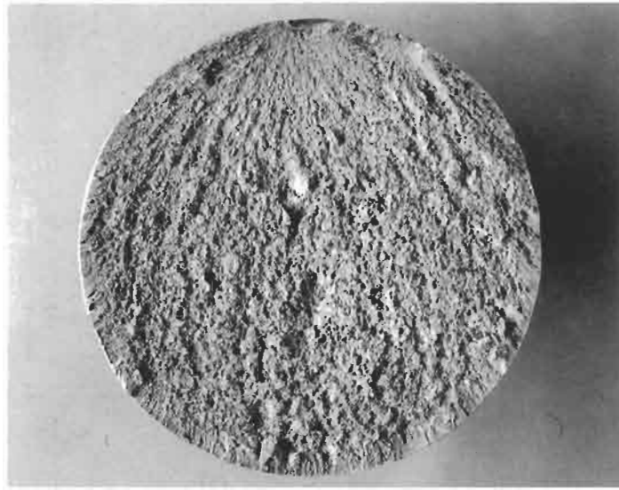
Fig. 2. Fracture surface of a broken bar.
