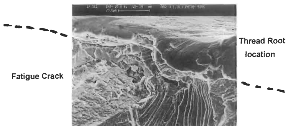
Fig. 2. Fatigue initiation site at thread root location.
