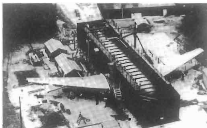
Fig. 2. Aerial view of Comet G-ALYU in testing tank. Crown Copyright. Reproduced with the permission of the Controller of HMSO.
