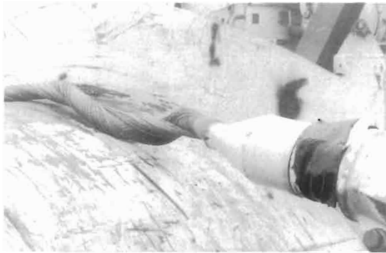
Fig. 8. Characteristic damage induced in spiral strand by pulling out a hockle or kink.
