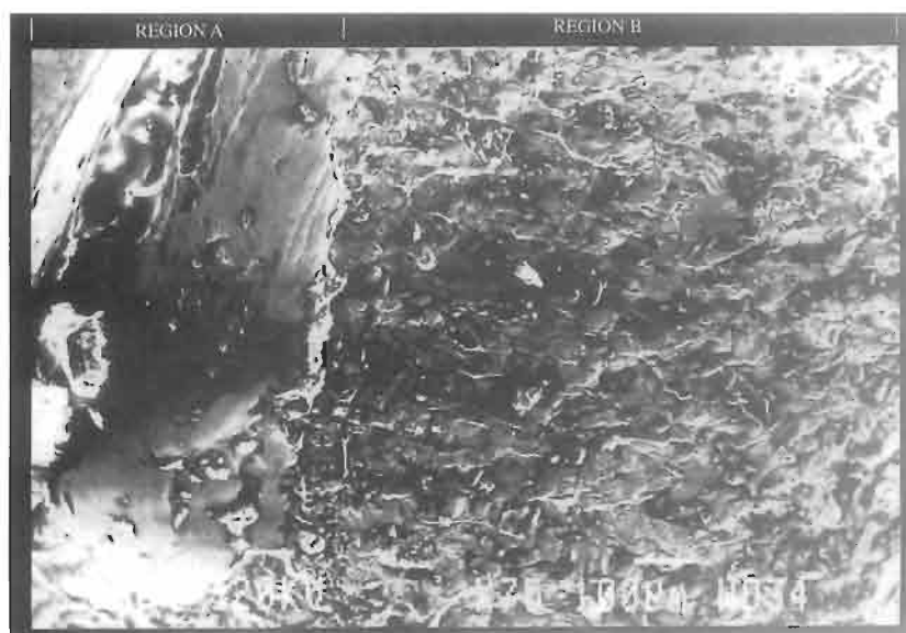
Fig. 4. Fracture surface taken close to the outer layer of the tubing.
