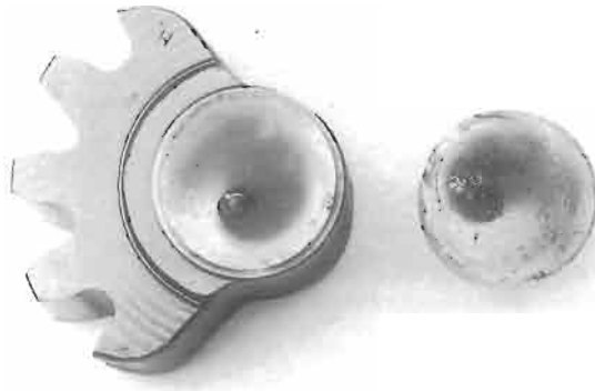
Fig. 5. Photograph of the matching fracture surfaces.
