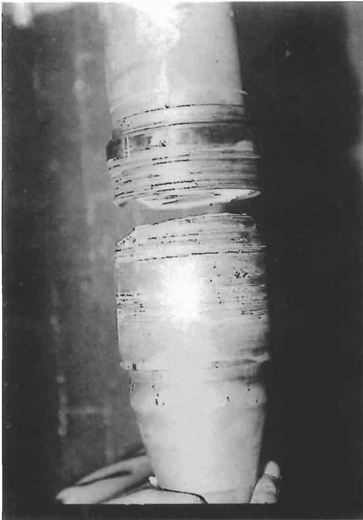
Fig. 2. Photograph of the failed shaft and chromium-plated sleeve.
