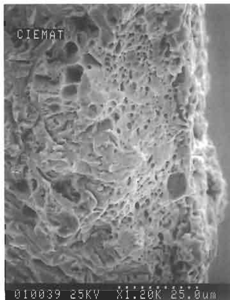
Fig. 11. Fracture surface of the failed chromium-plated sleeve (I.D.).
