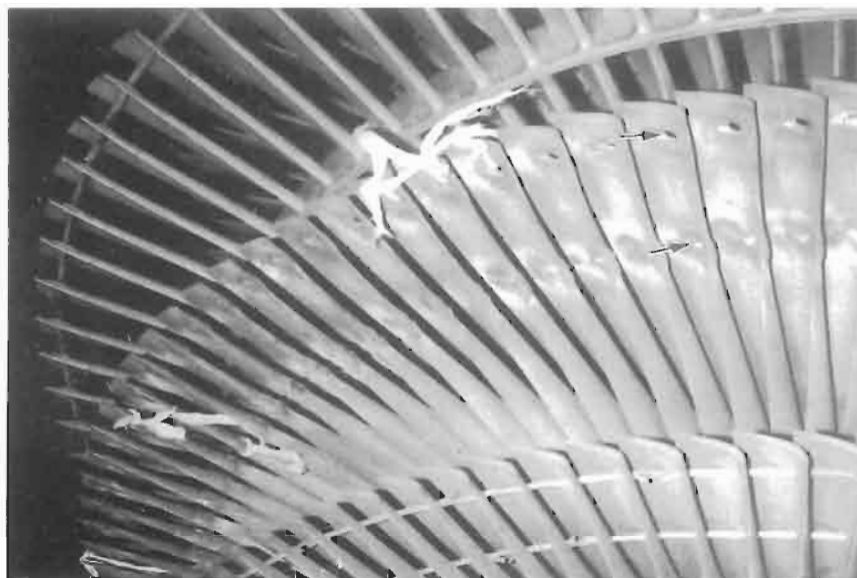
Fig. 1. Photograph showing the assembly of the blade without the lacing wire which has been removed by debrazing. Arrows indicate the position of lacing holes from where crack initiation occurred.
