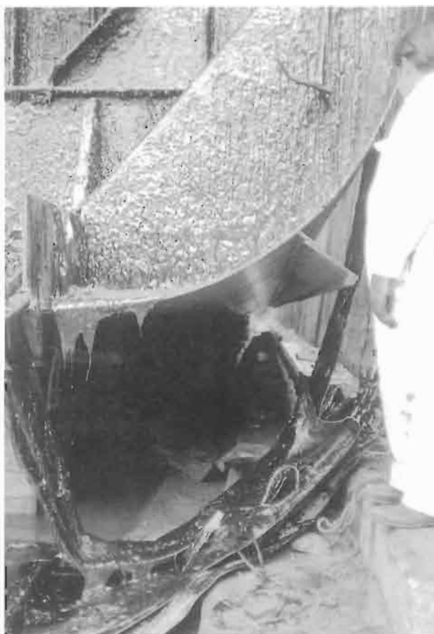
Fig. 9. Port bilge keel showing bilge bracket: also showing longitudinal.
