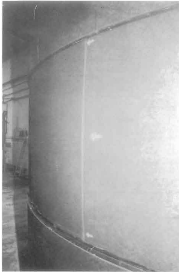
Fig. 3. Face view of the failed weld in the plastic panels of the tank. The large white arrow indicates the position of the crack initiation point in the centre of the weld, the crack eventually widening to the points shown by the two smaller arrows. The surface surrounding the failed weld is pristine and totally undamaged, with no abrasive wear or traces of impact damage.
