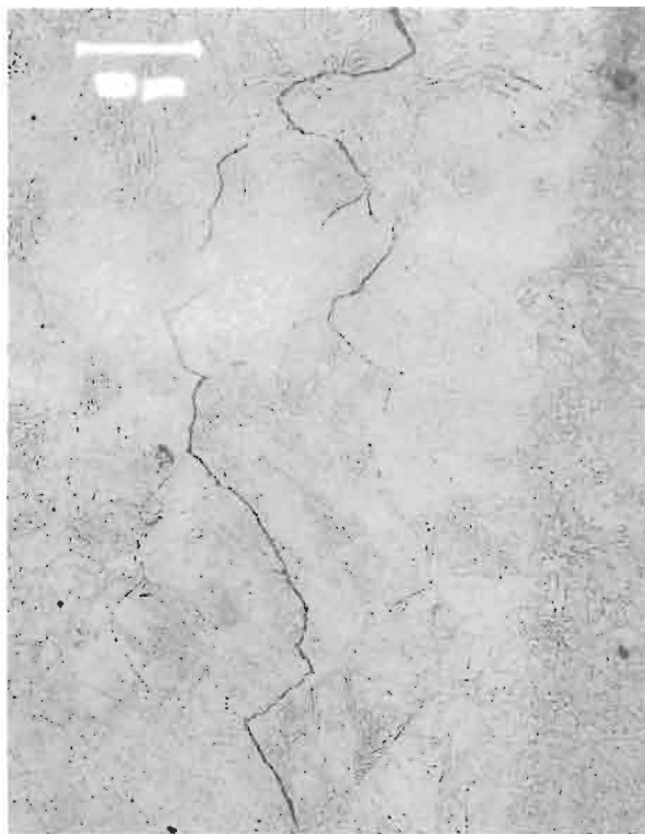
Fig. 5. Cracking on the 8 in. line side of the Y-side connection to the steam chest. The darker band to the right is weld metal. (Photomicrograph taken from a replica made in the cavity produced by removing a boat sample.) (Nital etch, bright field, cellulose acetate replica.)
