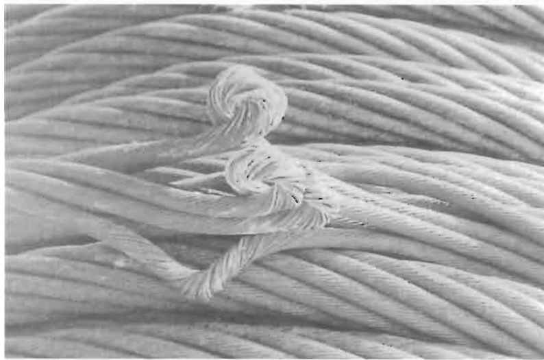
Fig. 5. Hockles formed in the individual strands of an eight strand work wire.
