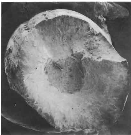
Fig. 6. SEM photograph of a specimen with Corr. d. = 2, with a reduced fibrous zone, and increased brittleness of the shear-lip zone. \times 13 .
