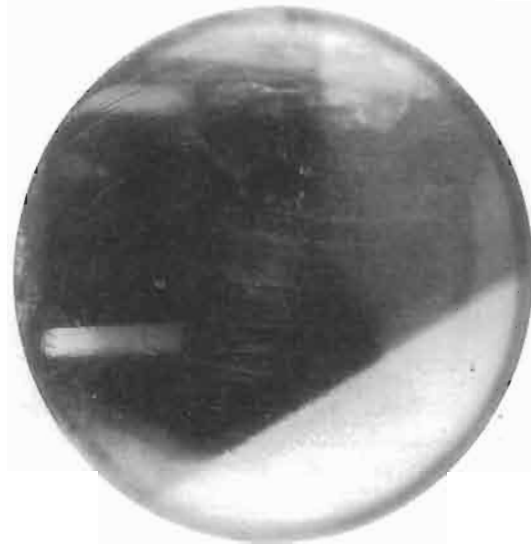
Fig. 8. Polished cross-section through the shaft, showing the case-hardened layer.
