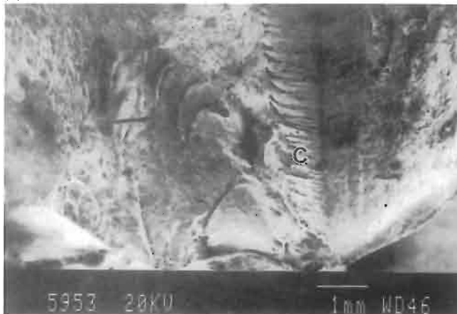
Fig. 4. (a) Crack initiation points marked by arrow head in optical micrograph; (b) SEM fractograph taken from area marked as 'X' in Fig. 4(a); (c) SEM fractograph from area marked as 'Y' in Fig. 4(a). Arrows indicate crack growth directions (dark line at the centre indicates the cut-mark along which fracture surface was cut into two pieces for SEM observation).
