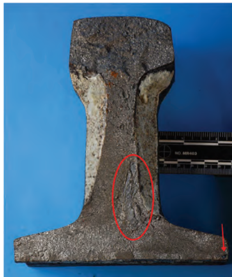
Fig. 99 Rail fracture surface. Circle indicates fracture initiation, and arrow indicates void
