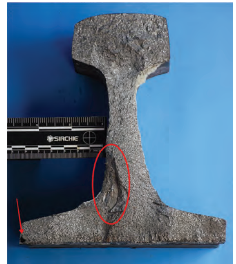
Fig. 100 Mate fracture surface. Circle indicates fracture initiation, and arrow indicates void
