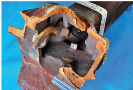
Fig. 89 Overall view of the fracture face. Arrow indicates deformation at crack shown in Fig. 88
