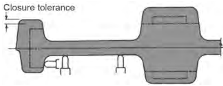
Fig. 18 Illustration of a closure error where the dies have not been brought together to the appropriate thickness dimension
