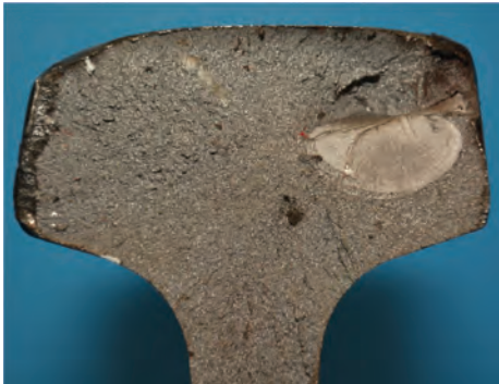
Fig. 94 Subsurface fatigue fracture surface initiating from field side of rail head. No discoloration indicates the crack was not open to the atmosphere
