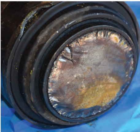
Fig. 30 Fractured axle journal within bearing. The end cap was removed from the failed side. A noticeable amount of red rust was present on the interior of the end cap, as seen in Fig. 32. The journal stub was pressed out of the bearing. Present on the end of the journal was the axle fabrication data, shown in Fig. 33. The axle was manufactured by Standard Forged Products, McKees Rocks Forgings of McKees Rocks, Pennsylvania, in June 1990
