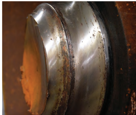
Fig. 18 Failed journal after cleaning at initiation site, with mechanical damage present
