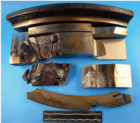
Fig. 74 Analyzed rim section showing fracture locations and macroetch performed on a section
