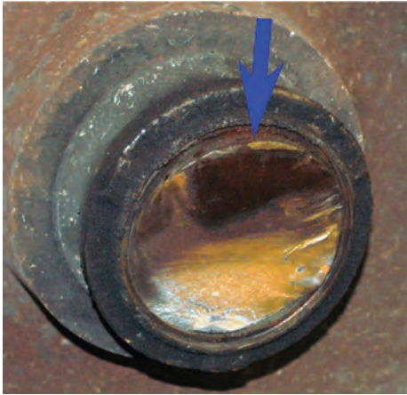
Fig. 5 Axle 1 wheel and backing ring in place. Arrow indicates fracture-initiation site
