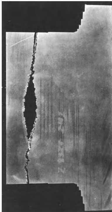
Fig. 15 Section through a heat-resistant alloy forging showing a central discontinuity that resulted from insufficient homogenization during conversion. Step machining was used to reveal the location of the rupture; original diameter is at right.
