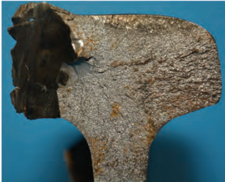
Fig. 95 Mating fracture surface of Fig. 94. Note the damage caused by postfracture wheel impact
