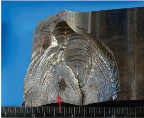
Fig. 78 Opposite fracture surface. Arrow indicates initiation location
