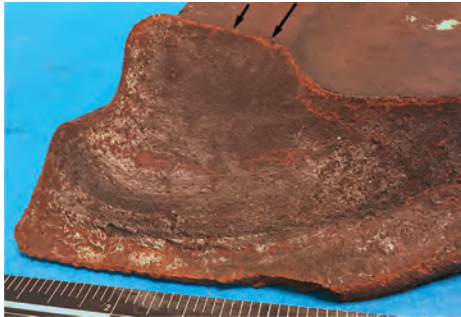
Fig. 116 Close-up view of fatigue fracture surface with beach marks. Arrows indicate the initiation-site areas
