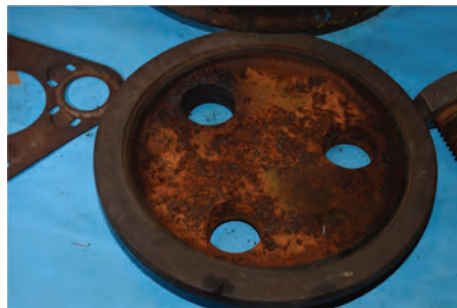
Fig. 32 Inside of subject bearing end cap
