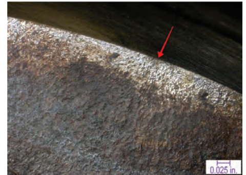
Fig. 21 Fracture-initiation location indicated by arrow
