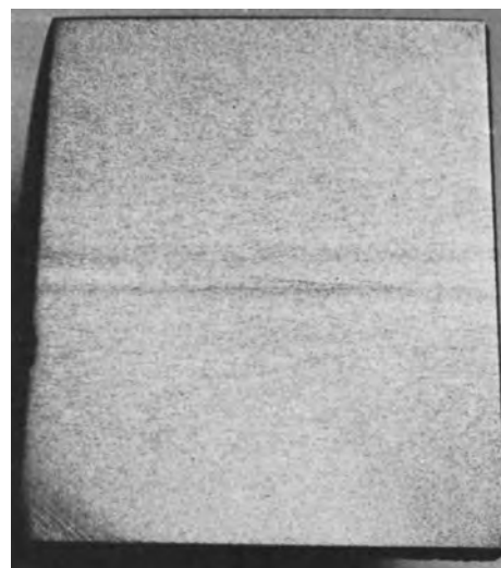
Fig. 2 Longitudinal section through a hot rolled 1041 steel bar showing a carbon-rich centerline (dark horizontal bands) that resulted from segregation in the ingot. Picral etch. Original magnification: 3 \times . Courtesy of J.R. Kilpatrick
