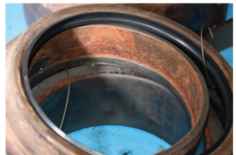
Fig. 34 Seal wear ring (inverted) below seal housing. Fretting wear can be seen on the inner cone at the bottom of the stack. The fractured journal was also cleaned in mineral spirits and then cut approximately 25 mm (1 in.) from the fracture surface. This was performed to enable the area adjacent to the fracture to be inspected. Prior to inspection with a digital light microscope, the section was soaked in Evapo-Rust to remove the tightly adhering red rust adjacent to the fracture surface, as seen in Fig. 35. An example of the surface condition of the axle is shown in Fig. 36. The fracture is to the viewer's left, and the concentric lathe tool cutting marks can be seen as vertical parallel grooves farther to the right of the pitting
