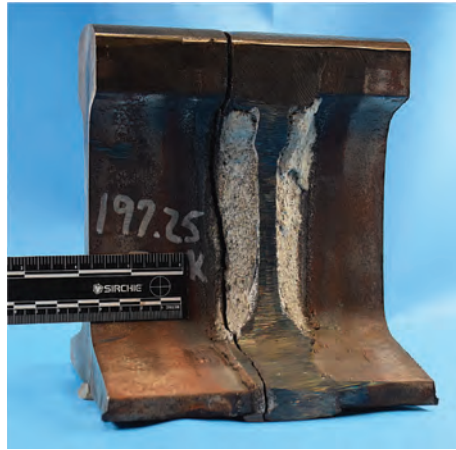
Fig. 97 Overall view of failed weld in the as-received condition
