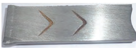
Fig. 14 Centerline chevron cracks in an extruded bar. Courtesy of Bharat Forge Limited, Pune, India
