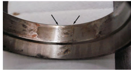
Fig. 7 Black arrows indicate galling damage. Note the fretting discoloration at right and left
