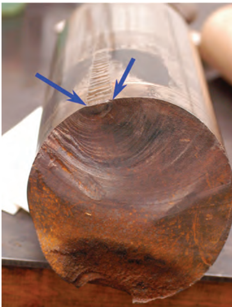
Fig. 6 Derailment 2. Arrows indicate boundary of galling damage and fracture-initiation location
