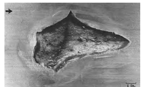
Fig. 16 Cross section of a forged bar showing a forging burst. The burst is located approximately at the centerline of the workpiece. Arrow indicates the direction of working.
