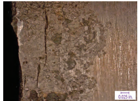
Fig. 39 Secondary fatigue cracks present near primary fracture surface
