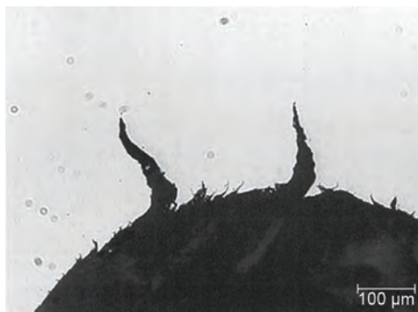
Fig. 34 Metallographic image of intrados cracks in compressed and released nitinol wire sample. Cracks initiate in shear during compression and grow in tension upon release
