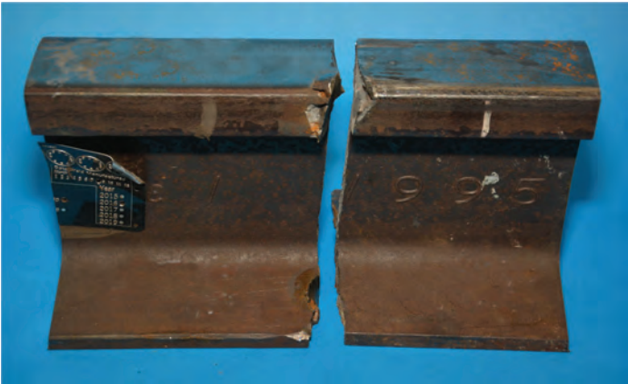
Fig. 93 Mating fracture surfaces with thumbnail fatigue fracture from field-side corner of rail head. Black tag is a partial record of rail weld not included
