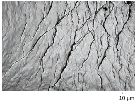
Fig. 32 SEM image of compression-induced cracks in a nitinol wire sample subjected to 50% strain
