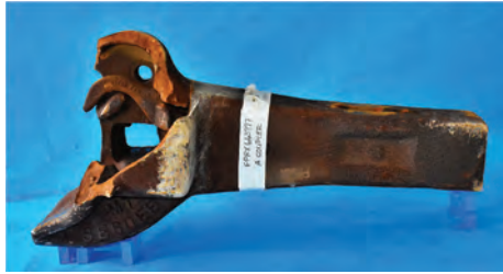
Fig. 87 As-received failed coupler
