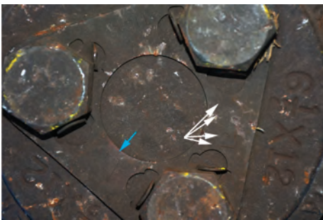
Fig. 31 Cap screw locking plate. Blue arrow indicates "N" for new, while white arrows indicate month and year (December 1990)
