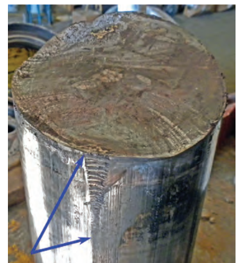
Fig. 3 Initiation site of fracture surface is indicated by larger blue arrow. Beginning of galling damage is indicated by smaller blue arrow
