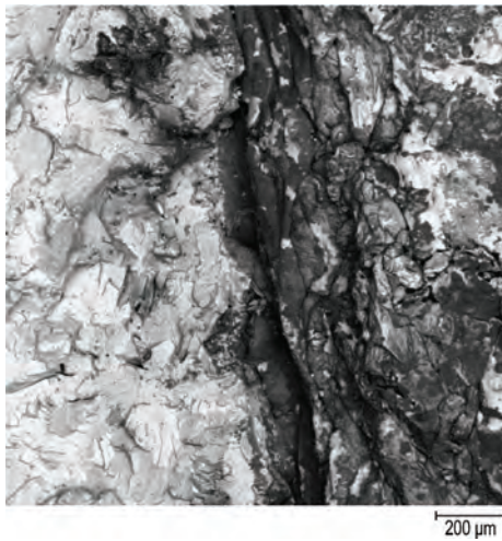
Fig. 107 Backscatter image. Left side of image is base metal; right side is the defect area. Original magnification: 116×
