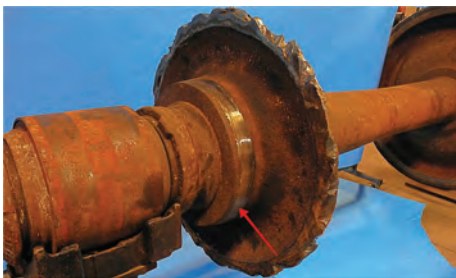
Fig. 52 Hub and partial plate section of failed wheel. Arrow shows the wear from riding on the rail
