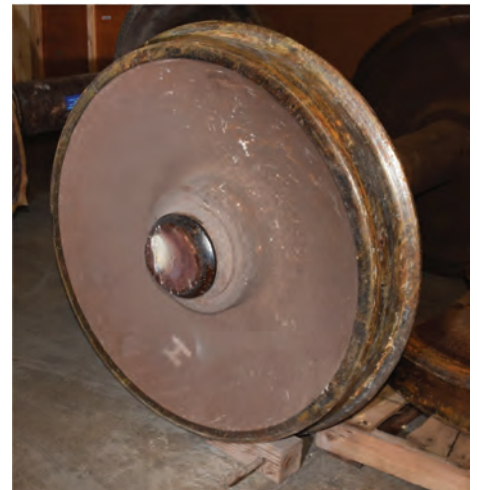
Fig. 27 Overall view of failed axle journal. The locking plate data are stamped on both bearings to provide information to the bearing installer as to whether the bearing is new or reconditioned, including the month and year of installation. In this case, it was found that the bearing had been installed in new condition in December 1990 by Trinity 54 in Dallas, Texas. These notations are shown in Fig. 31
