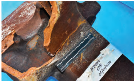
Fig. 88 View of cracking, which caused the thrower to be trapped
