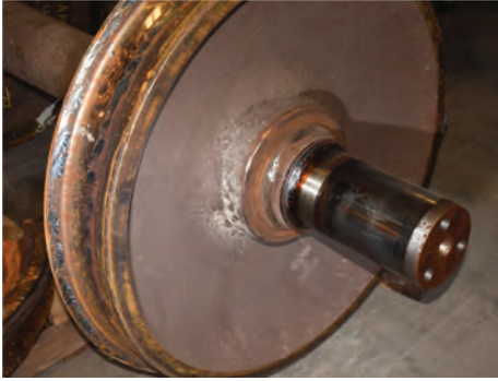
Fig. 29 Mating side of axle with bearing removed. The failed journal was still within the bearing assembly, as seen in Fig. 30. A distinct population of ratchet marks is observable around the circumference of the fracture surface. The ratchet marks indicate the combination of crack planes
