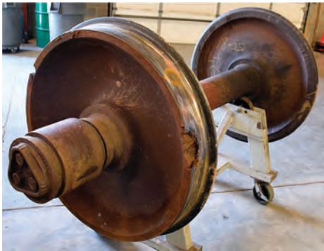
Fig. 62 As-received wheelset with damage present to the running surface
