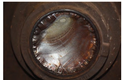
Fig. 28 Fracture surface on axle side. Note that the backing ring remains in place on the axle due to the fitted backing ring
