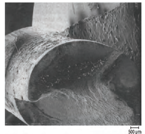
Fig. 11 The fatigue crack area (top) and overload location (below) with some minor corrosion residue
