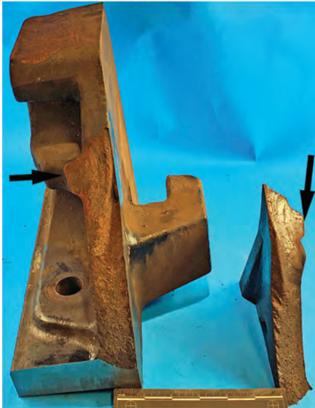
Fig. 115 Fracture surface opened. Black arrows correspond to crack-initiation sites on the mating fracture surfaces
