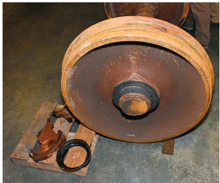
Fig. 11 As-received axle showing fracture surface
