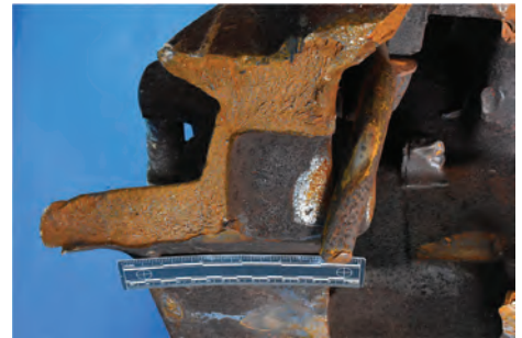
Fig. 91 Fracture surface to the left in Fig. 89. Overload failure
