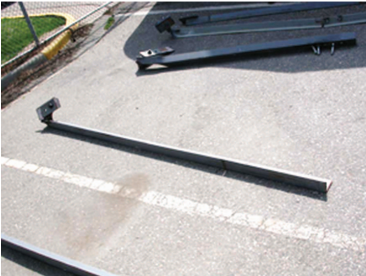
Figure 4-2. Post-accident photograph of one of the angle-shaped steel braces used to brace the collapsed girder.
