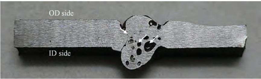
Fig. 6.160 Macrostructure showing longitudinal section view across the weld. The weld shows numerous porosities and through and through crack joining the undercuts from both sides.
