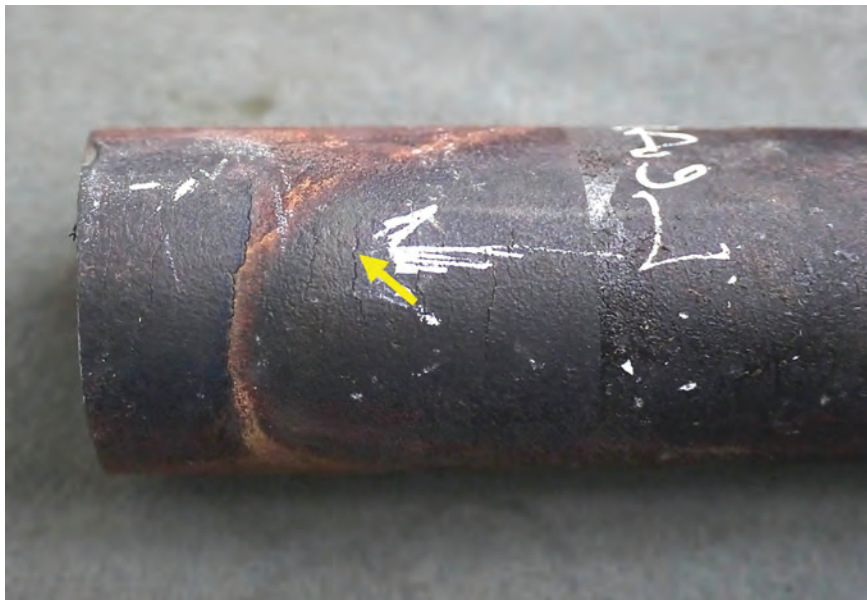
Fig. 6.140 Close-up view of a tube at leakage location revealing fine multiple and parallel cracks in transverse (circumferential) direction
