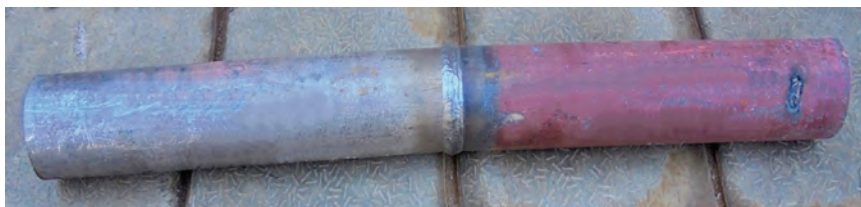
Fig. 6.45 Typical dissimilar metal weld joint
