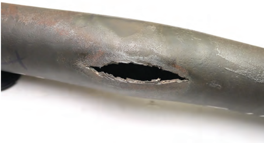
Fig. 6.12 Reheater tube sample showing bulging and bending at failure location with thick-lip fish-mouth rupture
