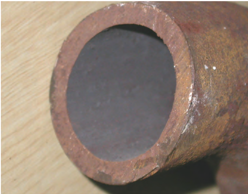
Fig. 6.146 (a) Weld joint with a hairline crack on weldment. (b) ID surface view showing tightly adherent smooth black scale
