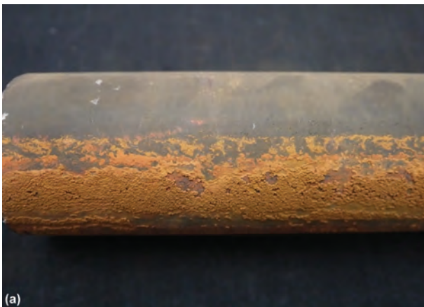
Fig. 6.28 (a) Dark brown scale on OD surface. (b) Brownish black scale on the ID surface of a tube
