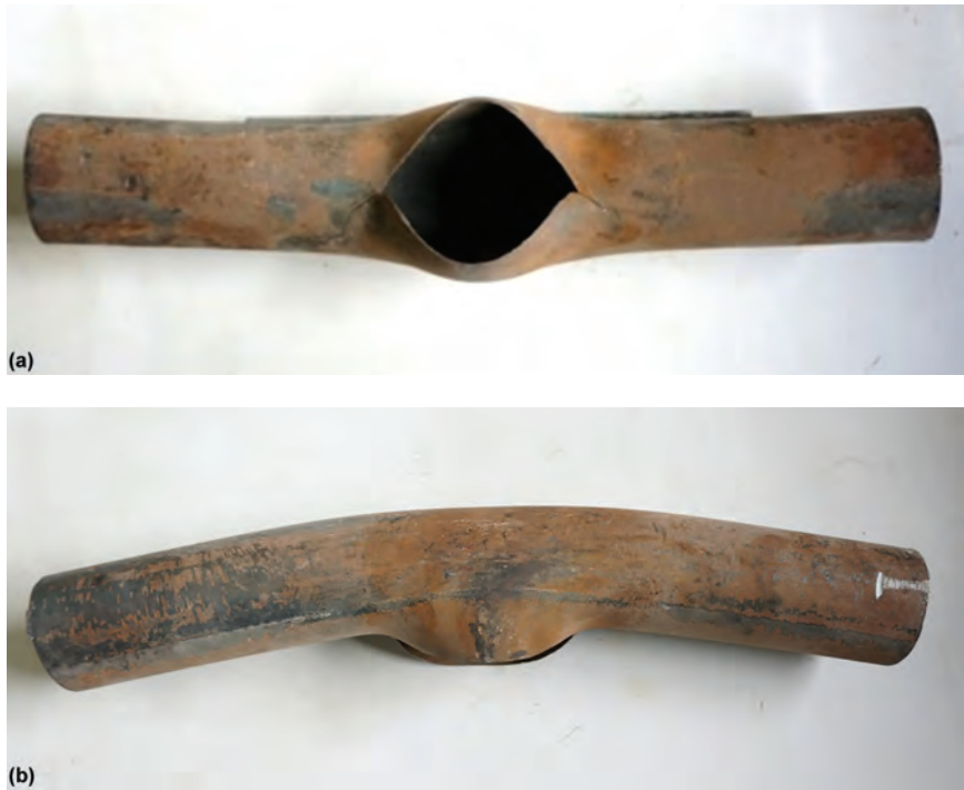
Fig. 6.17 Close-up views of the failed screen tube showing (a) thin-lip fish-mouth fracture and (b) bulging and bending of the tube
