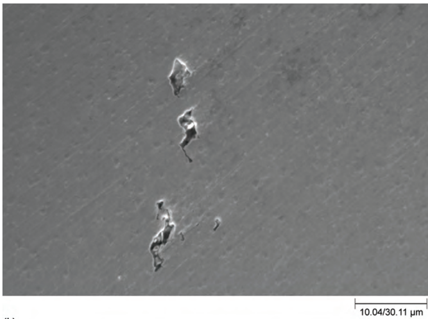
Fig. 6.15 (a) SEM fractograph showing presence of creep voids on fracture lip surface, 500 \times ; and (b) SEM image of as-polished sample after metallography showing scattered creep voids, 1000 \times
