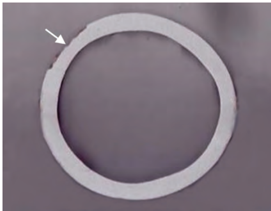
Fig. 6.115 Transverse cross section of a tube in macroetched condition. It shows the seamless nature of the tube with metal wastage due to corrosion on outer surface.
