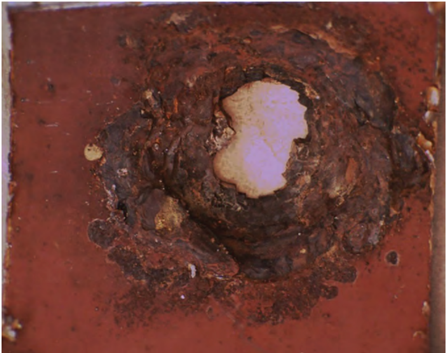
Fig. 6.67 Rounded pit formed due to phosphate corrosion
