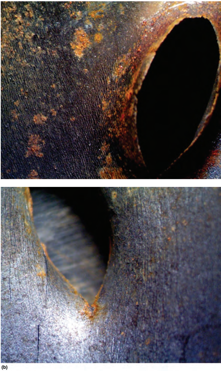
Fig. 6.133 Low-magnification view of (a) outer surface indicating corrosion and erosion marks, 6×; and (b) inner surface surrounding the puncture with scale, 6×
