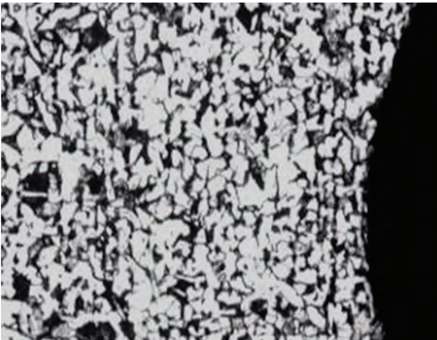
Fig. 6.76 Microstructure of an ID-side bend sample, 200×
