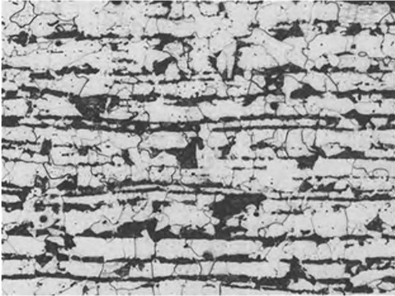
Fig. 5.7 Microstructure of steel showing pearlite banding
