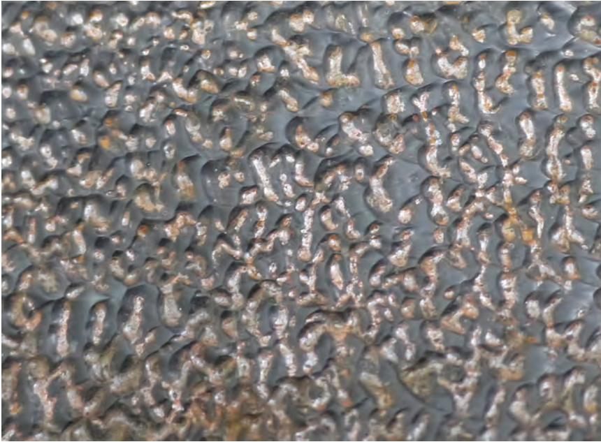
Fig. 6.75 Internal surface of a tube at extrados portion displaying scalloping marks at low magnification, 11×
