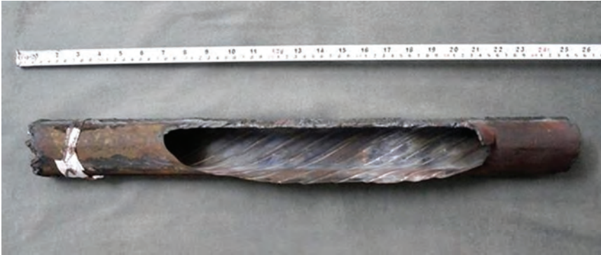
Fig. 6.49 Window-type fracture in waterwall tube due to hydrogen damage
