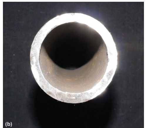
Fig. 6.28 (a) Dark brown scale on OD surface. (b) Brownish black scale on the ID surface of a tube
