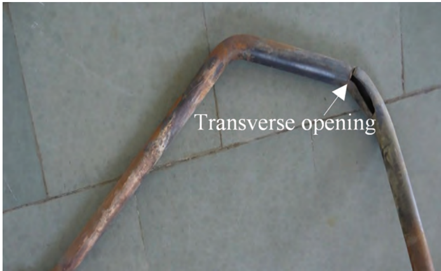
Fig. 6.137 Portion of a failed superheater tube showing failure location
