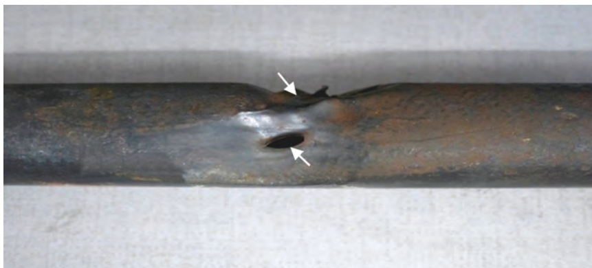
Fig. 6.132 Failed tube showing brownish black scale and two punctures side by side, radially approximately 90° apart
