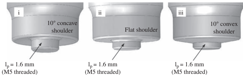
Figure 3.2 Schematic illustrating the three shoulder profiles used to produce friction stir spot weld in aluminum 5754-O sheets [3].
