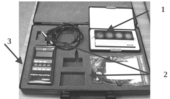
Fig. 36. Complete equipment for measuring the ferrite content, 1 - calibration standards, 2 – connecting cable, 3 - ferritescope [4]
