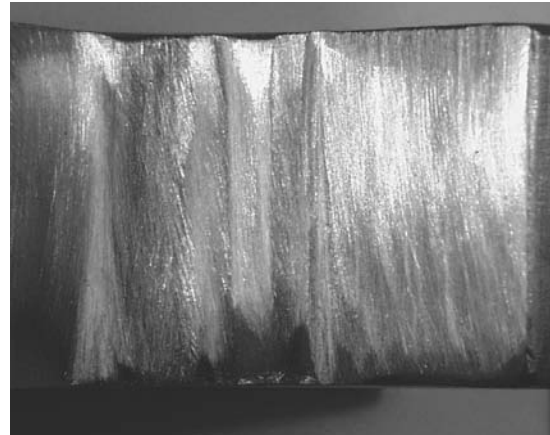
Fig. 29. Macrostructure of the weld after corrosion test; heat input 3.0 kJ/mm; no pitting corrosion [3]
