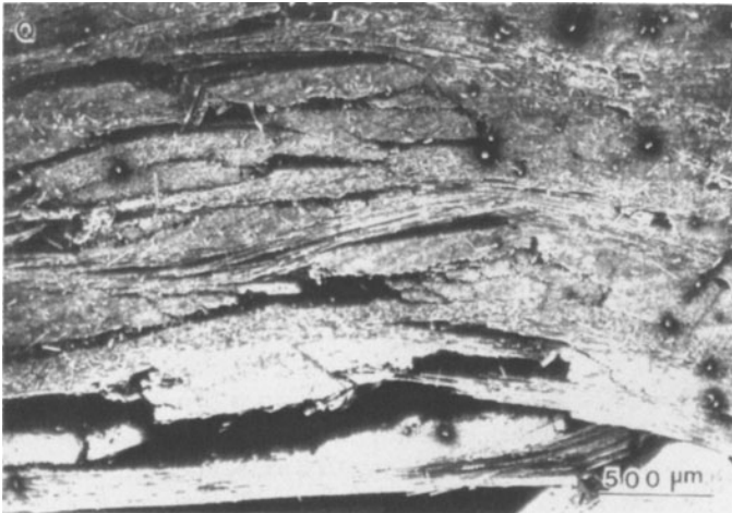
Figure 4.2-6 In-situ three point bend loading of a carbon-carbon laminate in SEM chamber.
