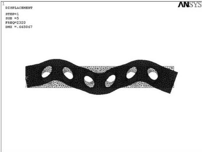
ANSYS graphics shows the beam before and after deformation
