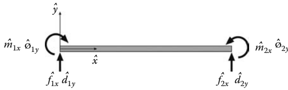
FIGURE 2.5 Beam element subjected to forces and moments.
