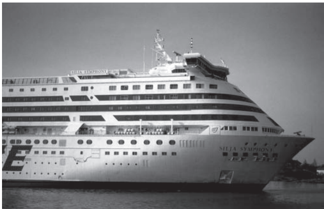
Fig. 3.10 Cruise ship superstructures make good use of aluminum sheet, plate, and extruded shapes. Source: Ref 3.18
