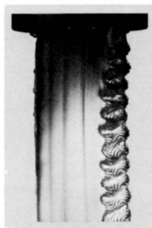
Figure 5.7 Surface distortion on a parison used in blow molding
