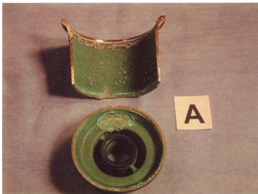
FIGURE 9.7 Half section of die-cast brass water meter body with fracture around base due to dezincification.
