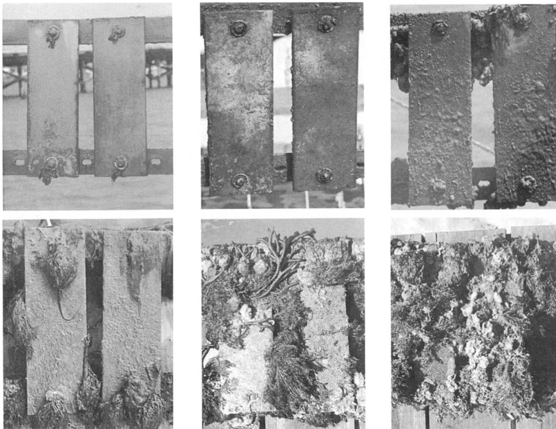
FIGURE 13.3 The 5-year sequence of fouling on 90/10 Cu-Ni in seawater (exposure periods from left to right): (top) 3 months, 9 months, 18 months; (bottom) 36 months, 48 months, 60 months. 1 (See color section.)
