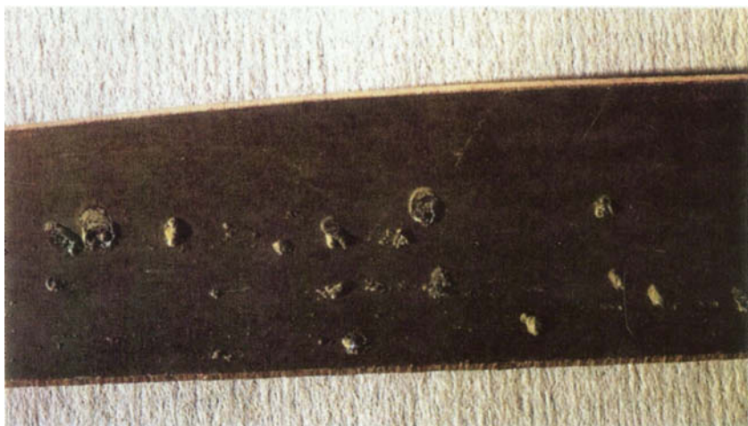
FIGURE 5.7 Typical appearance of Type II pitting. (Photograph courtesy of H.S. Campbell.)
