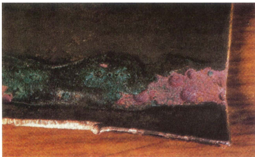
FIGURE 5.9 Typical appearance of Type III pitting. (Photograph courtesy of H.S. Campbell.)
