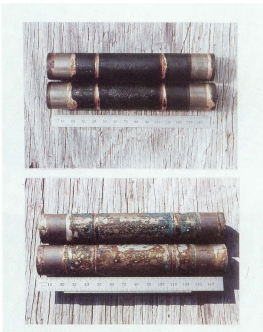
FIGURE 6.2 Appearance of 70/30 copper-nickel tubes with O-ring crevices after one and three cycles of 500 hours in flowing seawater followed by 500 hours of stagnant seawater. (Photographs courtesy of R.M. Kain.)
