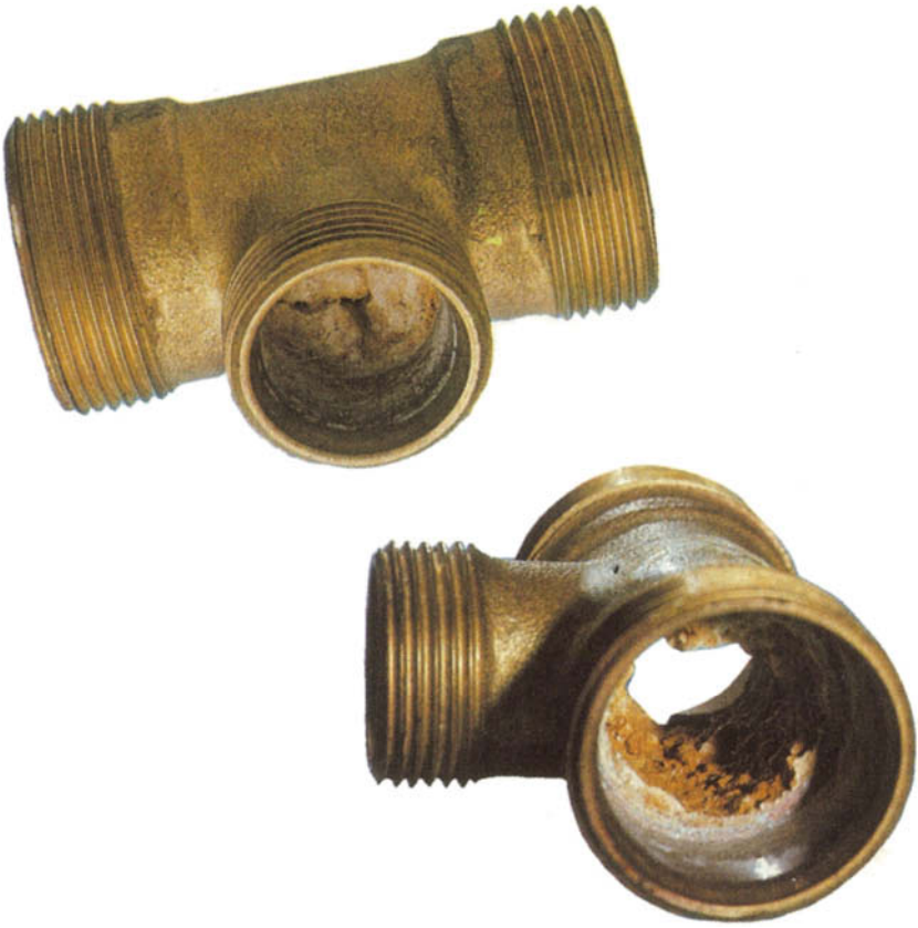
FIGURE 9.1 Meringue dezincification blocking a duplex brass fitting. (Photograph courtesy of Copper Development Association U.K.)
