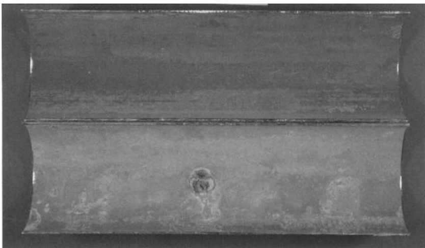
FIGURE 5.3 Type I pitting in a water with high phosphate. (Photograph courtesy of P. Munn.) (See color section.)
