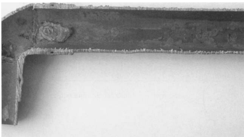
FIGURE 5.2 Type I pitting at a solder flux run. (Photograph courtesy of P. Munn.) (See color section.)
