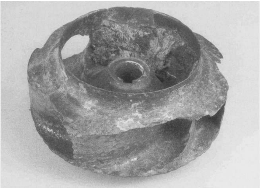
FIGURE 7.29 Severe erosion of a gunmetal impeller due to a high level of suspended solids. (See color section.)
