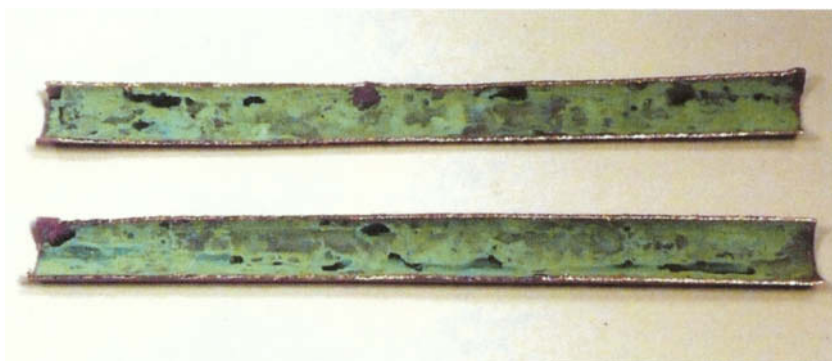
FIGURE 4.7 Appearance of films on copper tube exposed in a cuprosolvent water.
