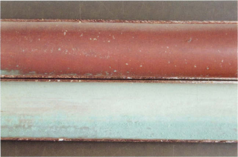
FIGURE 4.9 Appearance of a copper tube carrying so-called blue water. (Photograph courtesy of P. Munn.)
