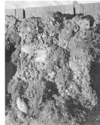
FIGURE 13.4 The 5-year sequence of fouling on 70/30 Cu-Ni in seawater (exposure periods from left to right): (top) 3 months, 9 months, 18 months; (bottom) 36 months, 48 months, 60 months. 1 (See color section.)
