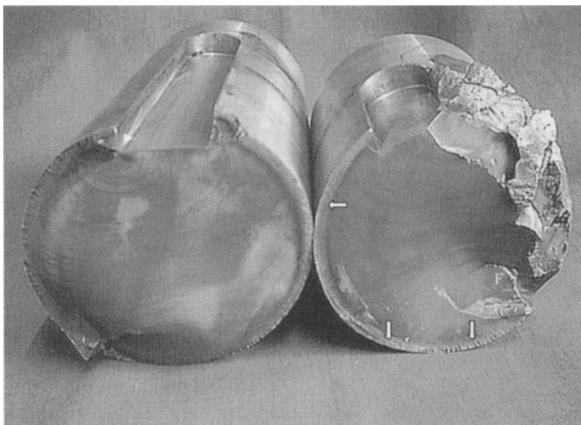
FIGURE 11.2 Typical appearance of a fatigue fracture, including beach marks. (See color section.)
