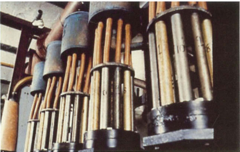
FIGURE B.3 Campbell condenser tube rigs at BNF test site.
