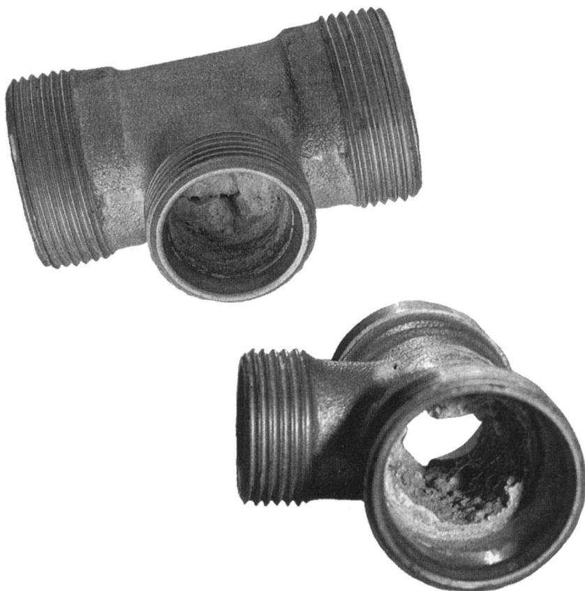
FIGURE 9.1 Meringue dezincification blocking a duplex brass fitting. (Photograph courtesy of Copper Development Association U.K.) (See color section.)
