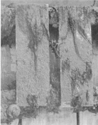
FIGURE 13.4 The 5-year sequence of fouling on 70/30 Cu-Ni in seawater (exposure periods from left to right): (top) 3 months, 9 months, 18 months; (bottom) 36 months, 48 months, 60 months. 1 (See color section.)
