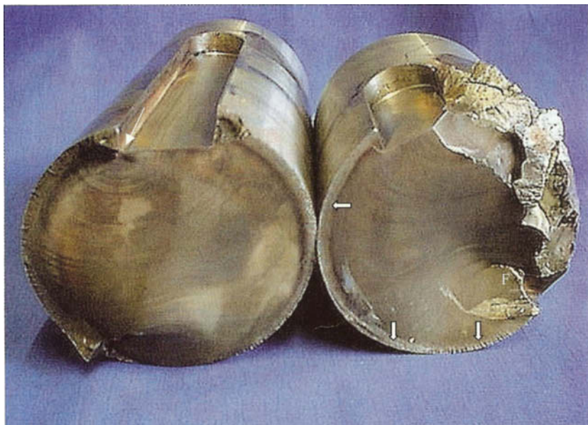
FIGURE 11.2 Typical appearance of a fatigue fracture, including beach marks.
