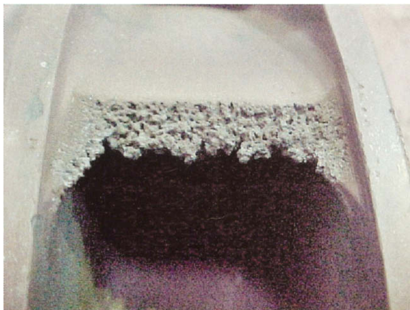
FIGURE 8.1 Cavitation damage, showing typical jagged, honeycomb appearance.
