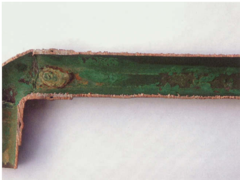
FIGURE 5.2 Type I pitting at a solder flux run. (Photograph courtesy of P. Munn.)
