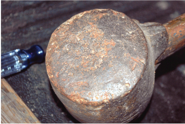
COLOR FIGURE 6.3 Impact wear on a cast iron post-driving maul.
