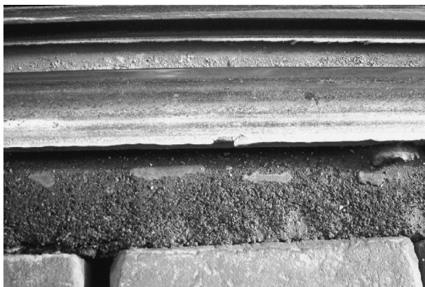
FIGURE 5.4 The frosted area on this roller (25 mm major diameter) was caused by micropitting fracture of microscopic particles from the rolling surface.
