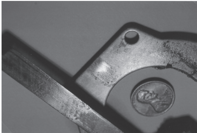
FIGURE 3.13 (See color insert.) Polishing wear of hard steel saw components after years of service.
