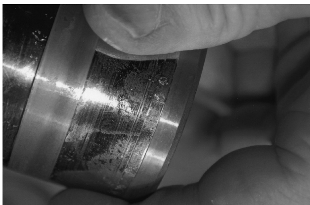
FIGURE 5.6 (See color insert.) Spalling of a hardened steel rolling surface for cam followers.
