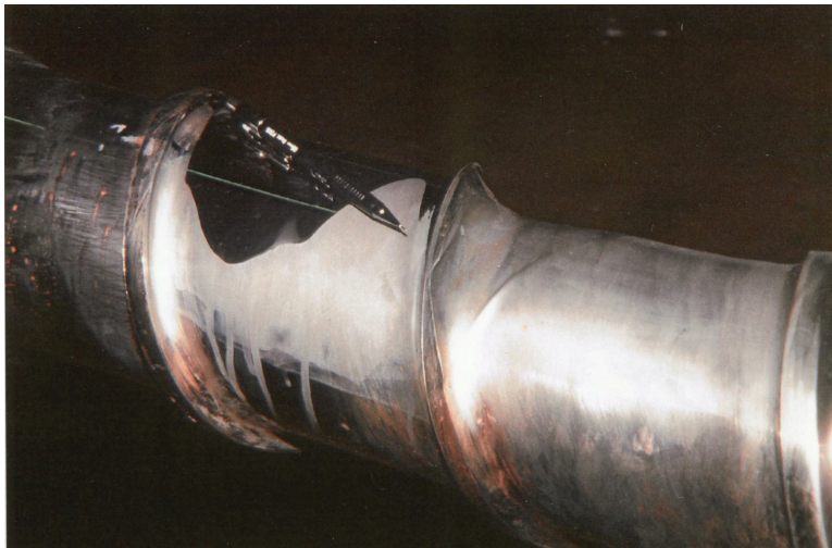
COLOR FIGURE 8.3 Abrasion of flights at the inlet section of a polyester extruder after introduction of carbon black into the melt. The screw was etched to show how the chromium plating had been removed. The flights were 12 mm wide to start, and the eroded width was as low as 2 mm.
