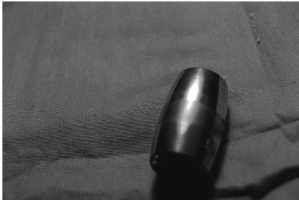
FIGURE 5.4 The frosted area on this roller (25 mm major diameter) was caused by micropitting fracture of microscopic particles from the rolling surface.
