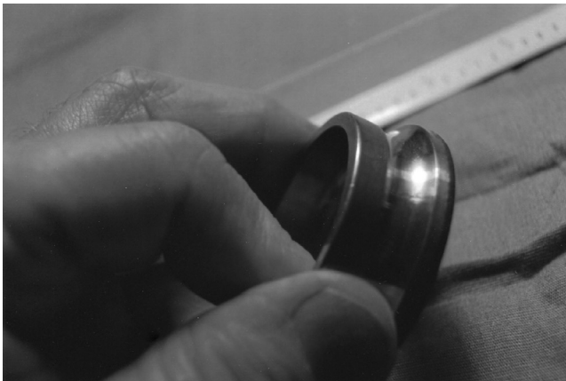
FIGURE 5.8 (See color insert.) Brinelling of a raceway from static overload.
