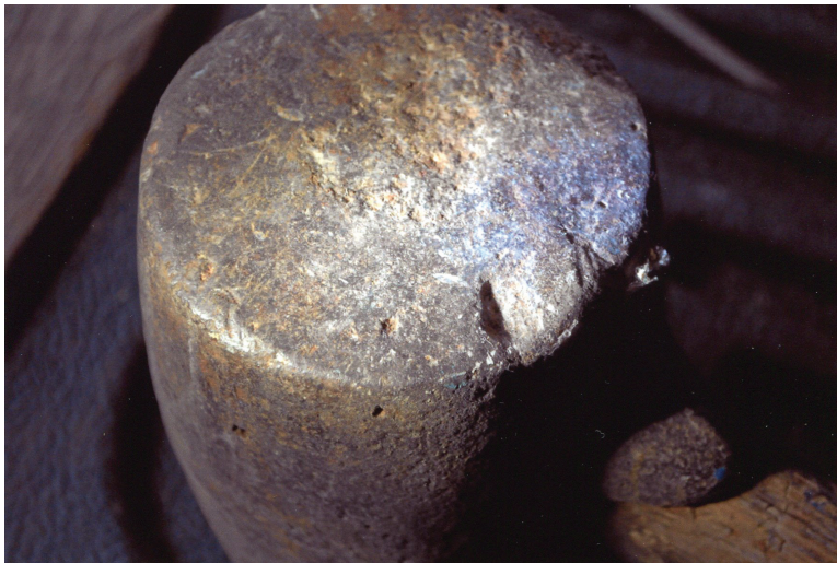
COLOR FIGURE 6.4 Impact wear on the same maul (other end) that was used on steel posts—spalling occurred.
