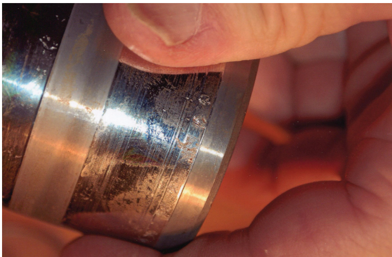
COLOR FIGURE 5.6 Spalling of a hardened steel rolling surface for cam followers.
