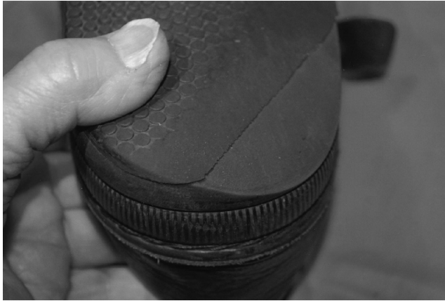
FIGURE 6.10 (See color insert.) Impact wear on an elastomer shoe heel.
