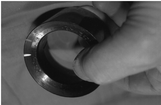
FIGURE 6.2 Impact wear on a valve seat from a hard steel ball contacting twice a minute for thousands of hours.
