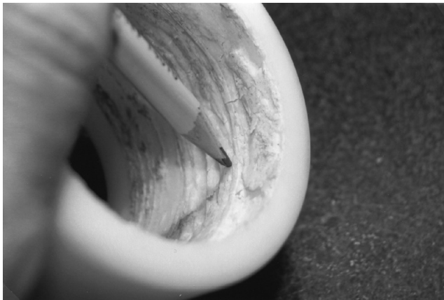
FIGURE 3.20 (See color insert.) Bore of a plastic bushing after a temperature-induced seizure.
