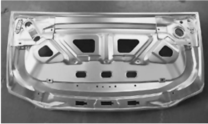
Figure 1.10 FSW to join the aluminum deck lid to galvanized steel brackets by Mazda (Mishra and Mahoney, 2007).
