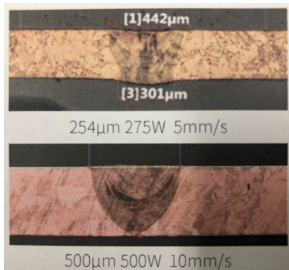
Fig. 3.22 Cross sections of blue laser weld beads produced in Cu sheets at 275 W and 5 mm/s and 500 W and 10 mm/s
