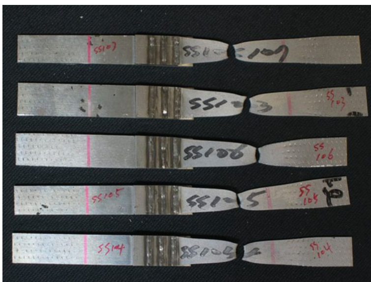
Fig. 9.6 Tensile shear test samples of three laser lap weld beads made under proper conditions, showing fracture in SPCC base specimen
