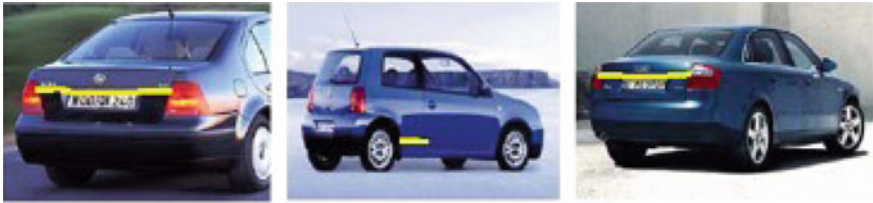
(a) Application examples of laser brazing to trunk lid, etc.
