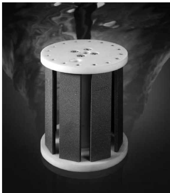
FIG. 2 Photo of Rotating Cage Containing Coupons
