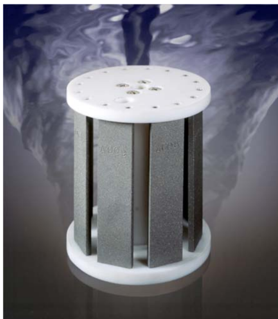
FIG. 2 Photo of Rotating Cage Containing Coupons
