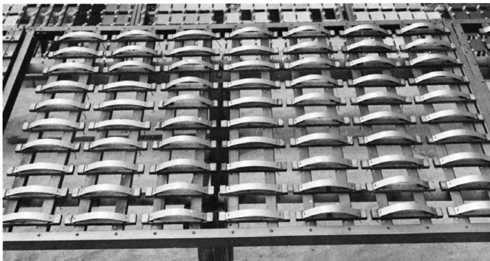
FIG. 4 Bent-Beam Specimens on Atmospheric Exposure Rack
