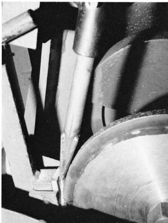
FIG. 8 Position of Sand Nozzle
