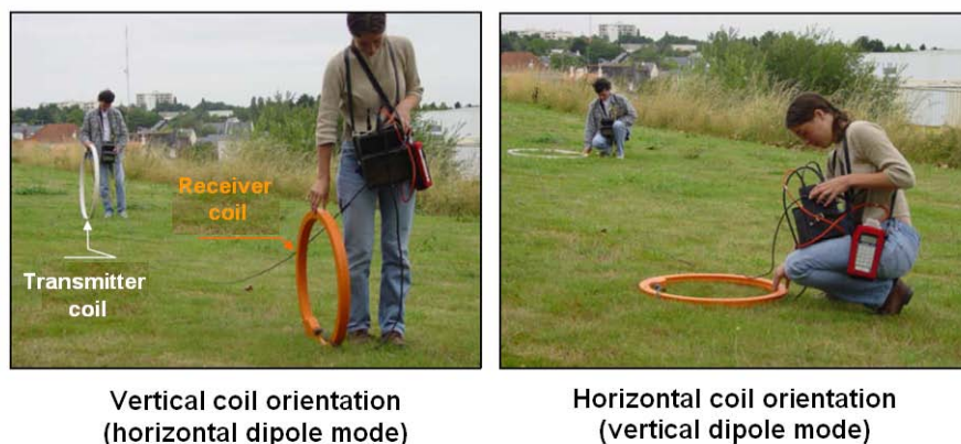
Figure 1 - Equipment in operation with 10-m spacing
