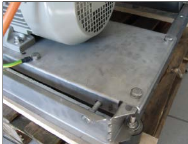
Picture 4 - Principle of omega sliding shape
