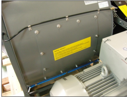
Picture 9 – Fixation of plastic tubing (in blue) and connector, outside the FAN casing
