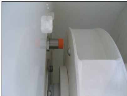
Pictures 11 and 12 - Principle of direct drive FAN proximity sensor – Front and back views
