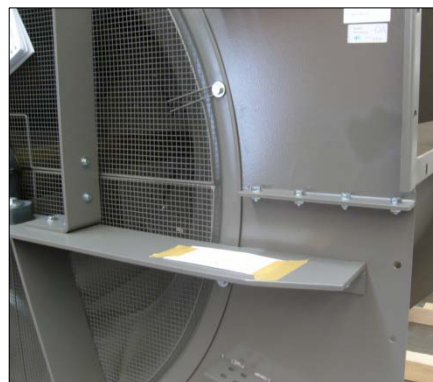
Pictures 1 and 2 - Principle of FAN casing which can be dismantled ( FAN casing in several parts with flanges)
