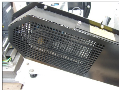
Picture 3 – Principle of access to the belts by dismantling of the upper part of the belt guarding
