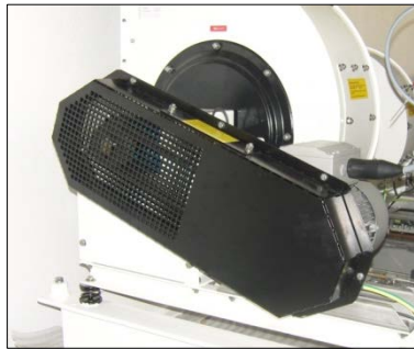
Picture 19 - Principle of FAN UNIT equipped with a belt guard
