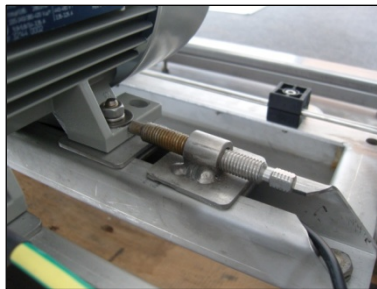
Picture 5 - Principle of screws adjustment
