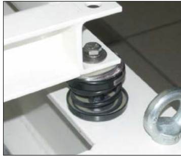
Picture 15: Principle of anti-vibration mounting
