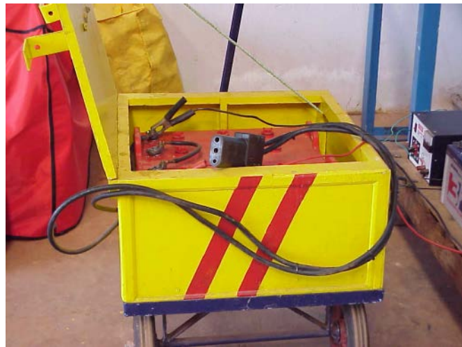
Trolley model equipped with lead batteries
