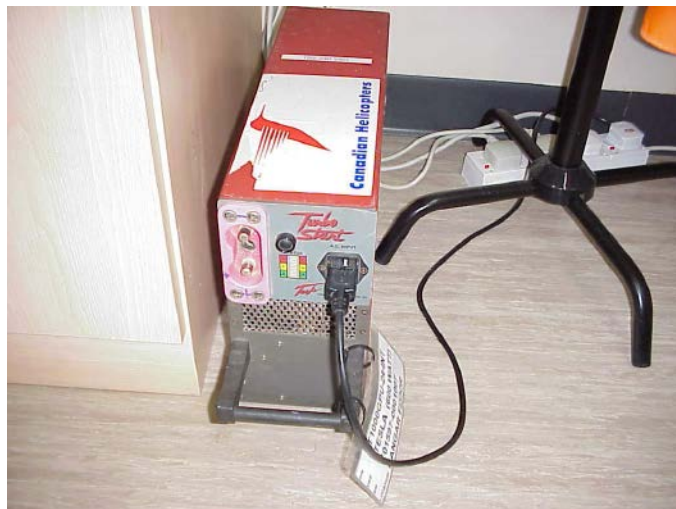
Trolley model equipped with lead batteries
