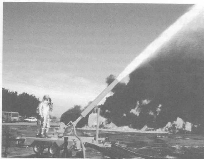
Figure 7.40 A foam cannon in operation - 15,000 litre/min of foam solution Courtesy of Angus Fire
