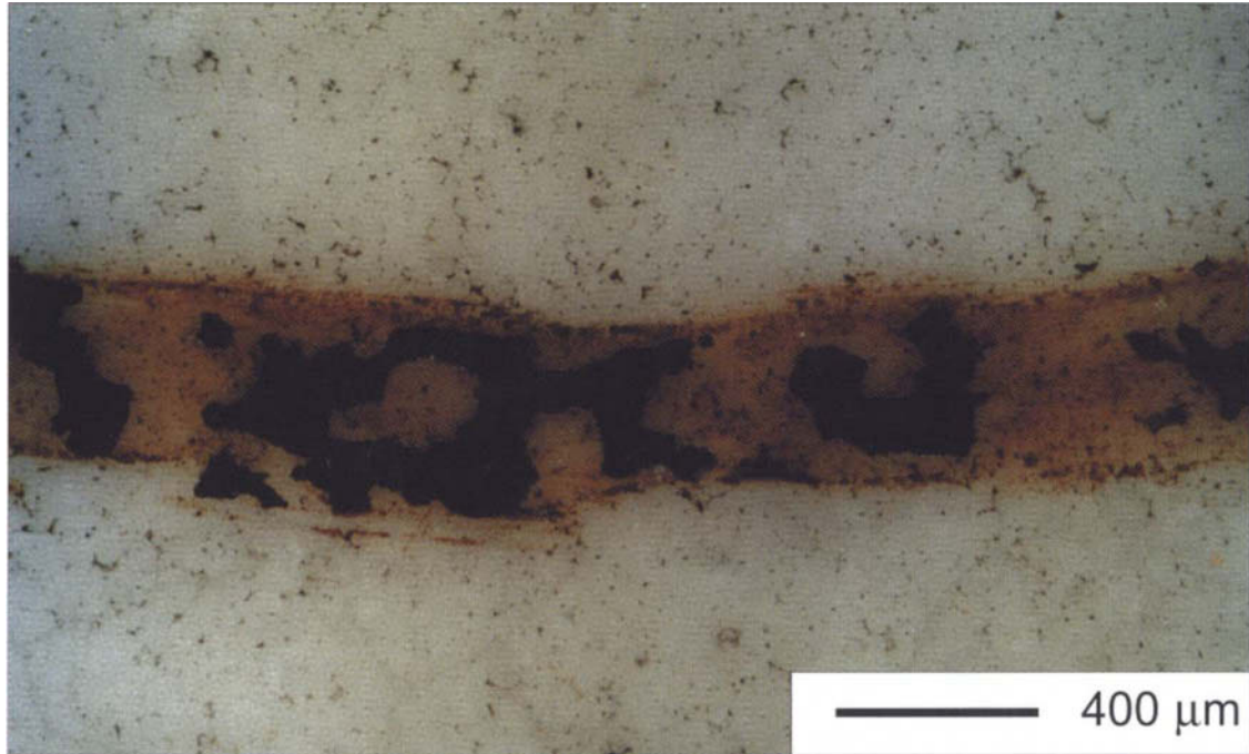
(a) Imaged with near-crossed polarizer illumination and emphasizing the iron oxide reaction layers on the surface of the wear track
