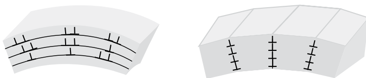
Figure 7.23: Mechanism of polygonization: (a) dislocations in a crystal after plastic bending, (b) formation of low-angle tilt boundaries separating the crystal in undeformed segments.
