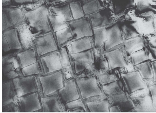
Figure 9.48: Micrograph from the transmission electron microscope showing \gamma' ( Ni_3Al ) particle dispersion in an FCC matrix in an Inconel 718 superalloy.
