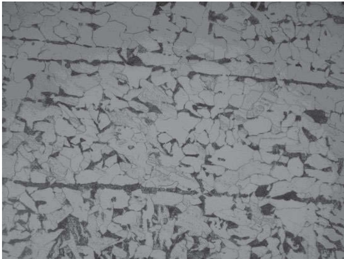
Figure 3.31: Microstructure of a carbon steel ( Fe - 0.4C ): Grain boundaries and interphase boundaries between ferrite (white) and pearlite (black).
