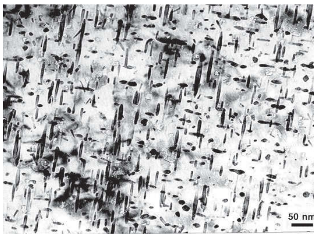
Figure 10.24: Secondary hardening in a steel containing molybdenum: (a) hardness curves, (b) TEM micrograph showing the fine Mo_2C carbide dispersion.
