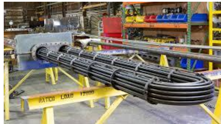
Bundle during fabrication
