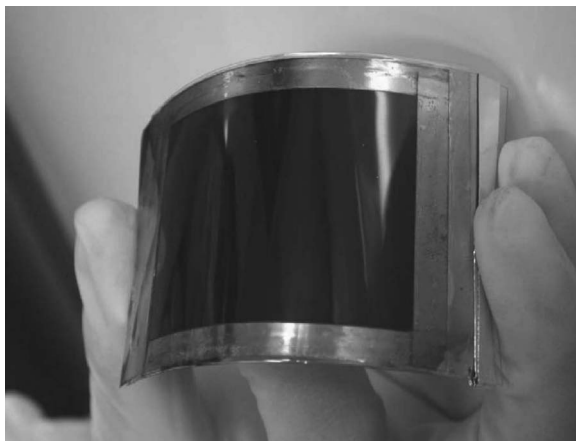
FIGURE 2.18 Lightweight flexible solid-state dye-sensitized solar cells: a stainless steel supported flexible cell with a conversion efficiency of 4.2%. (Reprinted from Kang, M.G. et al., Sol. Energy Mater. Sol. Cells , 90, 576, 2006. With permission.)
