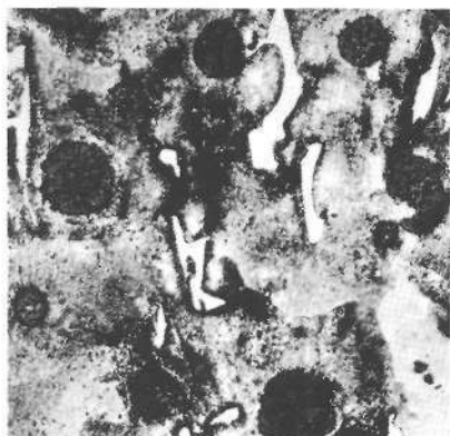
Fig. 4-25. As-cast ductile iron produced with 2.01% Si (Alloy WJA43, Table 4-3) showing carbide formation, nital etched, \times 250 .
