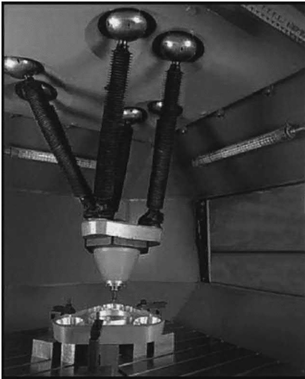
FIGURE 11.30 A typical hexapod machining application.
