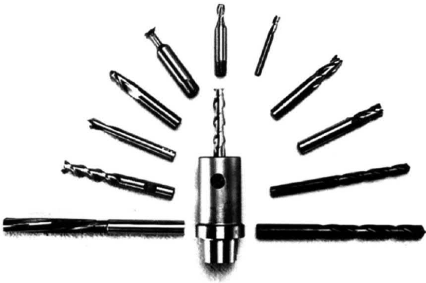
FIGURE 11.22 Tools accommodated by the spindle of a hexapod.
