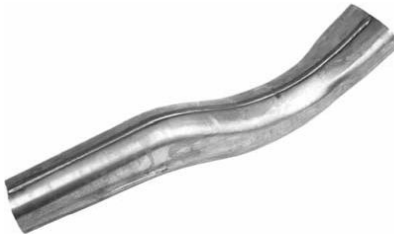
9.12 LaserTandem welding on a steel component, material thickness 4 mm, welding speed 3.5 \text{ m min}^{-1} .
