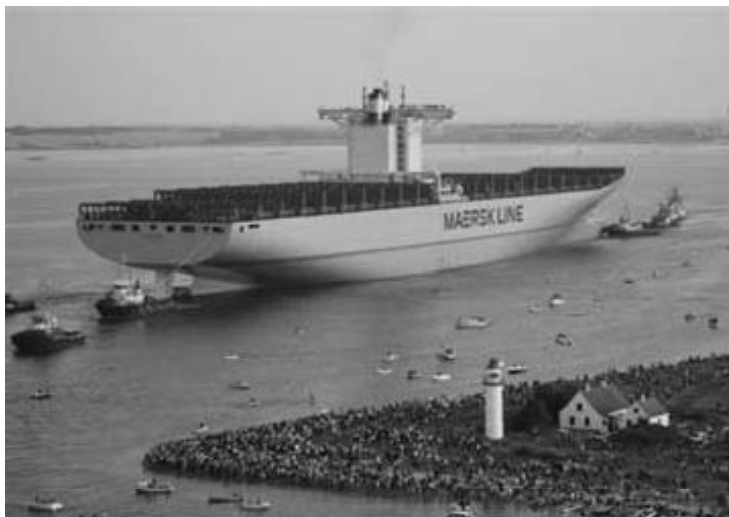
8.10 11000 twenty foot equivalent (TEU) container vessel at Odense Steel Shipyard. With 11000 TEU containers including 1000 forty foot equivalent (FEU) reefers. The ship is today (2008) the world's greatest container carrier and reefer vessel. 11 (Courtesy Odense Steel Shipyard).
