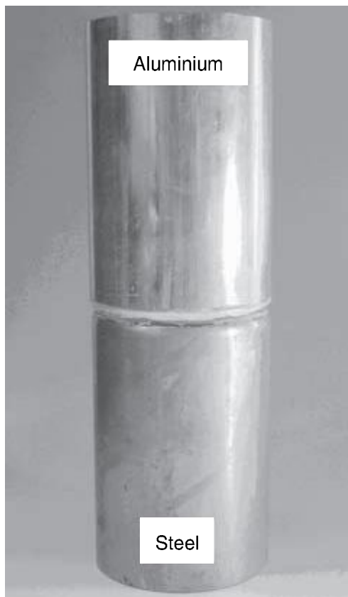
11.17 Aluminium–steel tailored hybrid tube joined by laser MIG hybrid welding.
