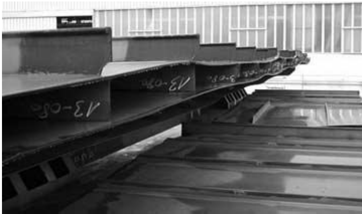
8.1 Typical arc welded deck panels for a passenger ship; note the distortions.
