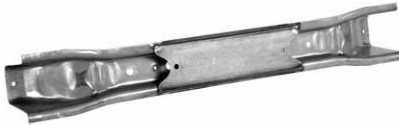
9.11 Case study: component from the automotive industry, welding speed 4.2 \text{ m min}^{-1} .
