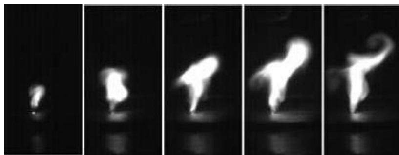
7.28 High-speed photographs of laser-induced plume/plasma of Mg alloy AZ31B during laser welding alone. 33
