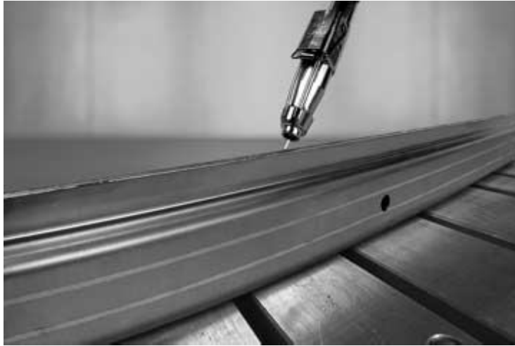
9.6 Application in the automotive industry: side panel in front of the driver's cabin.
