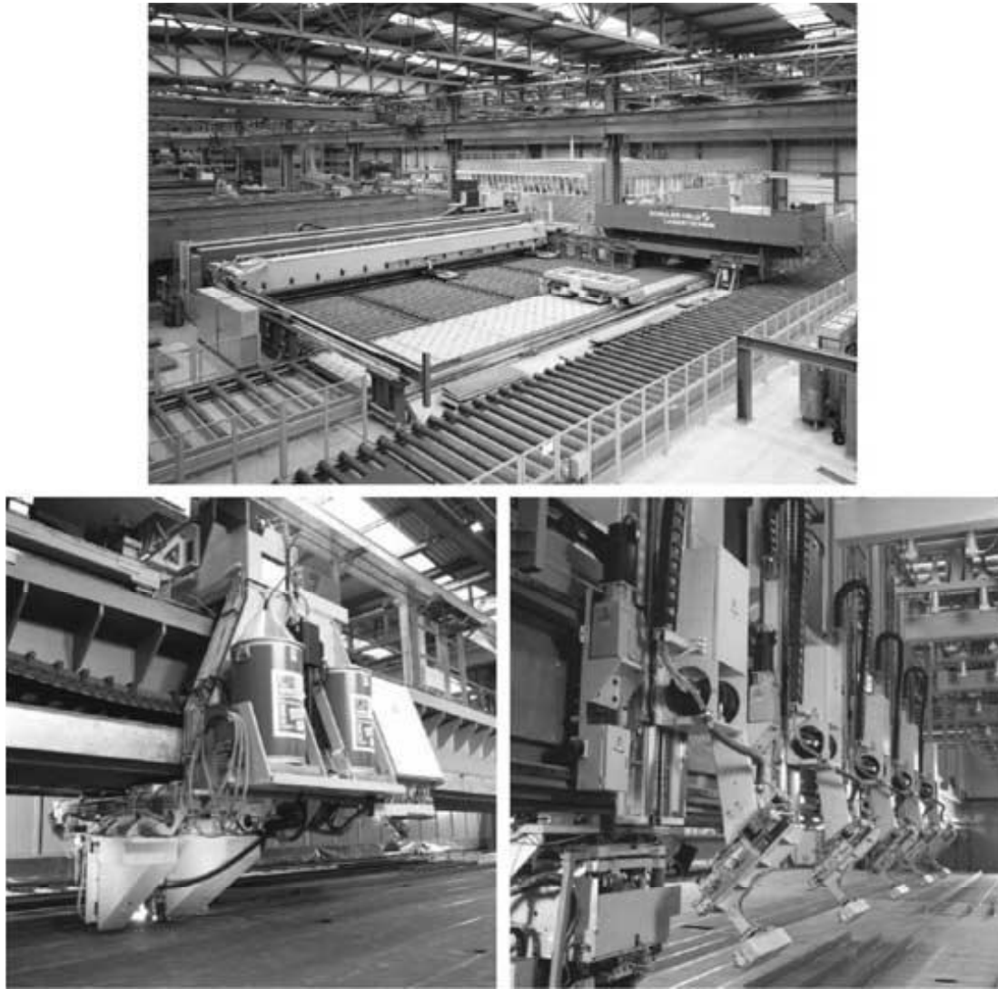
8.7 Photos of the installation as well as of a stiffener welding head and clamping tools (Courtesy: Guido Pethan, Meyer Werft).
