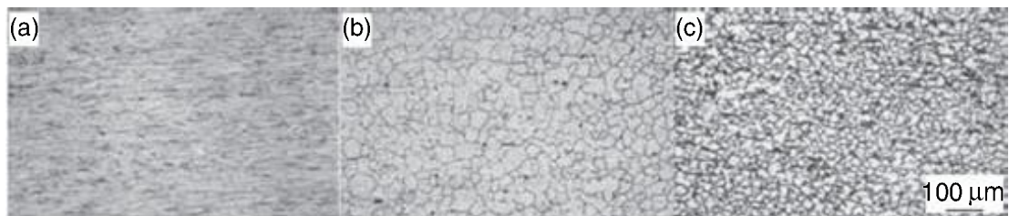
7.12 Microstructure of magnesium alloys 29 (a) AZ31; (b) AZ61; (c) AZ91.
