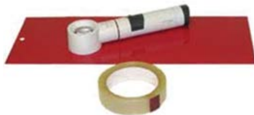
Fig. B.9: Transparent tape, magnifying light, and background for measuring surface contamination
