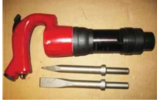
Fig. 8.3.b: Chipping hammer with chisel and point tools
