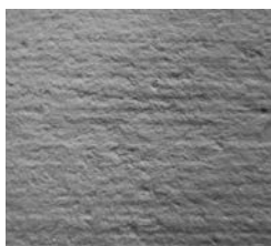
Fig. 6.4: CSP 4 (light scarification)
