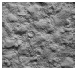
Fig. 6.7: CSP 7 (heavy abrasive blast)
