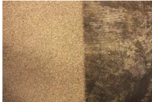
Fig. 8.12.c: CSP 3 surface using shotblasting
