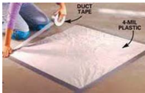
Fig. B.12.a: Moisture in concrete test using the plastic sheet method
