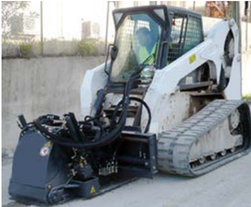
Fig. 8.8.a: Skid-steer-mounted rotomilling unit
