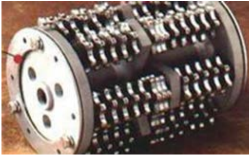
Fig. 8.11.a: Cutting drum with teeth
