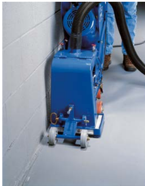
Fig. 8.12.d: 8 in. (203 mm) unit for trim work
