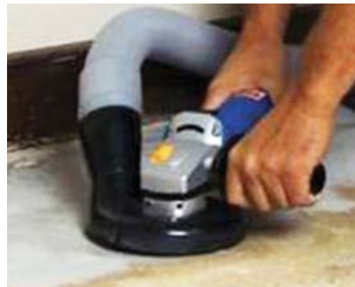
Fig. 8.5.d: Hand grinder for detail work
