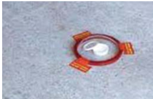
Fig. B.12.b: Moisture vapor emission test using the calcium chloride method
