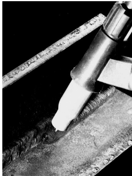
TIG dressing equipment and a partially dressed weld
