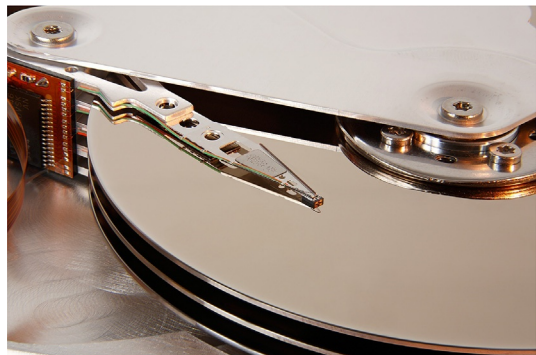
Fig. 9.33 Internal arrangement of a magnetic hard disk drive, showing a read/write head attached to the end of its support arm. The arm is moved across the surface of the disk so that the head can access circular tracks at various distances from the centre of the disk. Each surface of the three disks in this example has its own read/write head (Eric Gaba, Wikimedia Commons, CC-BY-SA-3.0)
