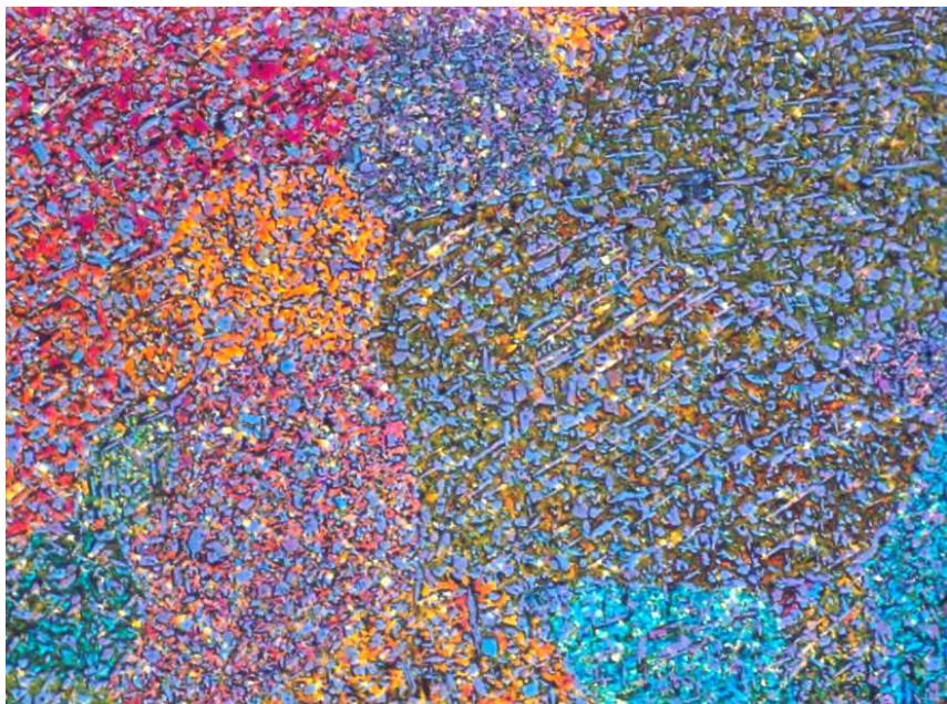
a) polyhedral microstructure, mag. 100 x
