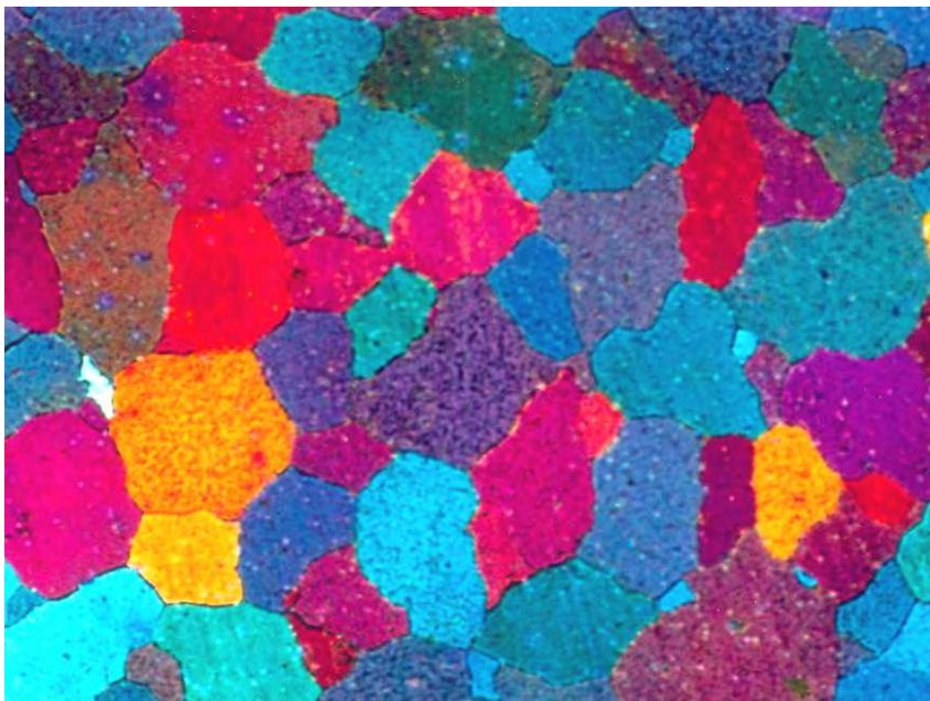
a) polyhedral grains of \beta' phase, polarized light, mag. 100 x
