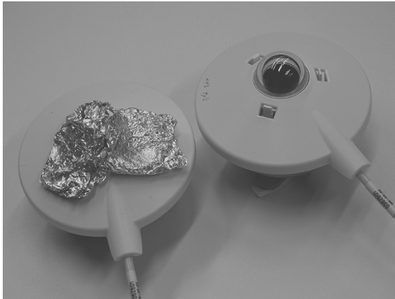
Figure 4.53 Measurement setup with CMP3 pyranometers. Measurements were recorded after reaching the thermal equilibrium with the environment. The shielded sensor served as control sensor. The same procedure was performed for the CMP11-pyranometers.
