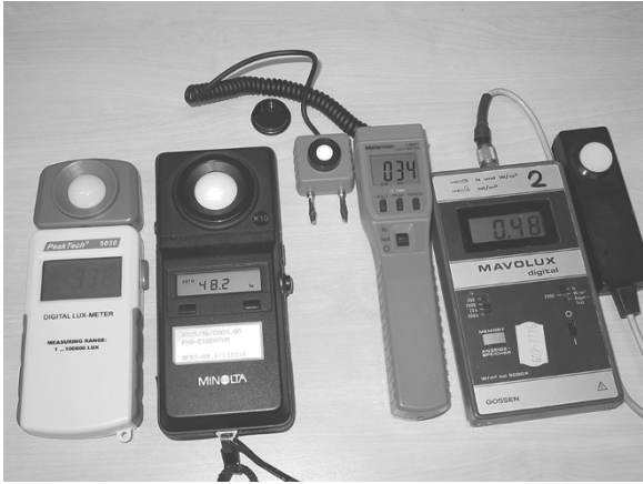
Figure 4.3 Displayed results for different luxmeter products with uncertainties from 2% to 4% under CIE standard lighting source A . For the fluorescent light of this measurement, the left luxmeter shows 332 Lux, the middle one 340 Lux.
