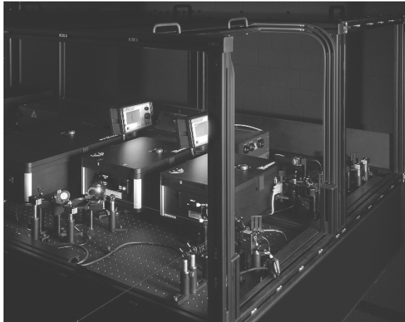
Figure 5.5 Photo of the complete laser setup with the beam routed through the SHG (400 nm). All beam paths are aligned to be coupled into the optical fiber (not shown here). During a measurement the laser setup is completely enclosed.
