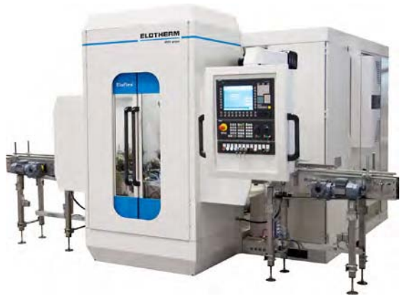
Figure 3.69: Interlinked and automatic hardening machine with one heating station (Source: SMS Elotherm)
