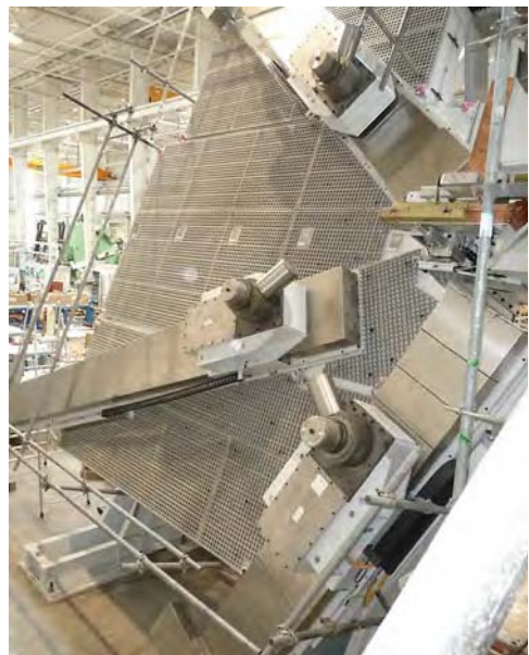
Figure 3.58: Induction hardening machine with pre-heater and 0-70° adjustable tilt table position (Source: SMS Elotherm)
