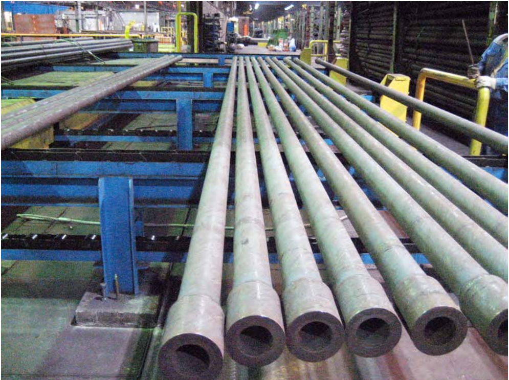
Figure 3.84: The result of the quenching & tempering process of tubes with upset ends
