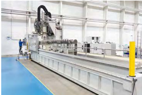
Figure 3.45: Induction hardening unit EloCrank™ XL for large crankshafts up to 10 meters (Source: SMS Elotherm)
