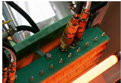
Figure 3.27: Heating using the single-shot hardening method (Source: SMS Elotherm)
