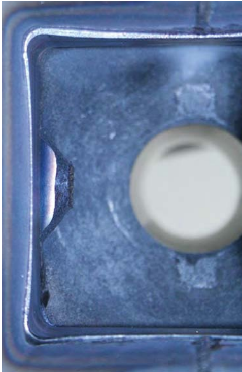
◀ Figure 4.50: IPS inner weld seam
