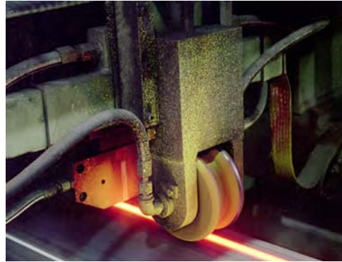
Figure 3.78: Tube seam annealing with pilot line for orbital correction of the inductor position (Source: SMS Elotherm)
