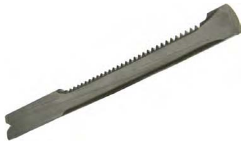
Figure 3.25: Section of induction-hardened teeth on a steering rack
