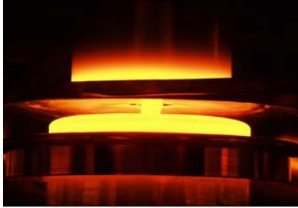
Figure 5.35: The melt zone in the FZ process
