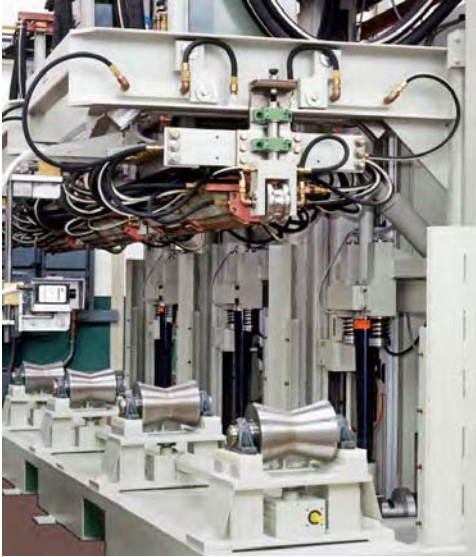
◀ Figure 3.77: Seam annealing for API tubes with NC-controlled positioning axis (Source: SMS Elotherm)
