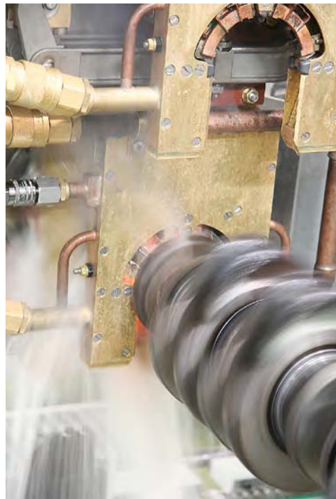
Figure 3.42: Quenching of a crankshaft (Source: SMS Elotherm)
