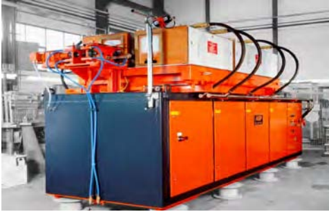
Figure 2.13: Induction heating plant in a forging line for billets (Source: ABP Induction)
