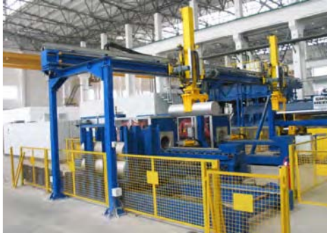
Figure 2.44: Two parallel single-billet induction furnaces with individually controllable heating sections, with a total capacity of 2x1,500 kW and billet dimensions of D 545 x 1,800 mm (Source: IAS GmbH)
