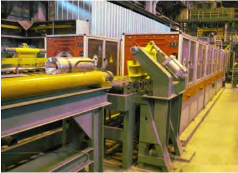
Figure 2.47 : Horizontal induction billet heating with an installed capacity of 2 x 3,600 kW (Source: IAS GmbH)
