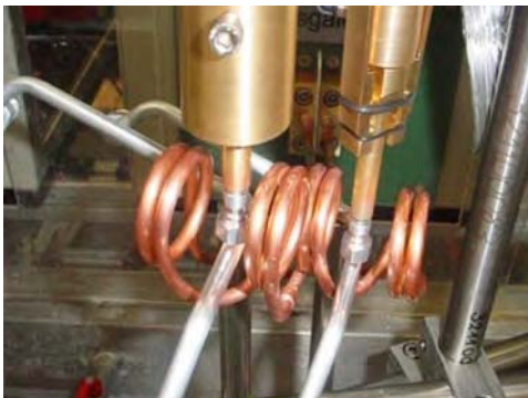
Figure 4.8: Inductive brazing with two frequencies of parts for automotive air-conditioning
