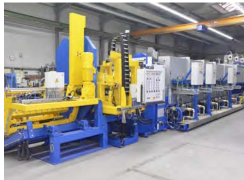
Figure 2.42: Inline furnace with downstream hot saw for 14" billet diameters (Source: IAS GmbH)
