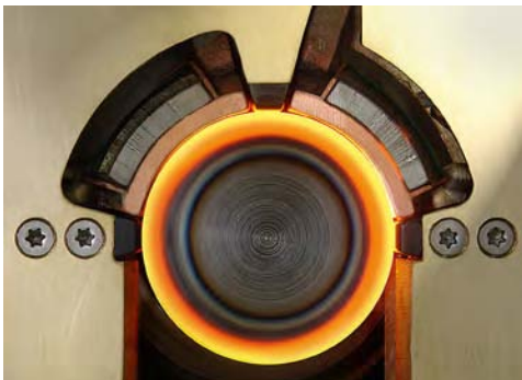
Figure 3.41: Inductor and cross-section of the crankshaft during heating procedure (Source: SMS Elotherm)
