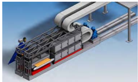
Figure 2.32: Example of a slab heating plant with separable inductors (Source: SMS Elotherm)
