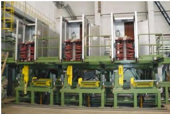
Figure 2.54: Vertical heating of titanium on a 3,500 t extrusion press line (Source: IAS GmbH)
