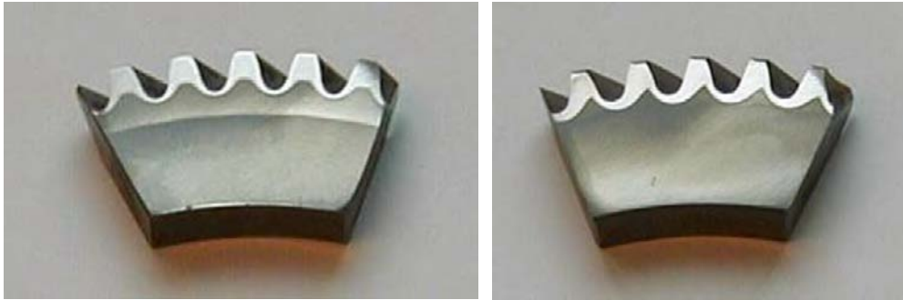
a) Symmetrical hardness profile at the centre of the gear
