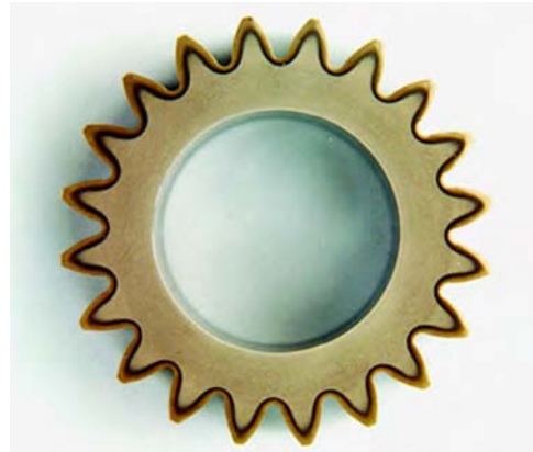
Figure 3.39: Micrograph of simultaneous dual frequency hardened gear
