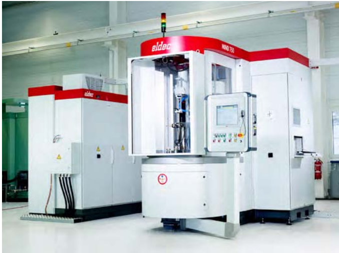
Figure 6.29: Hardening system with integrated 300 kW SDF® generator (on the left) (Source: eldec)
