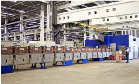
Figure 2.11: Bar heating plant upstream of a horizontal press (Source: SMS Elotherm)
