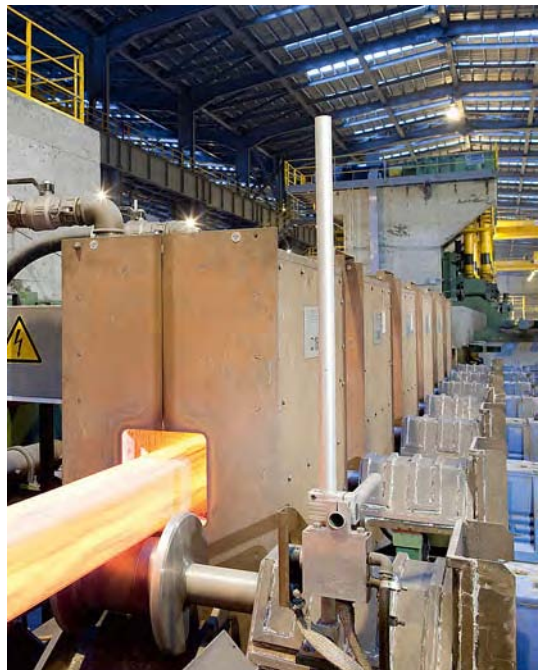
Figure 2.25: Billet before reheating in the induction heating at Tung Ho Steel in Taiwan (Source: SMS Elotherm)
