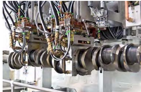
Figure 3.46: Assembly with four transformer-inductor units for parallel hardening of bearings (Source: SMS Elotherm)
