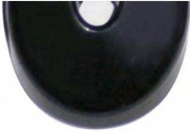
Figure 5.22: Grip of bottle opener, showing surface defects (Source: Kunststoffinstitut Lüdenscheld)
