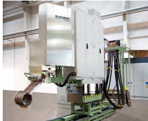
Figure 4.23: HFI welding facility for integration into the pipe shaping line (Source: SMS Elotherm)
