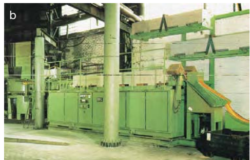
Figure 1.2: Induction heaters for forging a) Induction pusher type heater for ingots (Source: SMS Elotherm); b) Induction walking beam type heater (Source: ABP Induction Systems)
