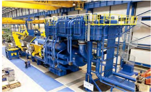
Figure 2.39: View of an extrusion press with a press force of 15,000 t (Source: SMS Meer GmbH, Mönchengladbach)
