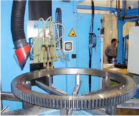
Figure 3.56: Induction hardening machine with horizontally positioned ring (Source: SMS Elotherm)
