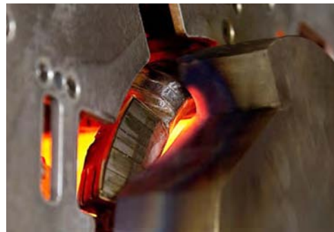
Figure 3.52b: Heating pattern of the undercut inductor (Source: SMS Elotherm)
