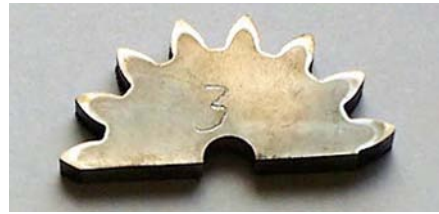
Figure 3.34: Micrograph of single frequency hardened gear
