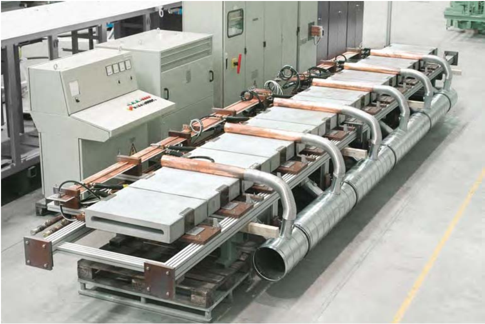
Figure 3.76: Typical heating system for varnish and lacquer drying (Source: SMS Elotherm)
