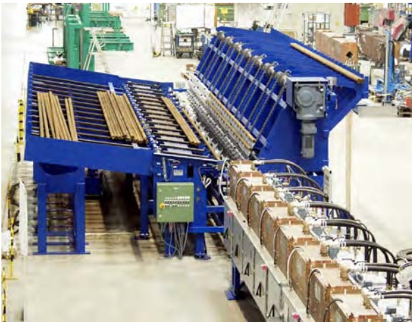
Figure 2.15: Induction bar heating line with bar magazine (Source: SMS Elotherm)
