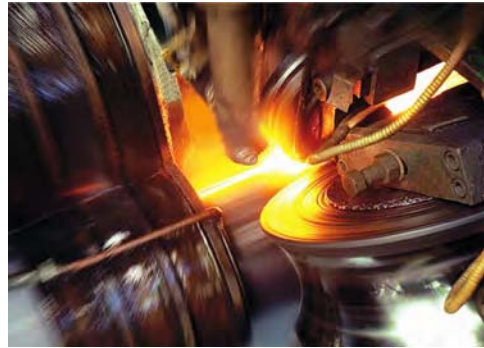
Figure 4.21: HFI welding process (Source: SMS Elotherm)
