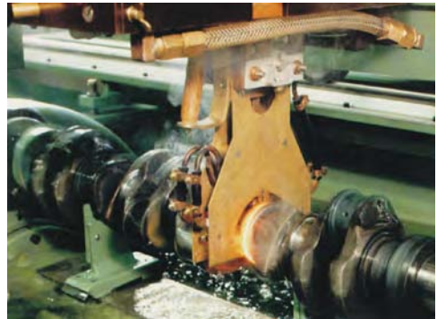
Figure 1.4: Hardening of crank shafts as typical example of surface hardening [1.2]
