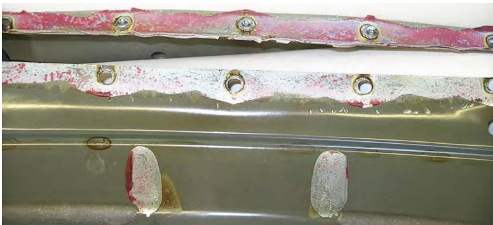
Figure 4.16: Separation of a structural bonding without adhesive pyrolysis
