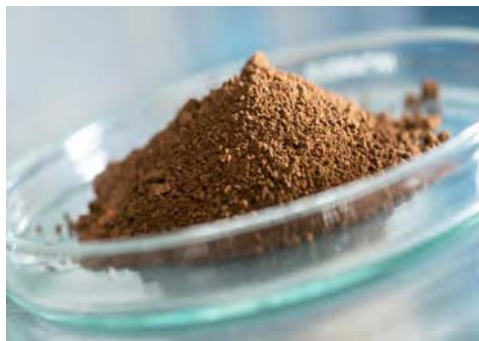
Figure 5.42: MAGSILICA®. These ferromagnetic nanostructured particles consist of various iron oxides (FeO) located in an insulating shell of SiO 2 . The particles are for this reason particularly chemically stable and have a low reactivity (image courtesy of Evonik Industries AG)
