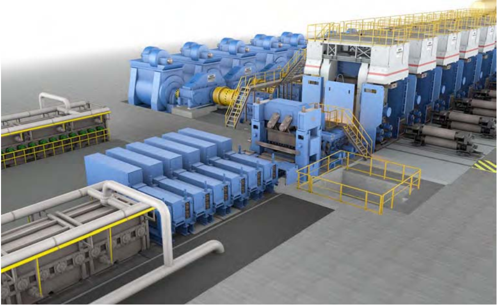
Figure 2.29: Example of an induction plant between the tunnel furnace and mill line for adapting the temperature level (Source: SMS Siemag AG)
