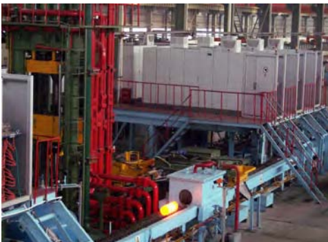
Figure 2.49: Intermediate heating for piercing press (used only in tube production) and vertical final heating (Source: IAS GmbH)
