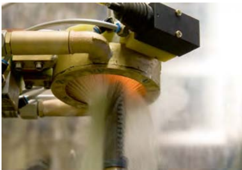
Figure 3.26: Scan-hardening of a vertically clamped rack (Source: SMS Elotherm)
