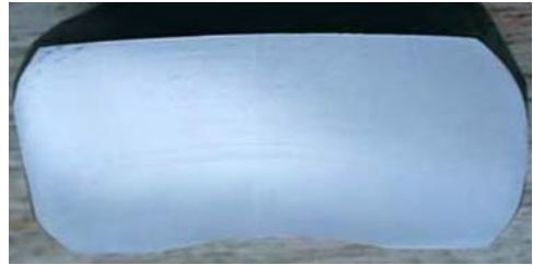
Figure 3.79: Weld on a longitudinally welded pipe with subsequent double-annealing (micro-section etched in order to show the ferrite line) (Source: SMS Elotherm)
