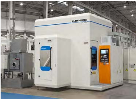
Figure 3.43: Flexible induction hardening unit for automotive crankshafts (Source: SMS Elotherm)
