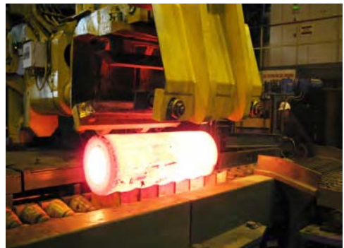
Figure 2.50: Heated billet of D 280 mm x 1,100 downstream of the piercing press, showing the temperature profile (Source: IAS GmbH)
