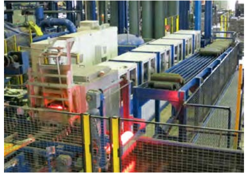
Figure 2.48: Horizontal induction heating plant with 6 individual zones with an installed capacity of 3,300 kW (Source: IAS GmbH)
