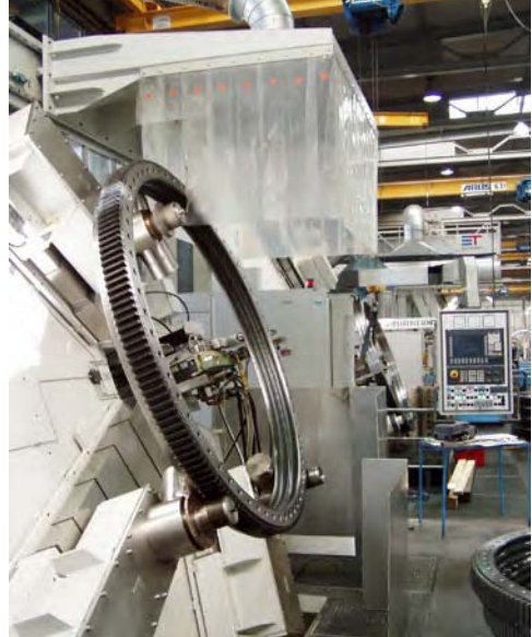
Figure 3.57: Induction hardening machine with 70° tilted ring in a fixed position (Source: SMS Elotherm)
