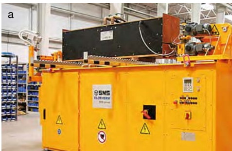
Figure 1.2: Induction heaters for forging a) Induction pusher type heater for ingots (Source: SMS Elotherm); b) Induction walking beam type heater (Source: ABP Induction Systems)
