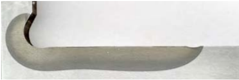
Figure 3.51a: Hardening zone with single-sided undercut (Source: SMS Elotherm)
