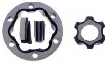
Figure 3.71: Hardening depths on sections of VL outer race (left) and inner race (right)
