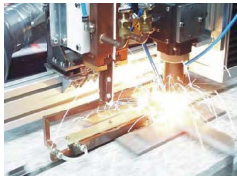
Figure 1.11: Combination of laser beam treatment supported by induction heating
