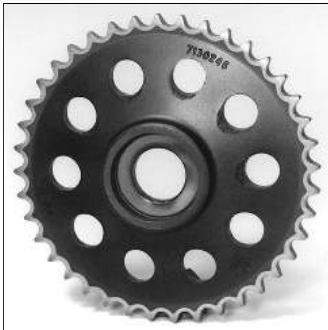
Fig.21. Holes in gears can cause unfavourable stress when induction hardening, resulting in cracks. Material selection and quench are important to reduce risk.
