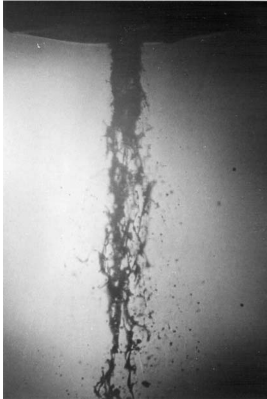
Figure 5.5 Mechanism of spray formation from a typical atomiser (Mullinger and Chigier 1974) (reproduced with kind permission of the Energy Institute)
