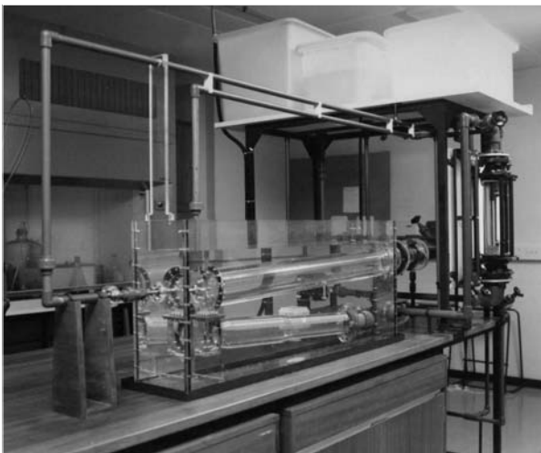
Figure 6.1 Physical modelling facility set-up for water modelling
