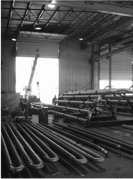
Figure 1.25 Heat transfer coils for refinery heaters showing a coil for a cabin heater (foreground) and cylindrical heater in the background (photo provided courtesy of Born Heaters, Canada, an Onquest company)
