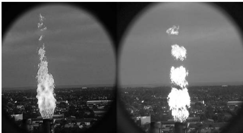
Figure 5.42 The Clyde Refinery flares in normal mode (left) and oscillation mode (right) (photos courtesy of Prof. G.J. Nathan and Mr A. Langham)
