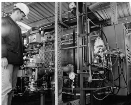
Figure 1.21 A small incinerator designed by the authors to recover energy from methanol contaminated water
