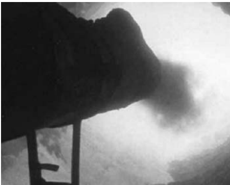
Note how the high secondary air velocity in the narrow kiln hood deflects the flame
