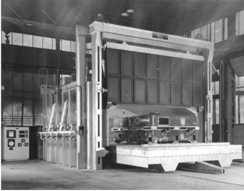
Figure 1.20 Two large gearbox cases entering a large annealing furnace (photo courtesy of John Mottershaw)
