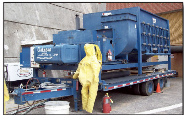
Air Handling Unit/Dust Collector
